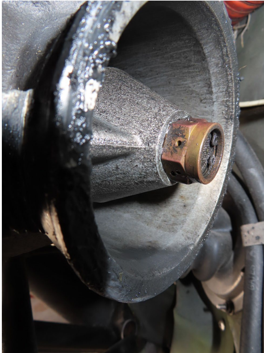
Photograph 8 - Fuel servo air inlet (Courtesy of Piper)
