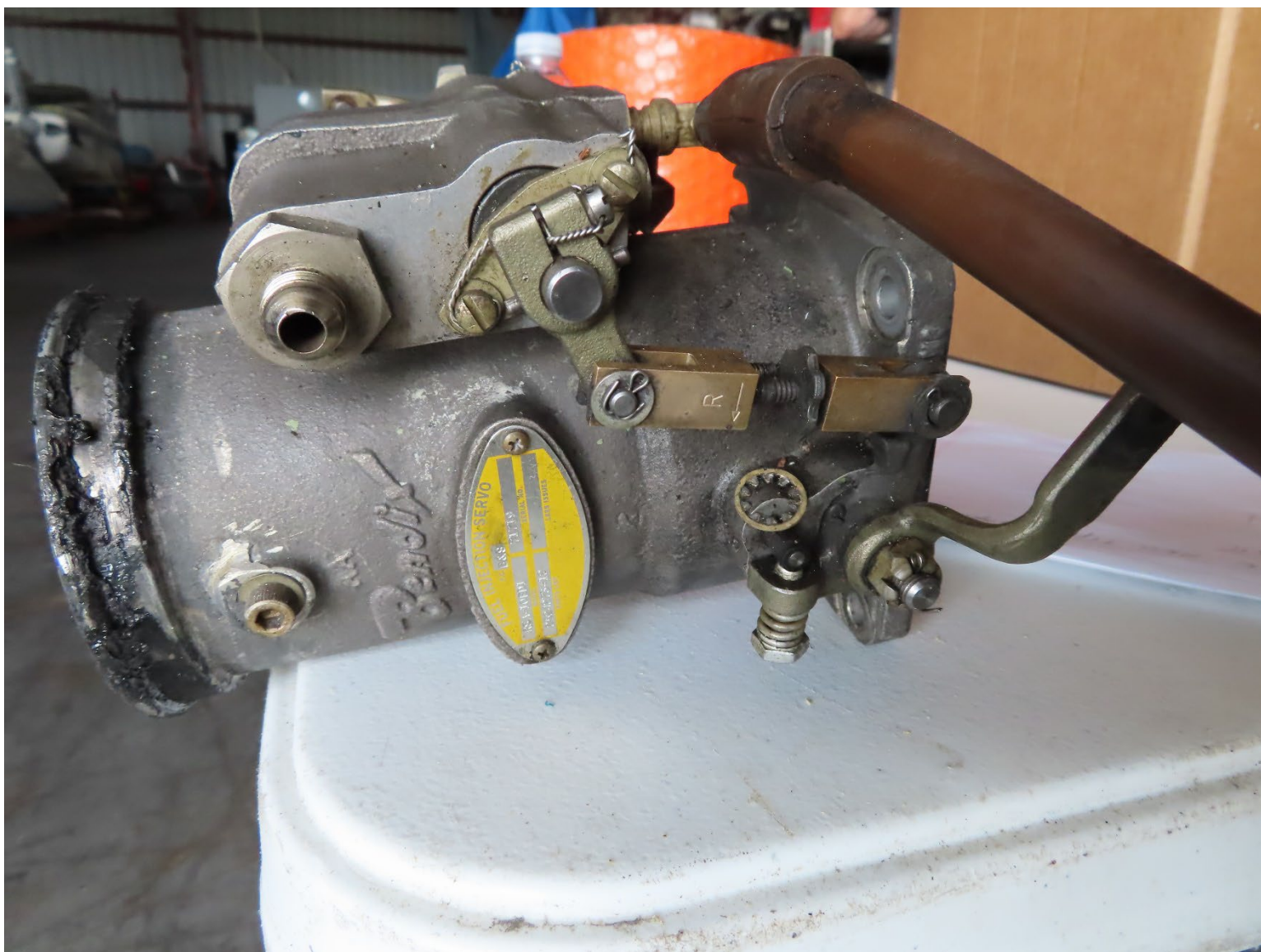
Photograph 10 - Fuel servo idle mixture linkage (Courtesy of Piper)
