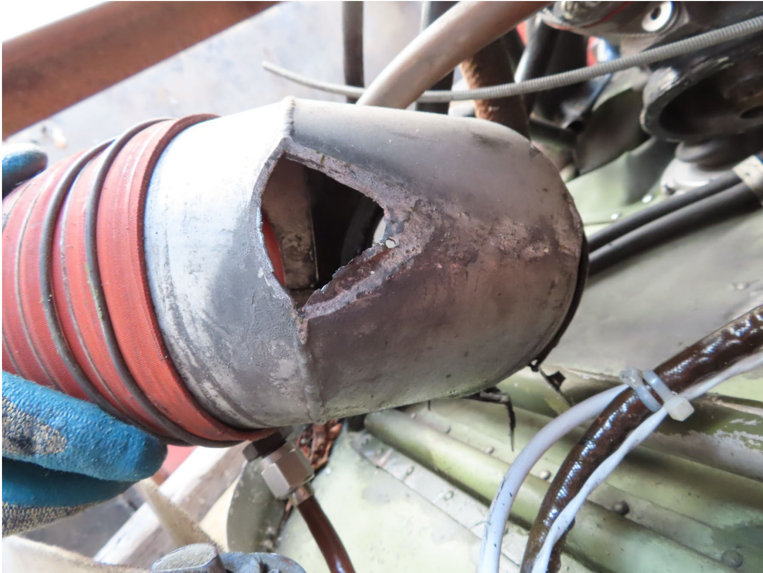
Photograph 6 - Fuel servo air inlet tube with hole (Courtesy of Piper)
