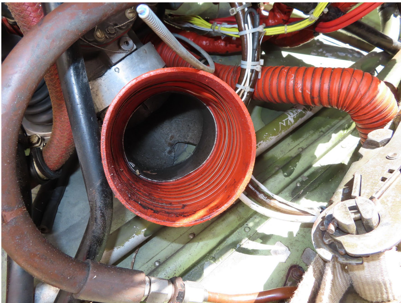
Photograph 5 - Fuel servo air inlet tube (Courtesy of Piper)
