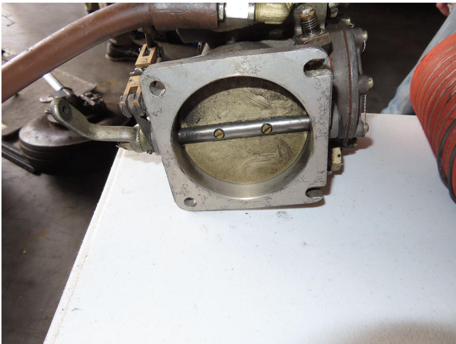
Photograph 11 - Fuel Servo Throttle Valve (Courtesy of Piper)
