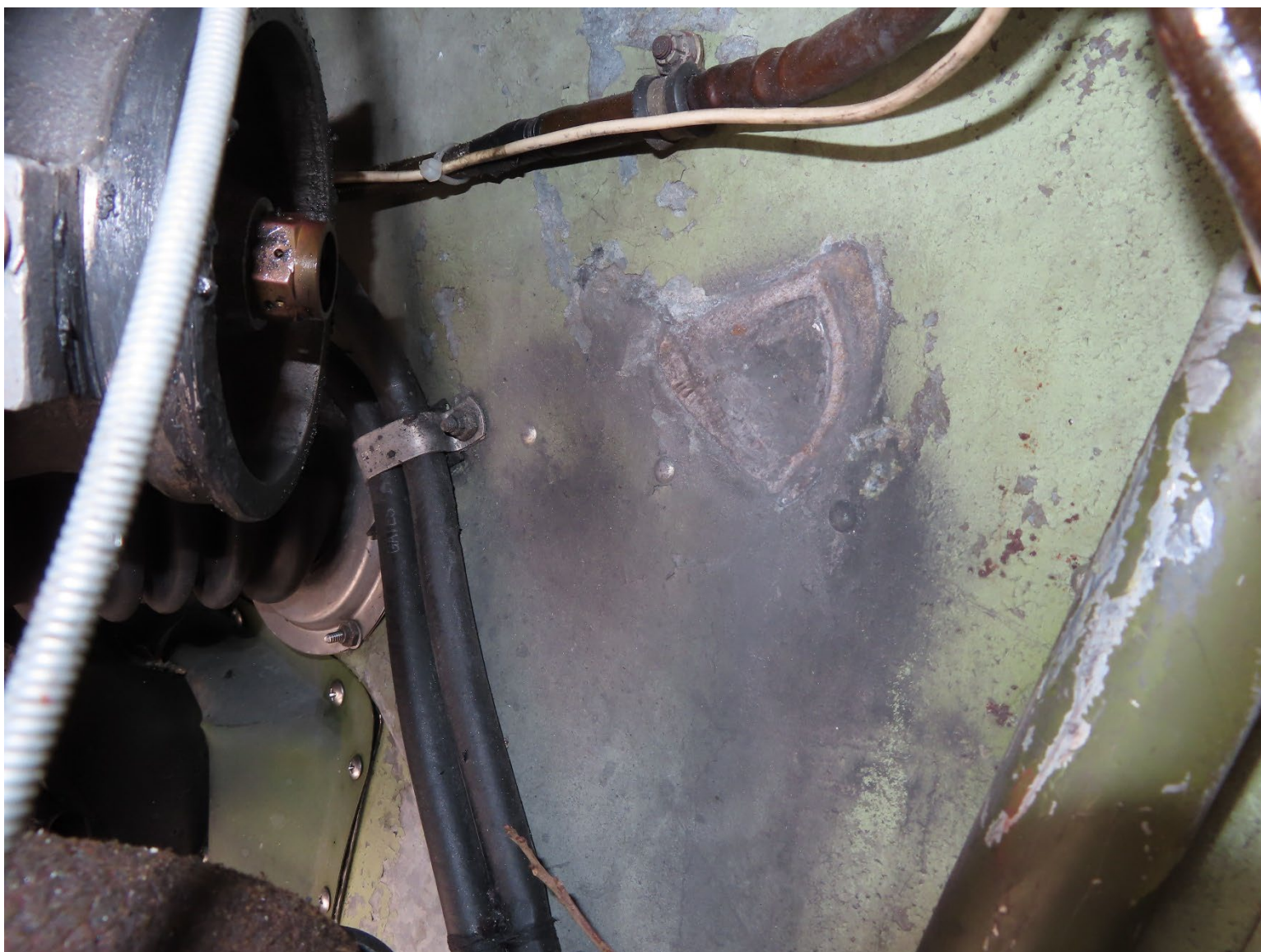
Photograph 7 - Firewall wear from induction tube (Courtesy of Piper)
