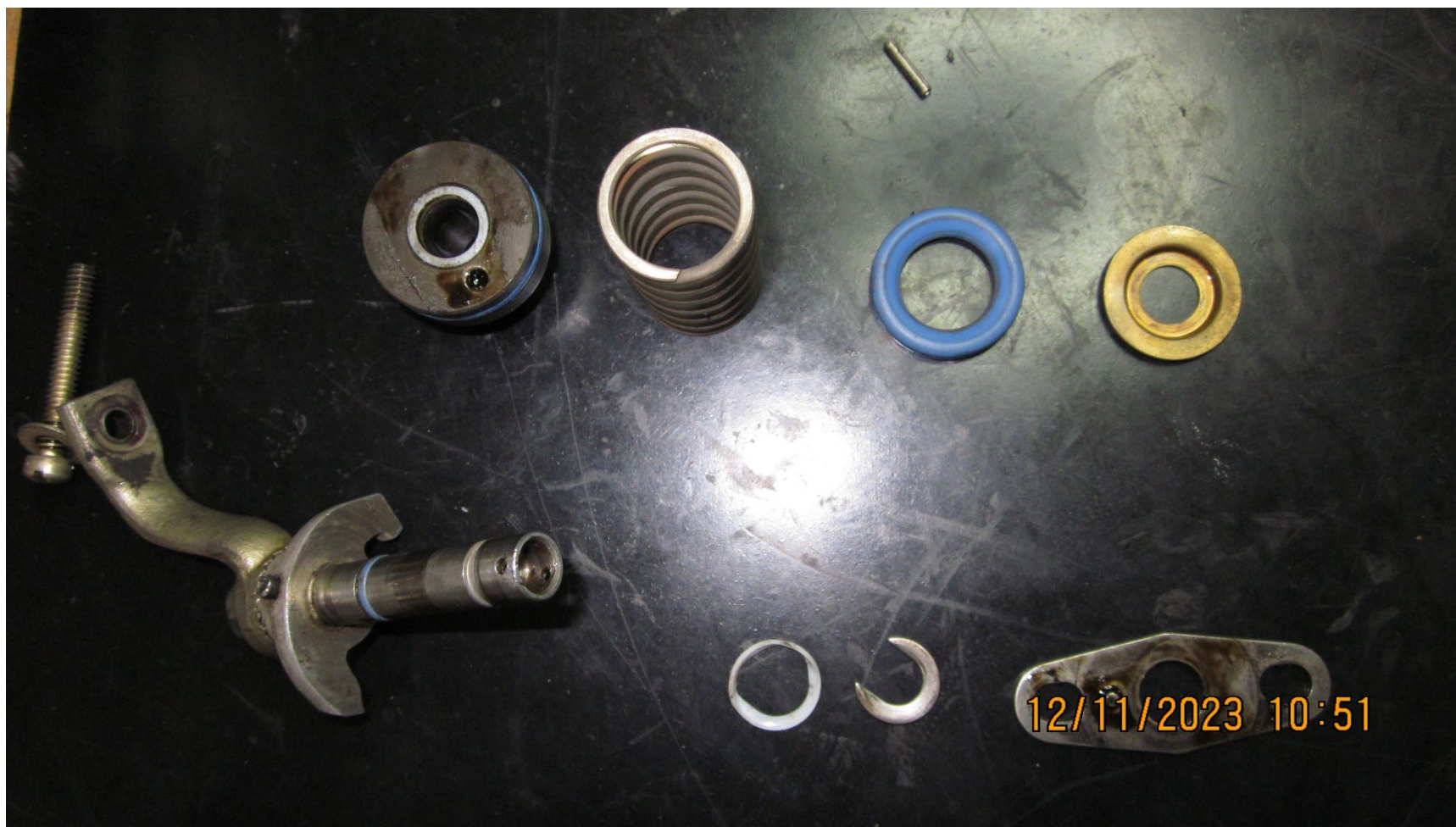
Photograph 8 - Mixture control components (Courtesy of FAA)
