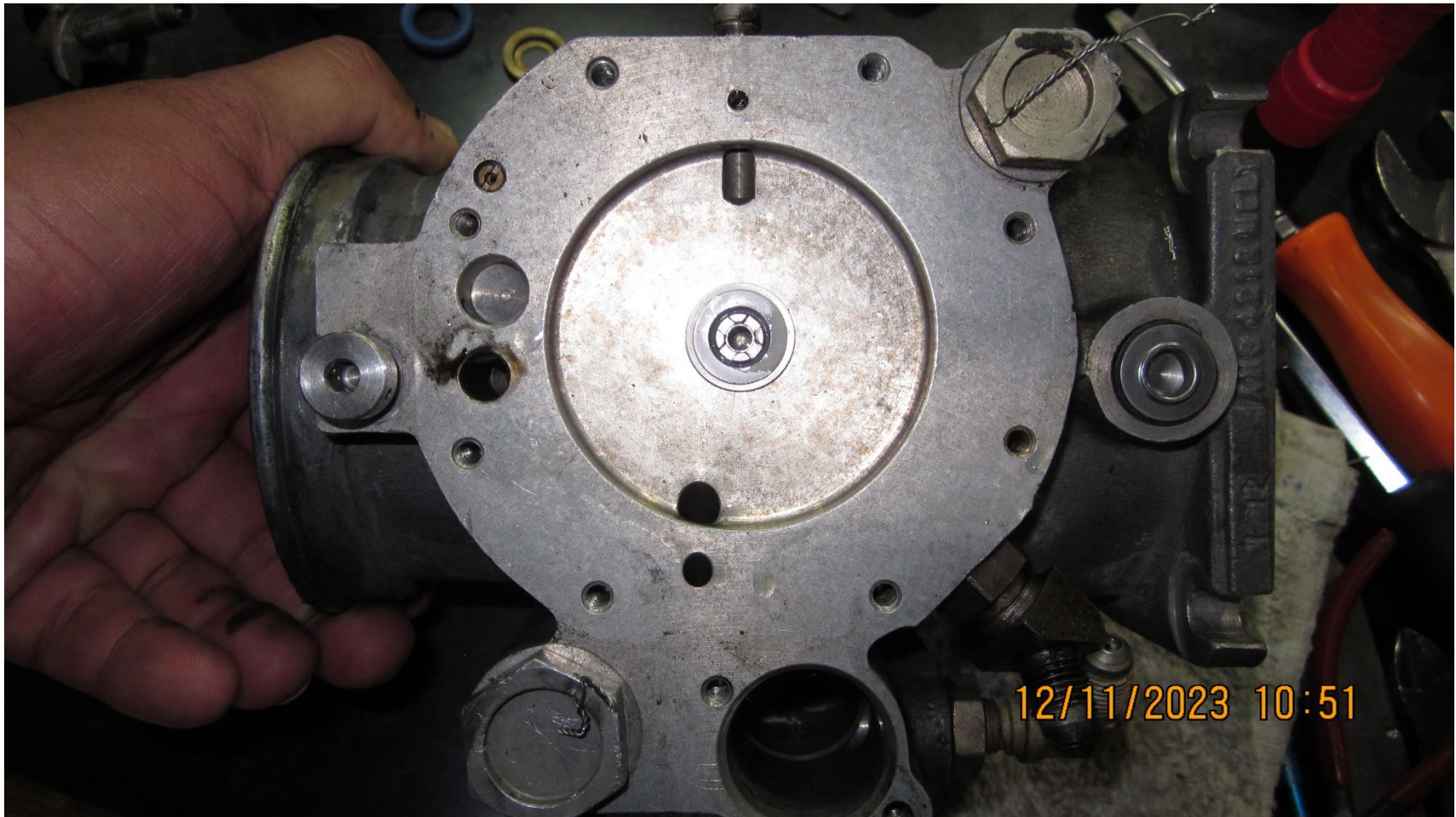
Photograph 7 - Fuel servo housing (Courtesy of FAA)
