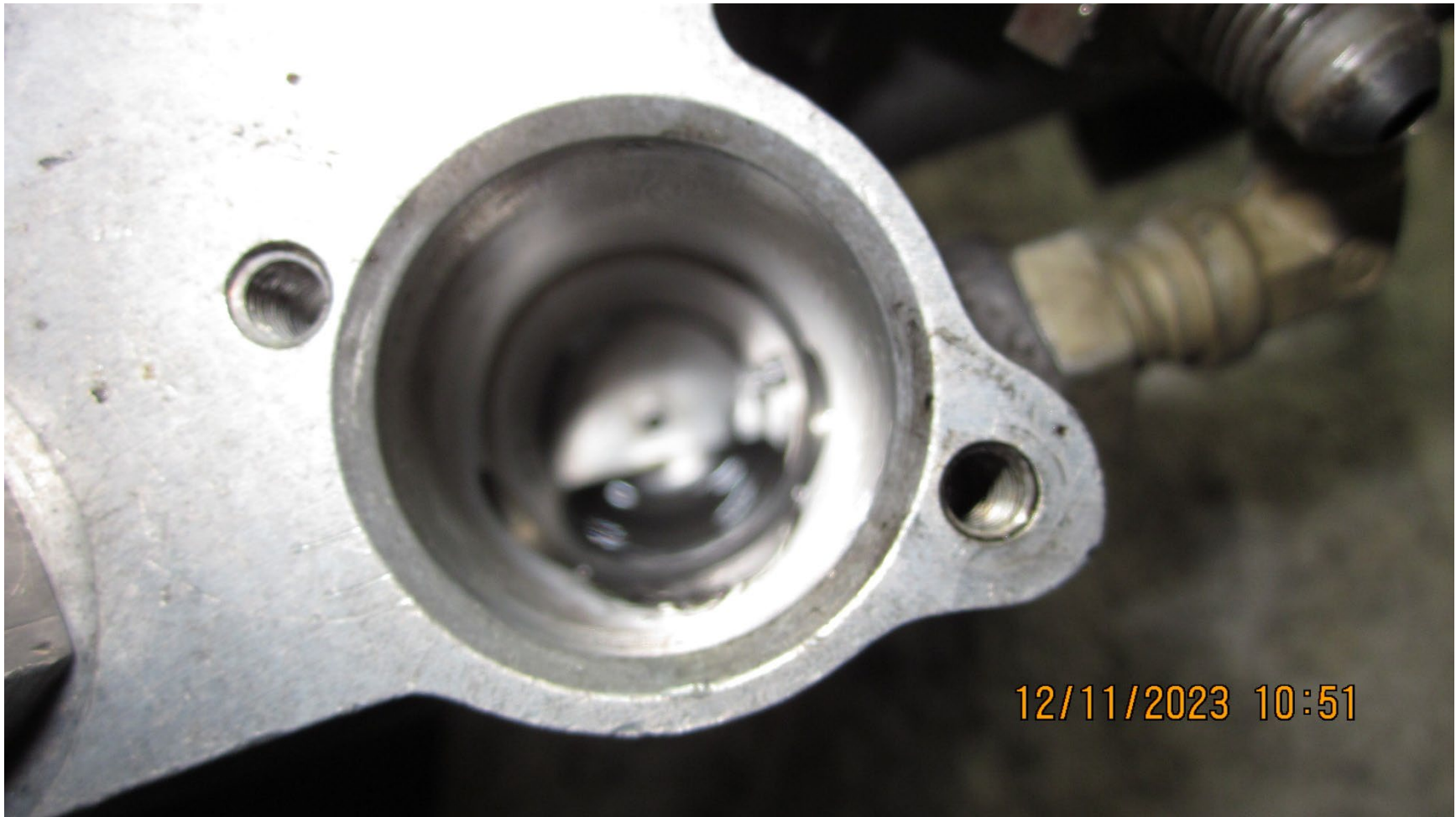
Photograph 9 - Mixture control housing (Courtesy of FAA)
