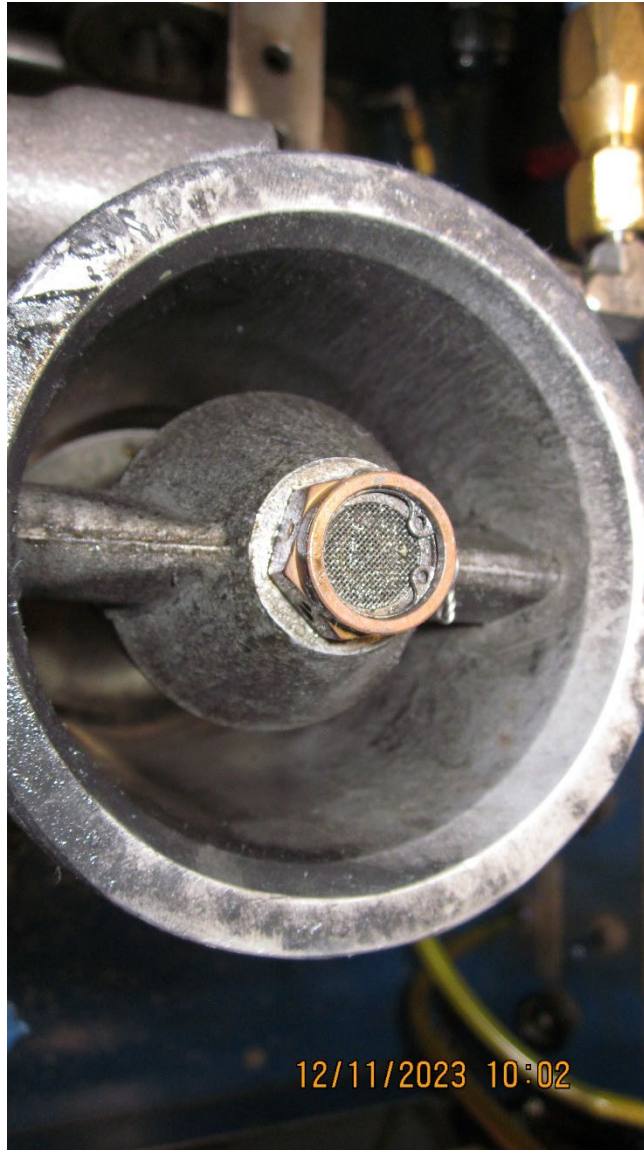
Photograph 2 - Air inlet with contamination (Courtesy of FAA)
