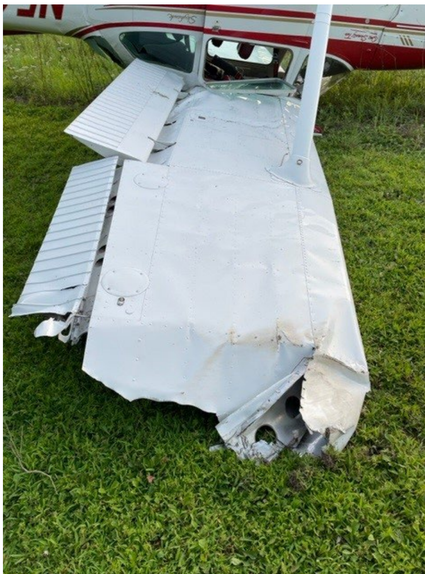
Photograph 3 - Left Wing Damage (Courtesy of FAA)
