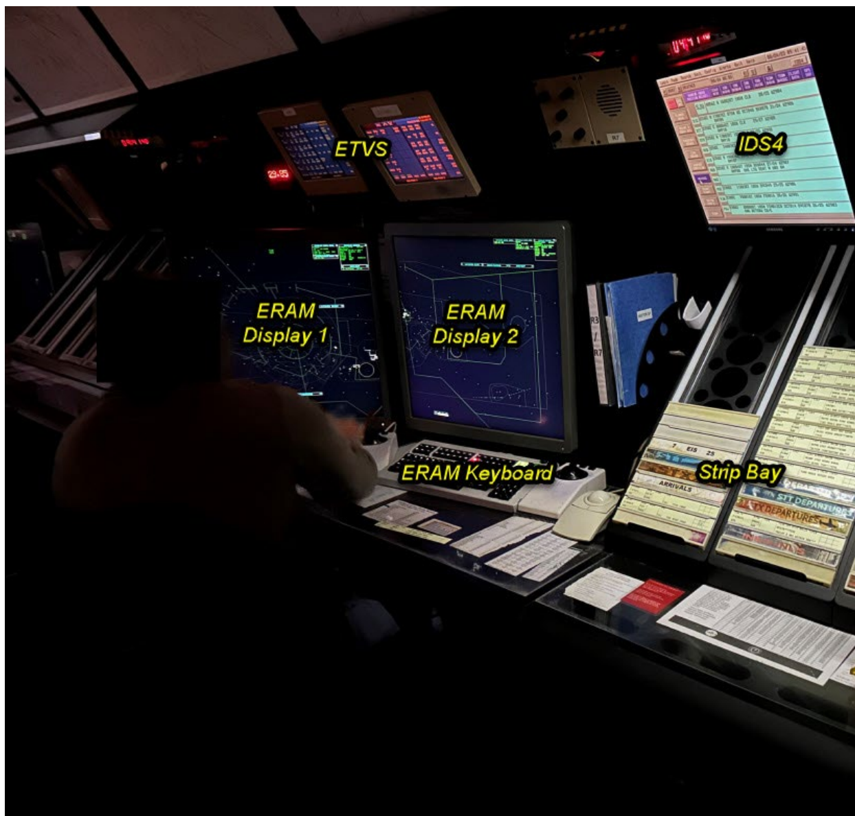
Figure 6. Photograph of the R7 position combined as it was at the time of the accident with pertinent information labeled.
