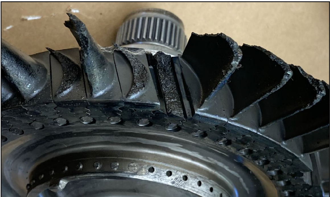
Photo No. 12, Power Turbine Blade Fractured Surfaces
