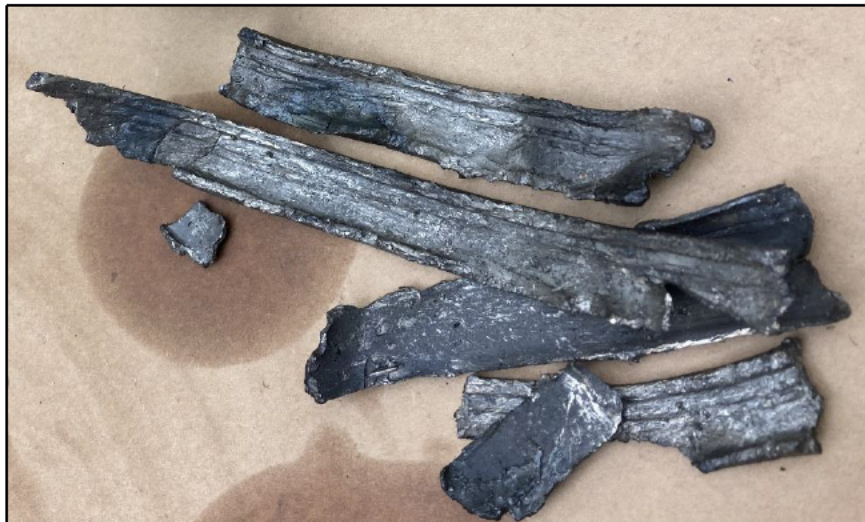
Photo No. 13, Power Turbine Shroud Ring
