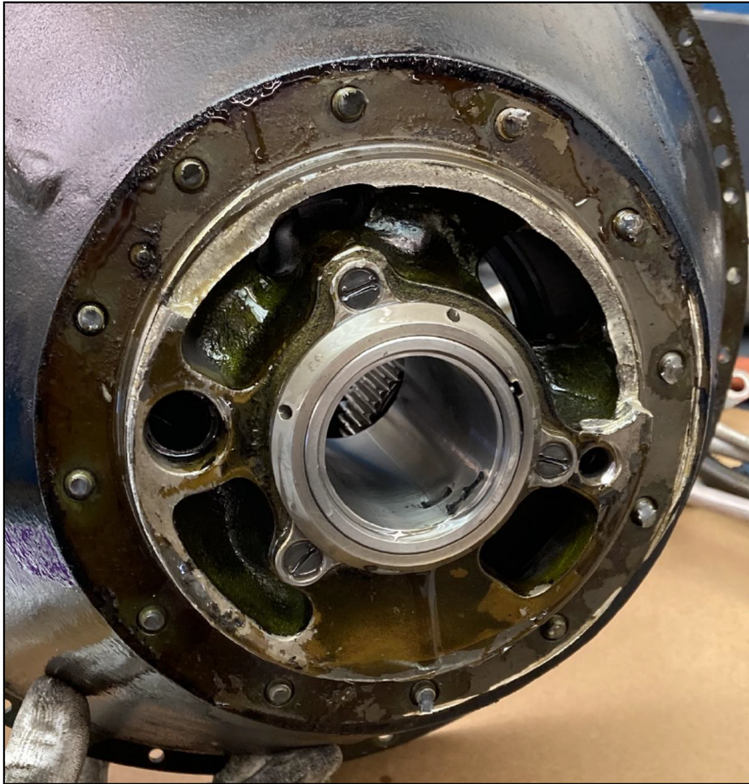
Photo No. 17, Reduction Gear Box Rear Housing
