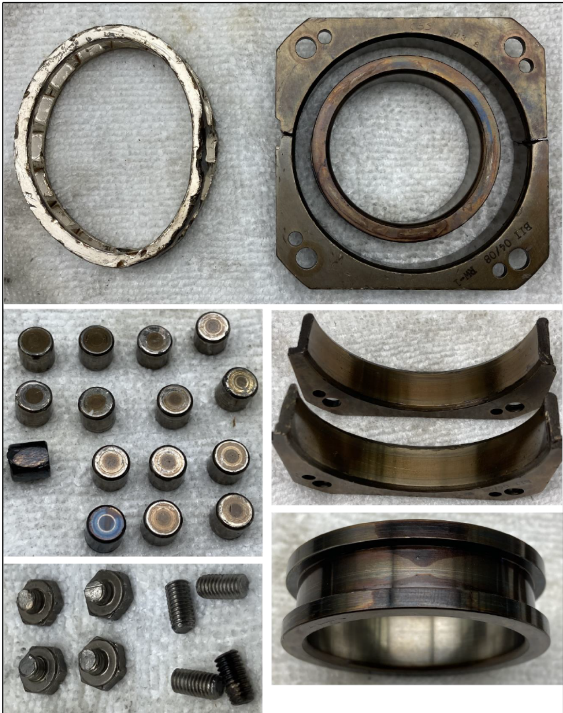
Photo No. 20, No. 3 Roller Bearing
