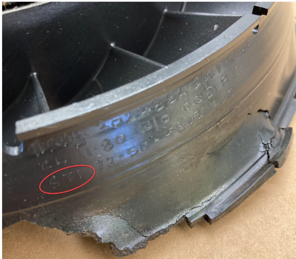
Photo No. 16, Power Turbine Vane Identification
