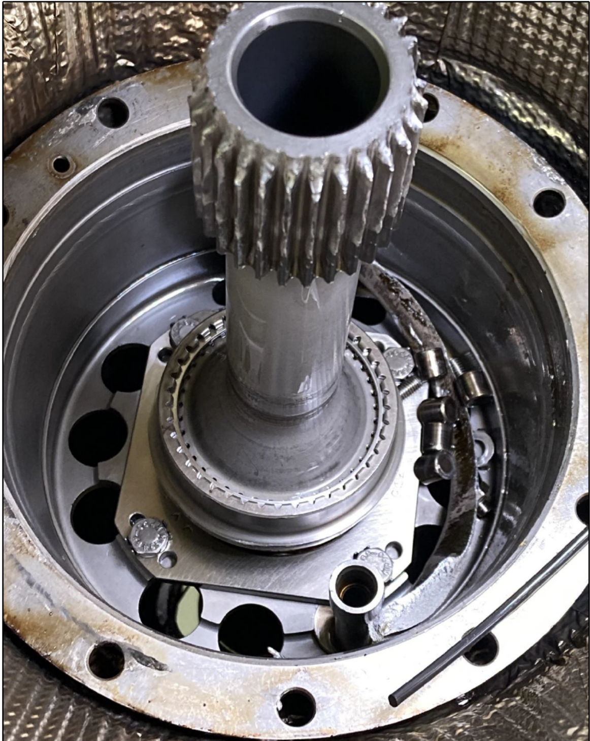
Photo No. 21, No. 3 Bearing Rollers Next to No. 4 Bearing
