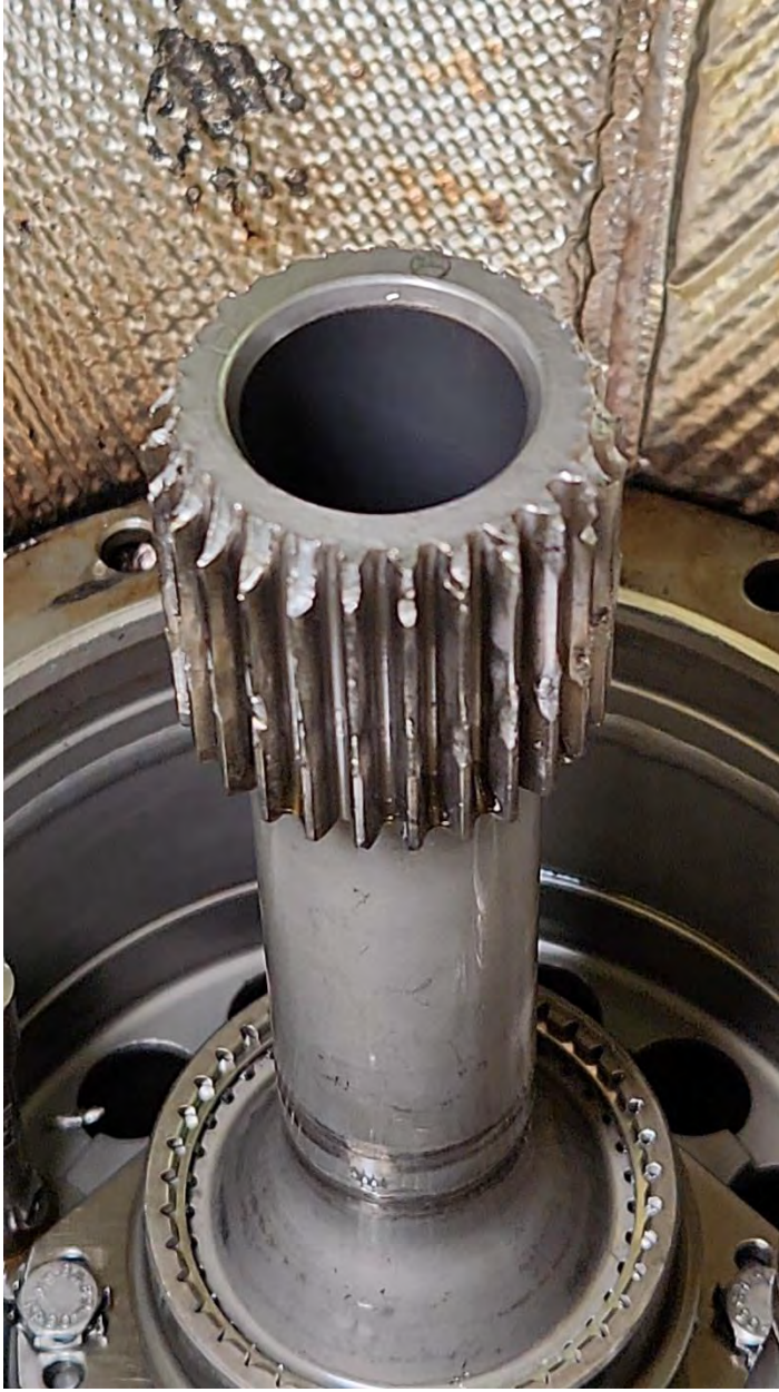
PT Shaft with damage
