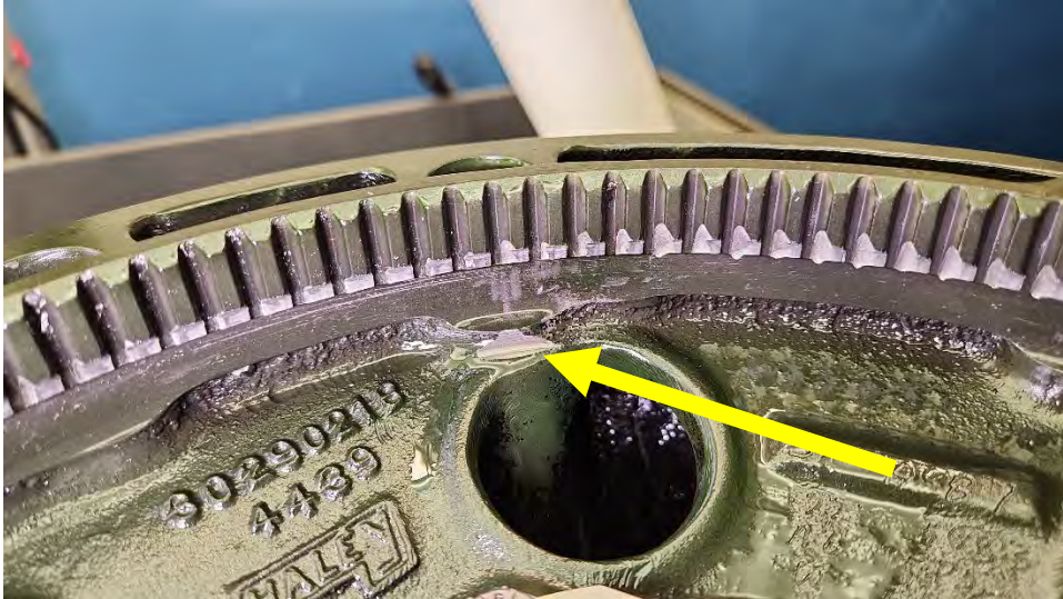
Bottom FWD RGB casing ring gear insert damaged
