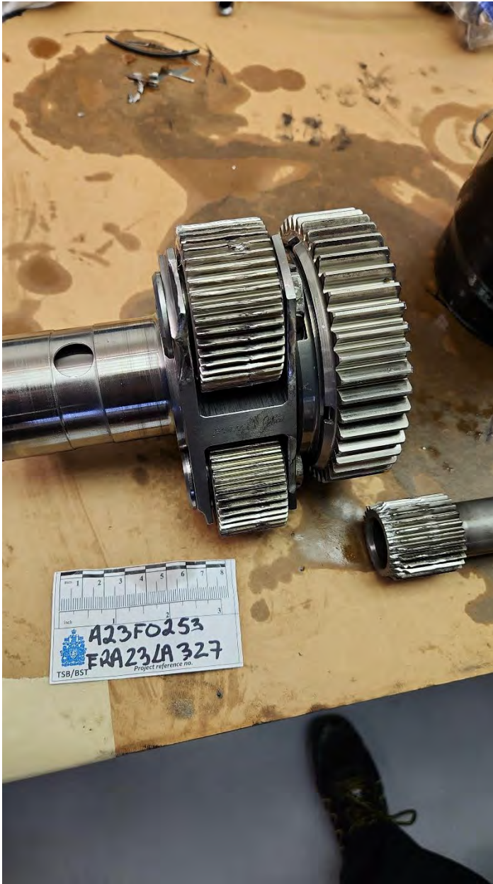
Damages found on first stage planetary gears
