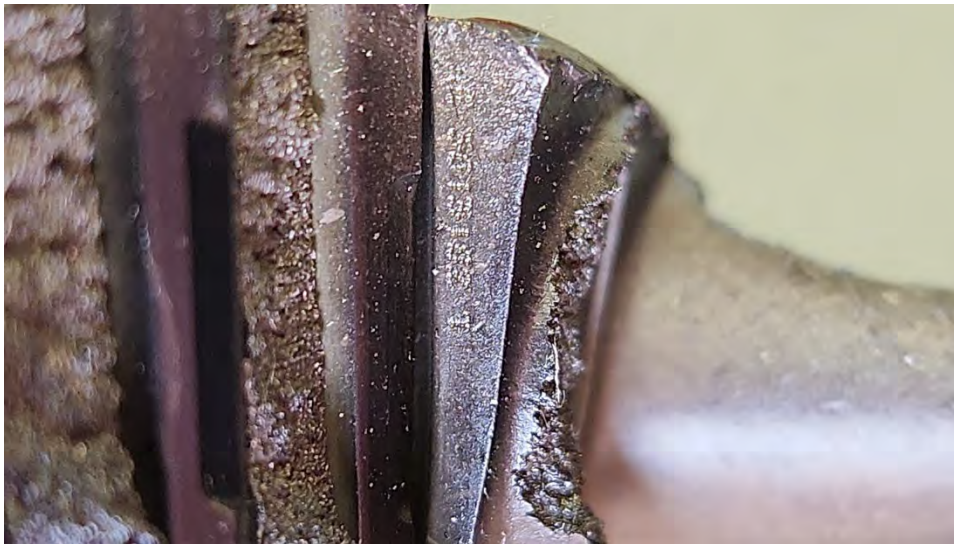
Blade part number AE 3013102T. All blades will need to be removed from disk, analyzed and PN verified
