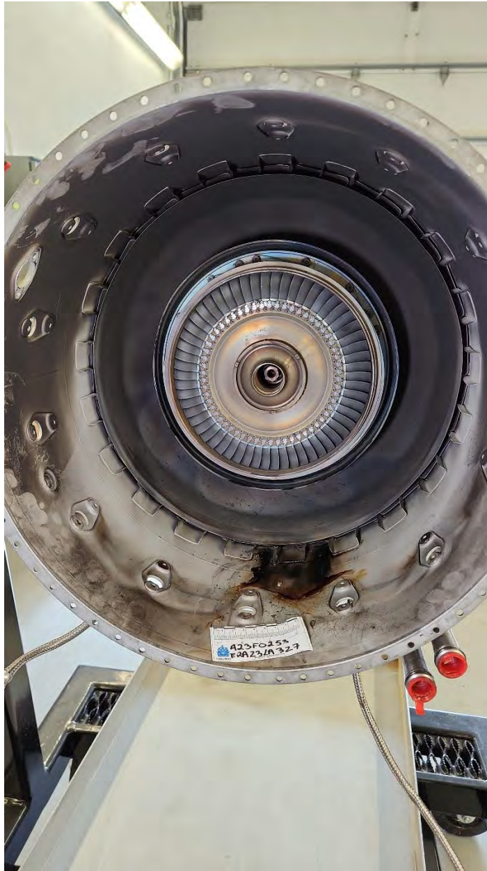
CT wheel Trailing edge looking aft
