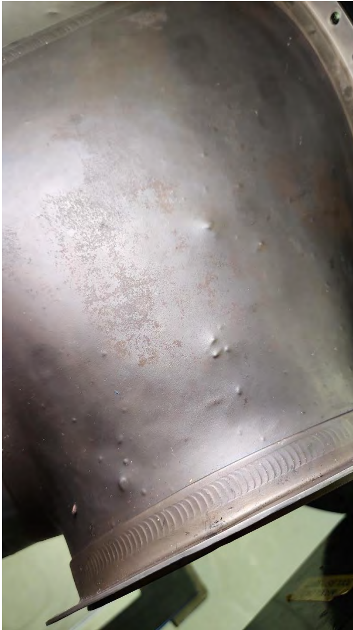
Dimple damages from departing PT blades
