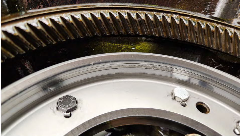
Torque plate scoring. No visible damage found on ring gear
