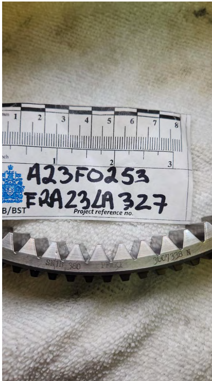
Ring gear part number. PN and SN were visible and therefore the groove on the ring gear was installed the right way (aft)
