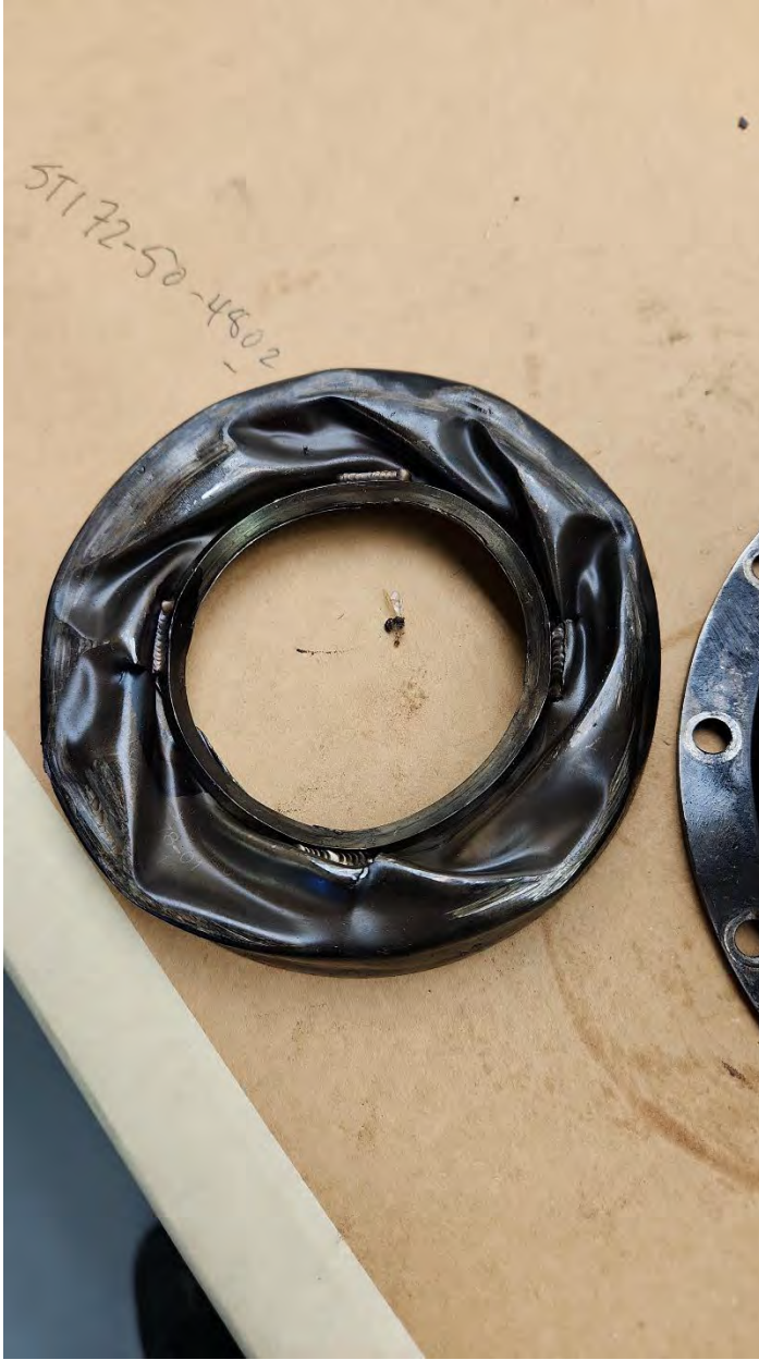
Tip of power turbine shaft casing between bearing 3 and PT wheel
