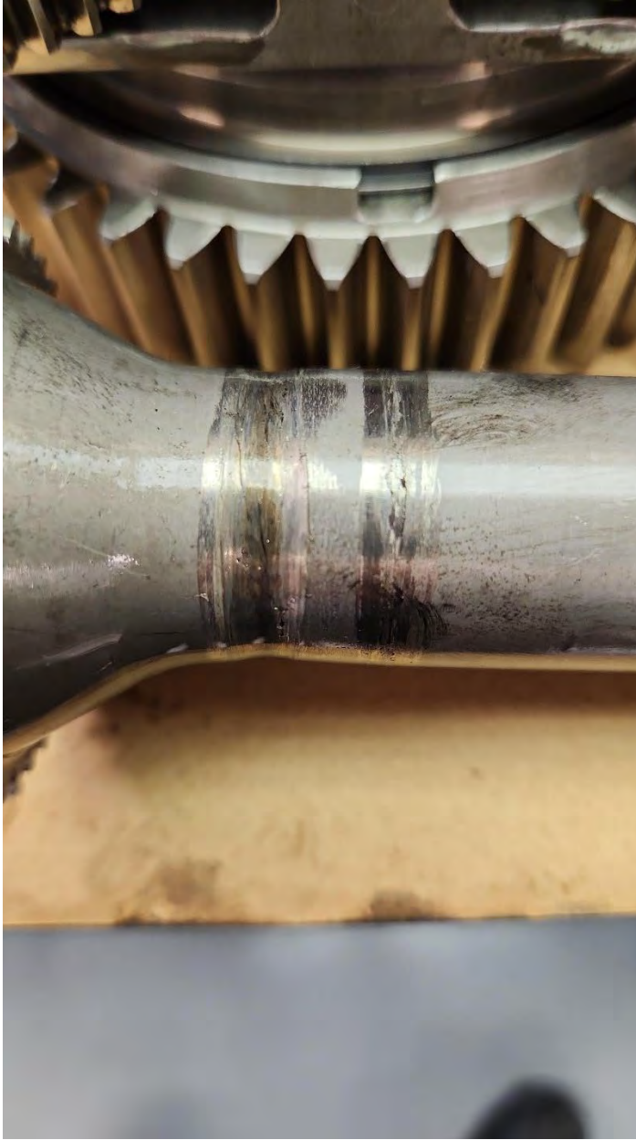
Scoring/rubbing on PT shaft
