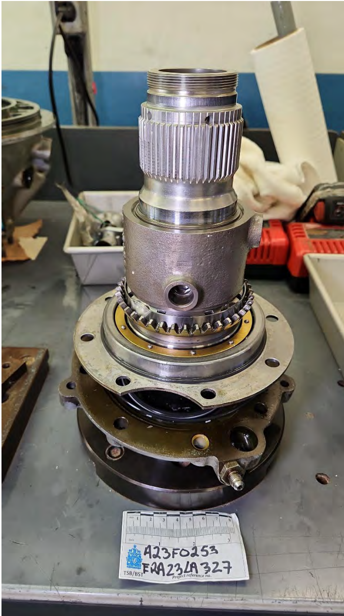
FWD prop shaft
