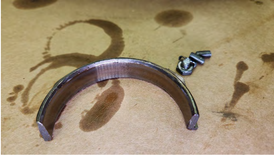
Bearing #3 race found in 2 separate parts no evident signs of scraping or overheat on the race All 4 bolts holding the race found sheared
