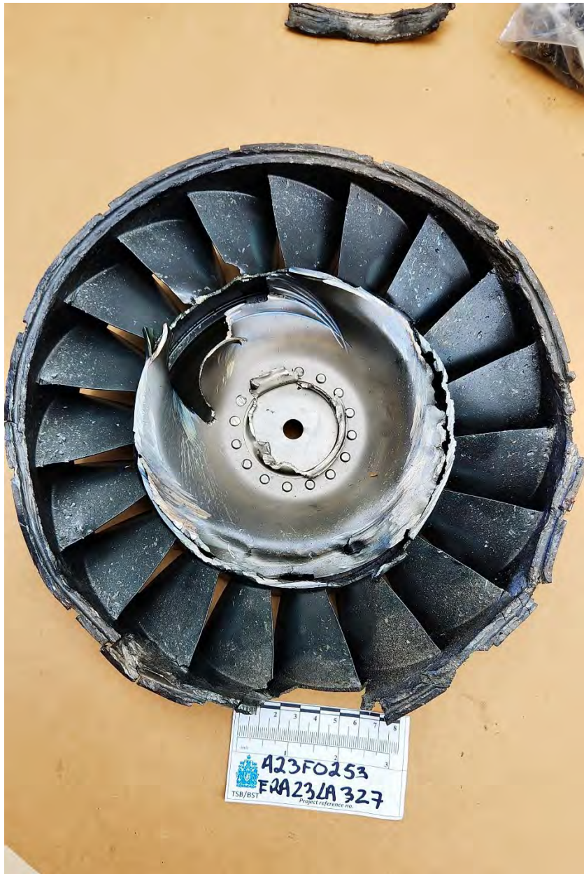
Stator vanes between CT and PT seen from trailing edge with damages on PT side
