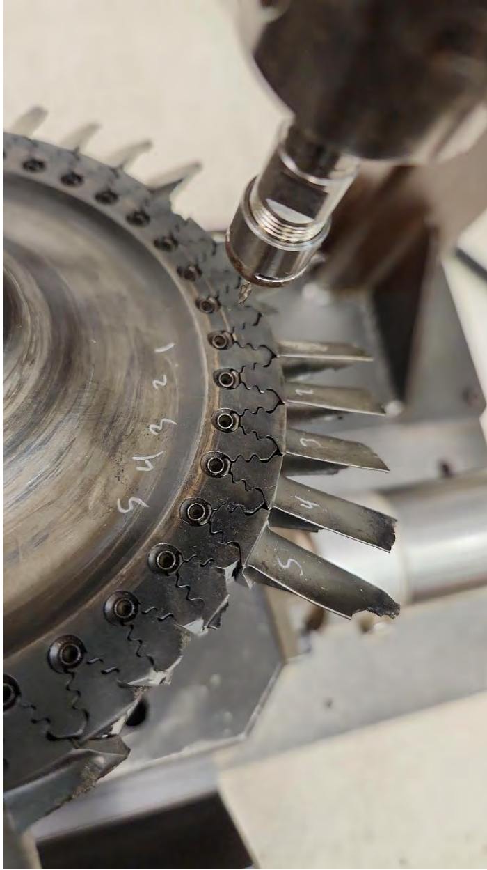
5 blades were removed to confirm part numbers. Blades were identified.
