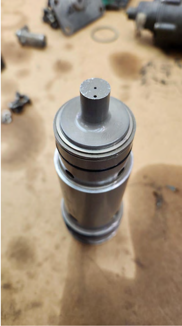
Inner core with damages
