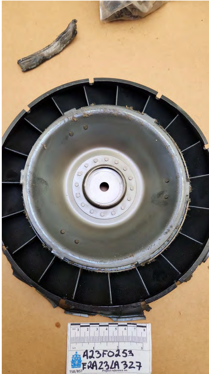
Leading edge's view (center part show evidence of rotational signature with CT disk due to rubbing evidence)
