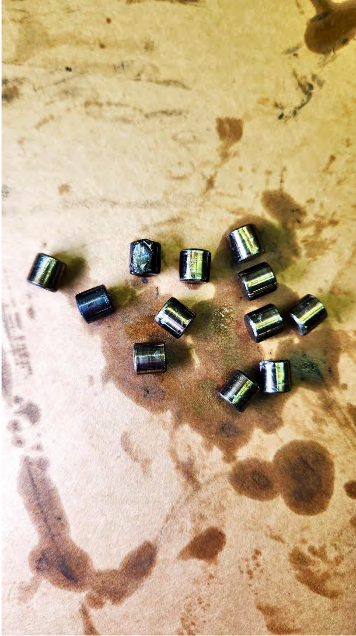
Bearing roller found with heat damage and rubbing
