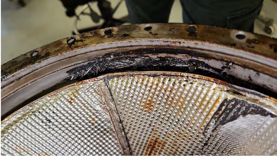
Bottom of RGB rear casing with debris
