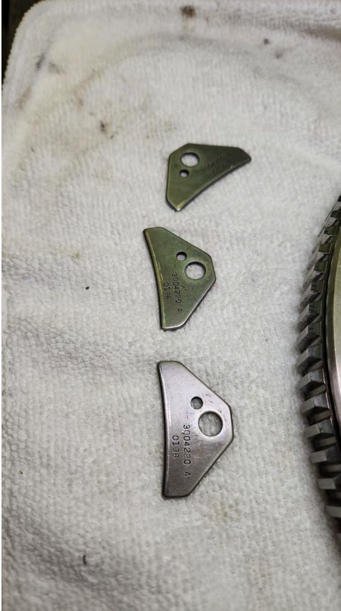
Wear on top of brackets may indicate it was installed properly at some point during the life of the ring gear/tabs
