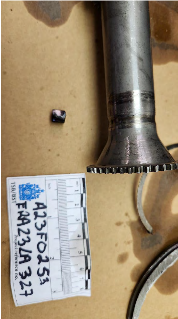
Most likely this roller was stuck between shaft and tube
