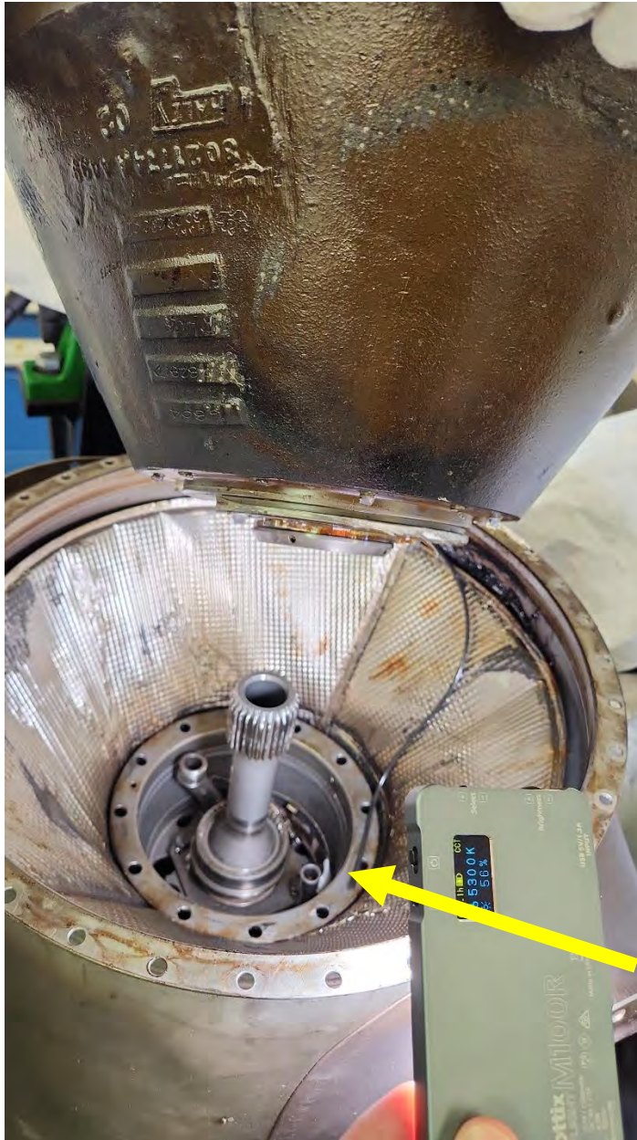
All bolts on gear RGB rear case found sheared and #3 roller bearing at bottom (please do not mind the light...)
