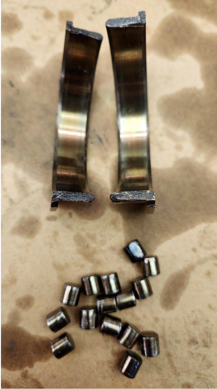
Bearing 3 race and found roller (One roller was not found). #3 bearing race did not exhibit sign of overheat or heavy scoring
