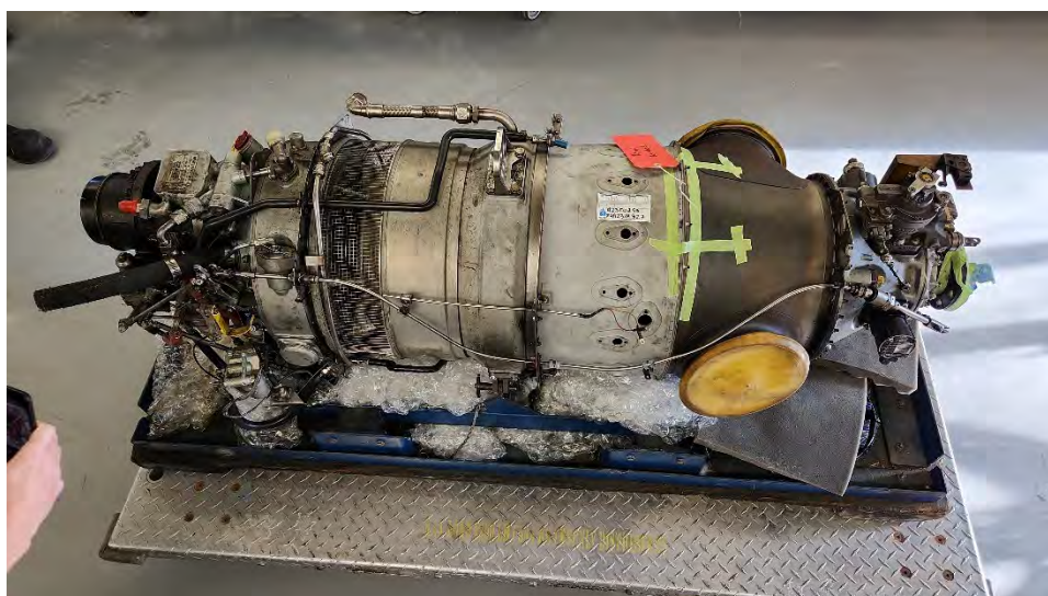
Casing split on c flange. Combustion can liner found missing from shipment
