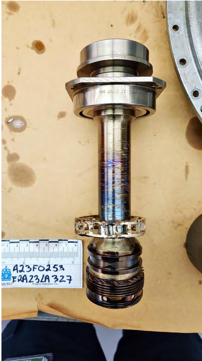
PT shaft overheat signature.
