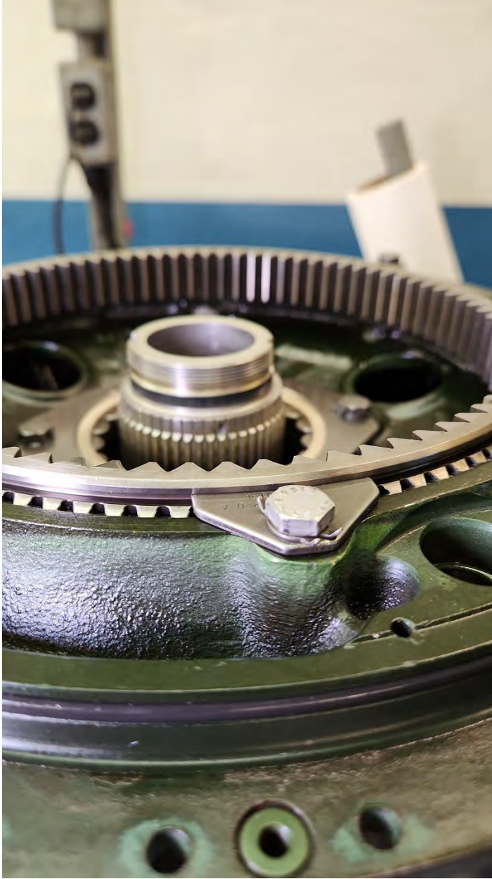
For demonstration ONLY. Ring gear correctly installed in groove to prevent axial play
