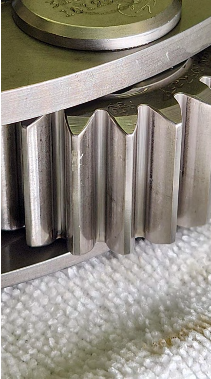
Second stage planetary gear with damages
