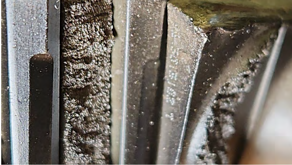
Blade part number AE 3013102T. All blades will need to be removed from disk, analyzed and PN verified
