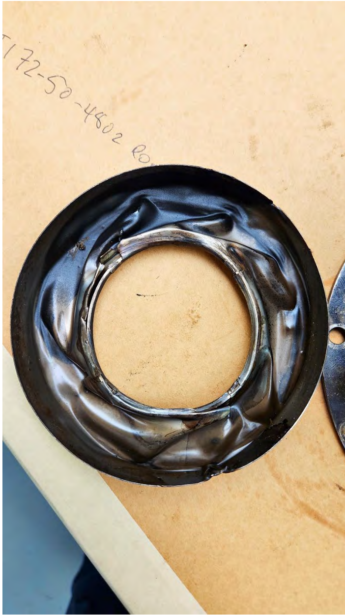
Power turbine shaft cap between PT shaft housing and PT wheel exhibit evidence of crushing and torsional force
