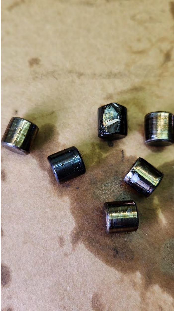
2 bearing roller indicated signs of rubbing and overheat signatures
