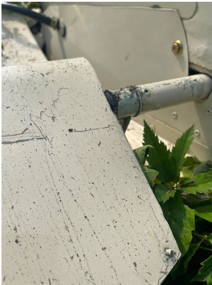
Photograph 3 – Fuel Staining on RH Flaperon (Courtesy of Tyler Hodge)
