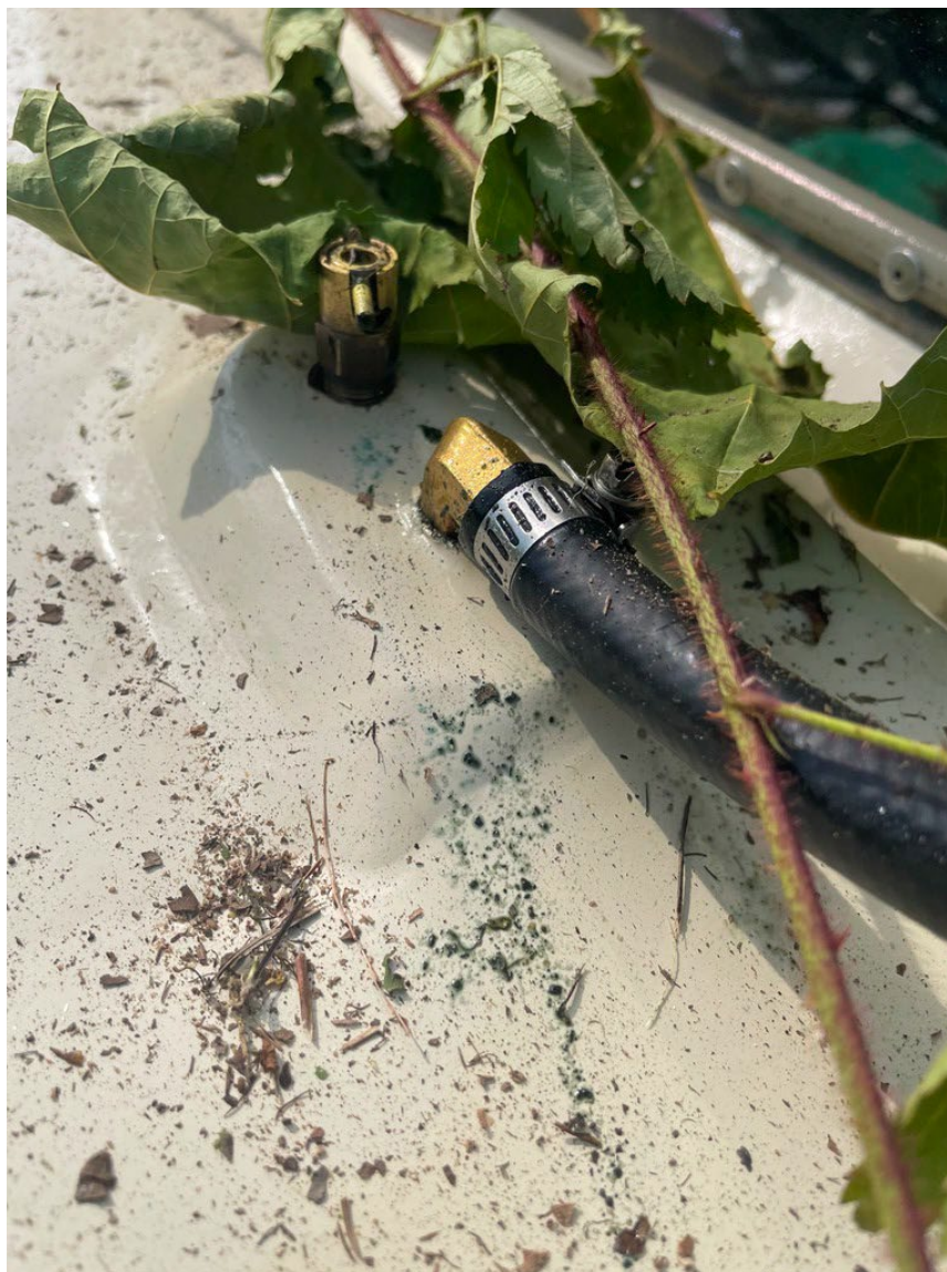
Photograph 2 – Fuel Staining Around Fuel Drain Valve on Right Wing (Courtesy of Tyler Hodge)
