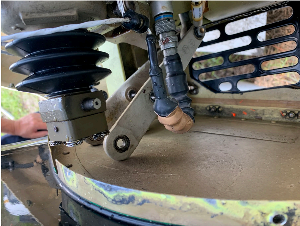
Photograph 5 - Tail Rotor Pitch Change Trunnion and Lever Assemblies (Courtesy of FAA)
