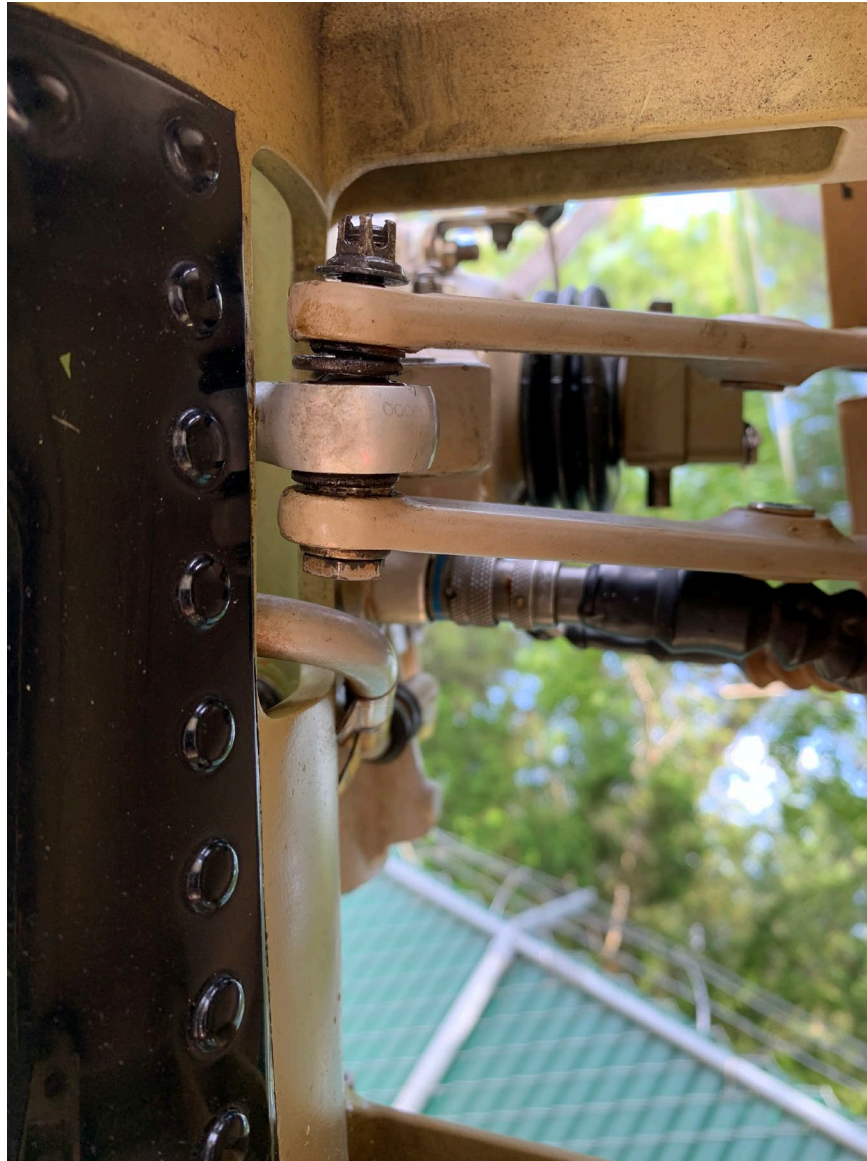
Photograph 6 - Tail Rotor Pitch Change Trunnion and Lever Assemblies (Courtesy of FAA)
