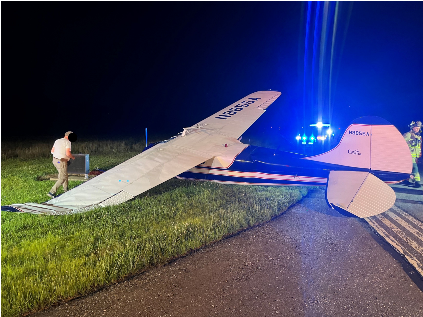
Photo 2 – View of Damage to Left Wing (LAA)
