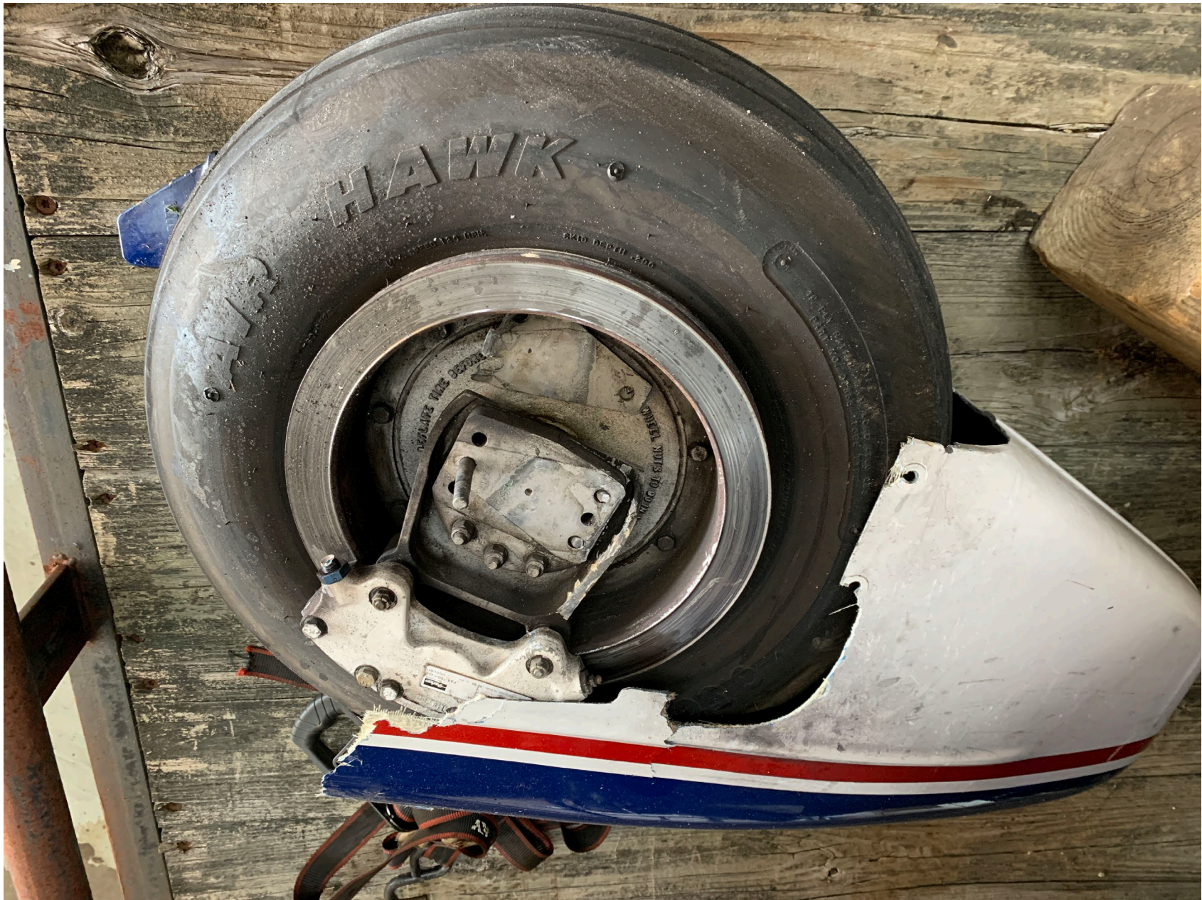
Photo 3 – View of Left Main Landing Gear Mount Studs (LAA)
