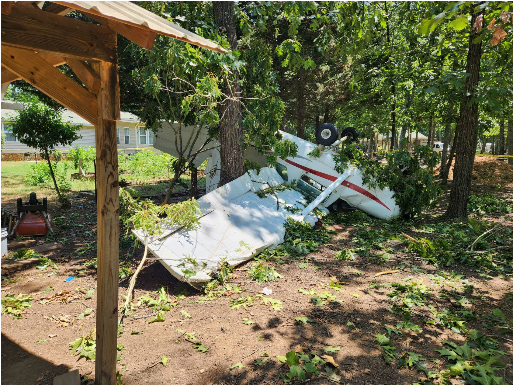
Photo 2 - FAA Digital Photograph. Left Side View of the Inverted Airplane at the Accident Site.
