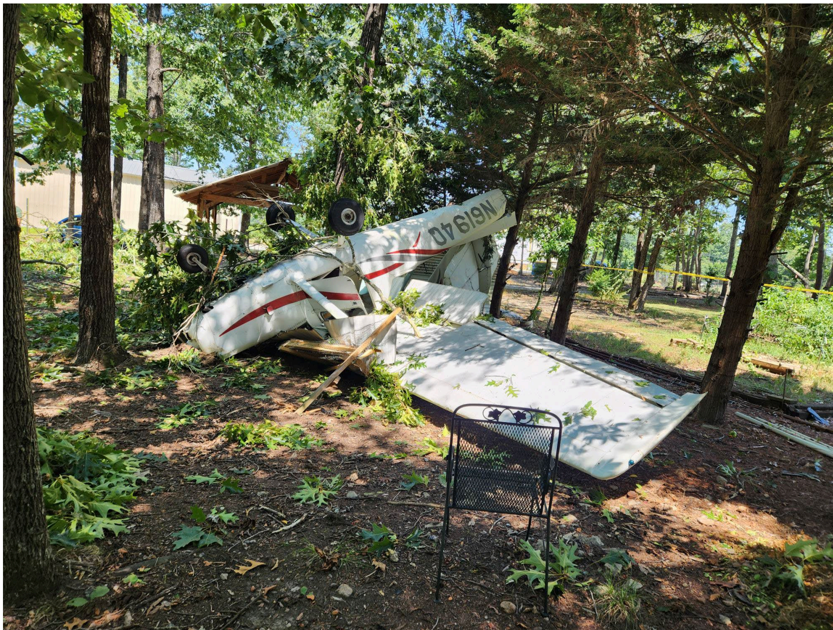
Photo 1 – FAA Digital Photograph. Right Side View of the Inverted Airplane at the Accident Site. Note the Extended Right Flap.
