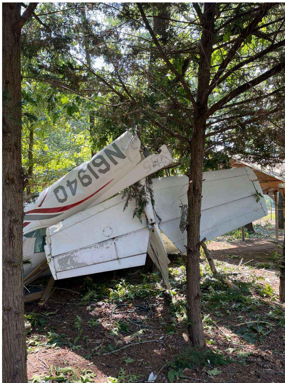
Photo 4 - FAA Digital Photograph. Right Side View of the Inverted Airplane at the Accident Site. Note the Nearly Separated Aft Empennage.
