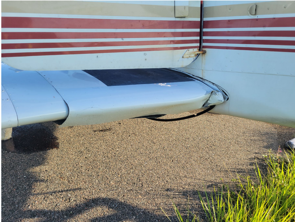
Photograph 2 - Right wing root showing damage (Courtesy of FAA)
