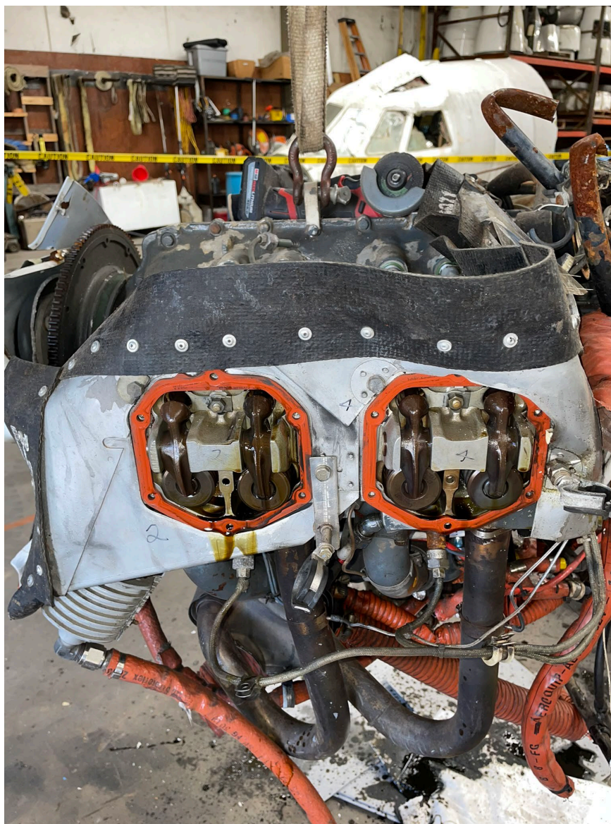
Photograph 5 - View of Nos. 2 and 4 side with valve covers removed. (NTSB)
