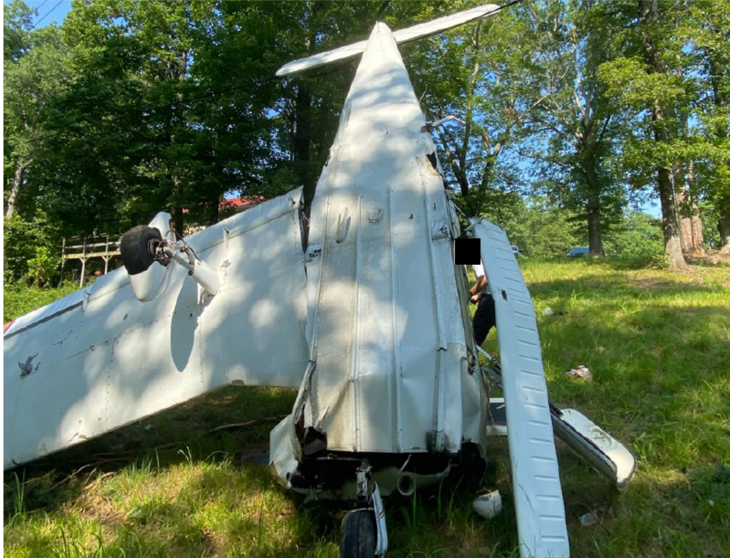
Figure 2 Airplane wreckage from bottom of aircraft showing wing separation.
