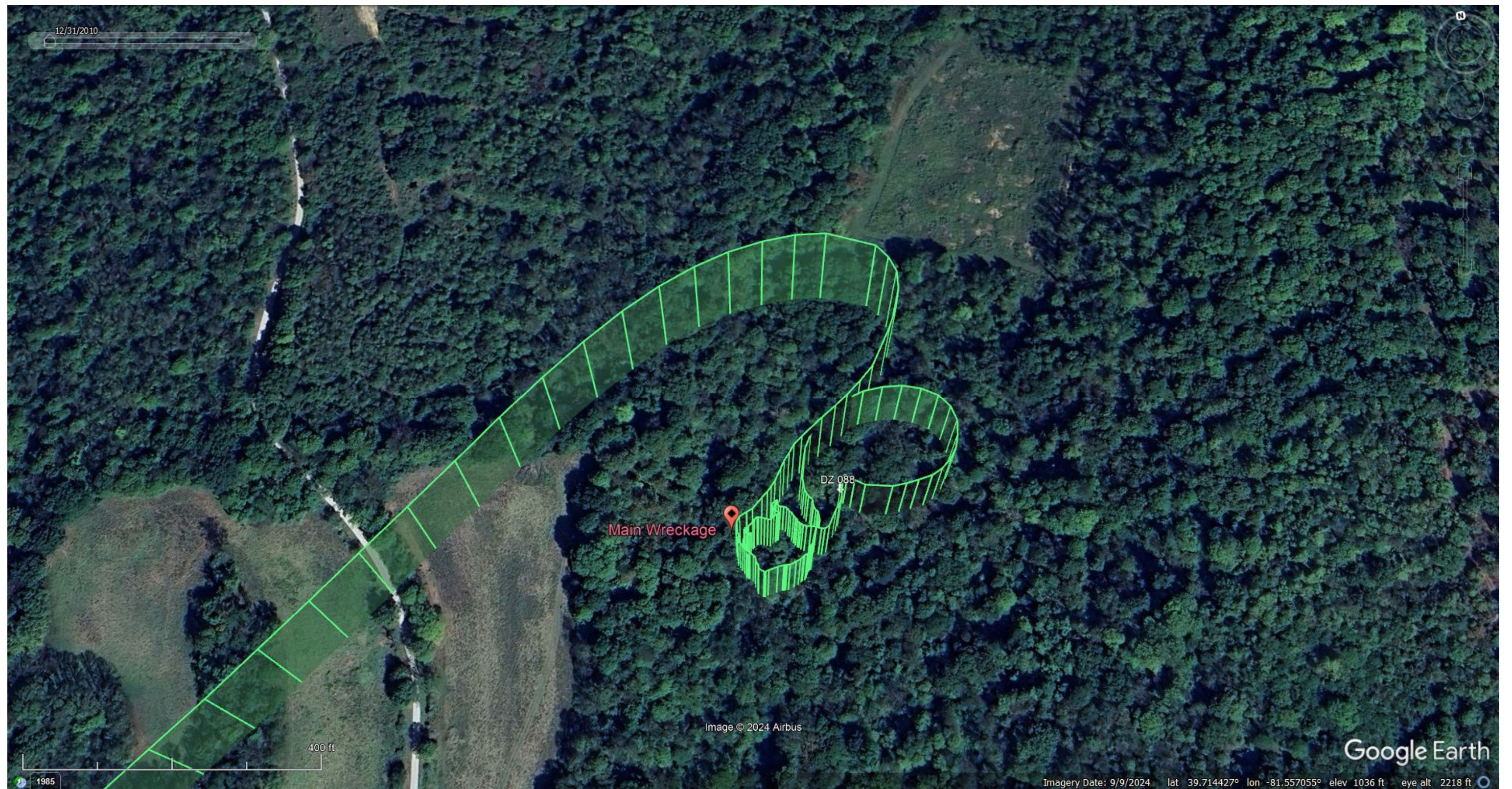
Figure 9: Flight path reconstruction (green lines) of N482TJ making clockwise approach to drop zone 088 during the accident flight, maneuvering, and experiencing an uncontrolled vertical descent and terrain impact. Due north is toward the top of the page.
