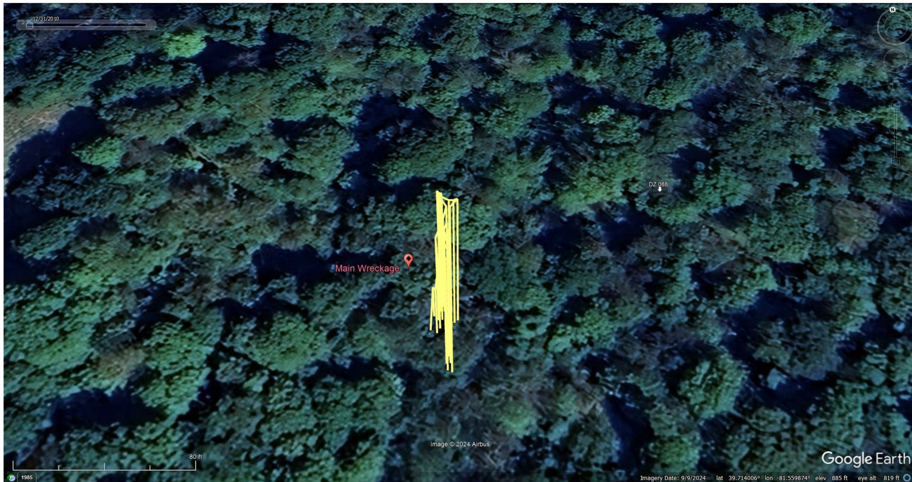
Figure A4.15: Flight path reconstruction (yellow lines) of N482TJ maneuvering near drop zone 088 during the accident flight about 30 seconds prior to experiencing an uncontrolled vertical descent and terrain impact. Due north is toward the top of the page.
