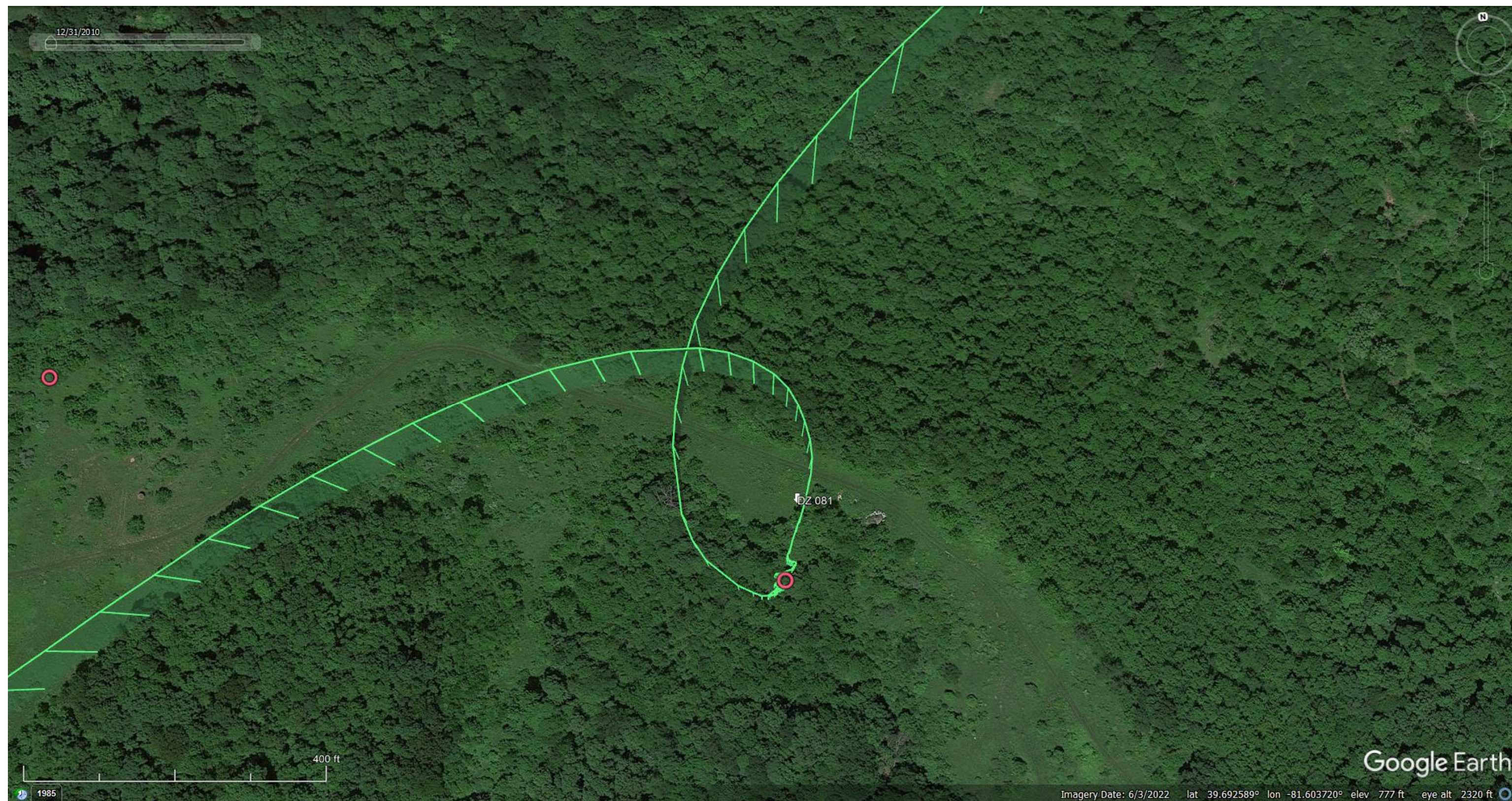
Figure A4.3: Flight path reconstruction (green lines) of N482TJ making clockwise approach to (and departure from) drop zone 081 during the pre-accident flight. Due north is toward the top of the page.
