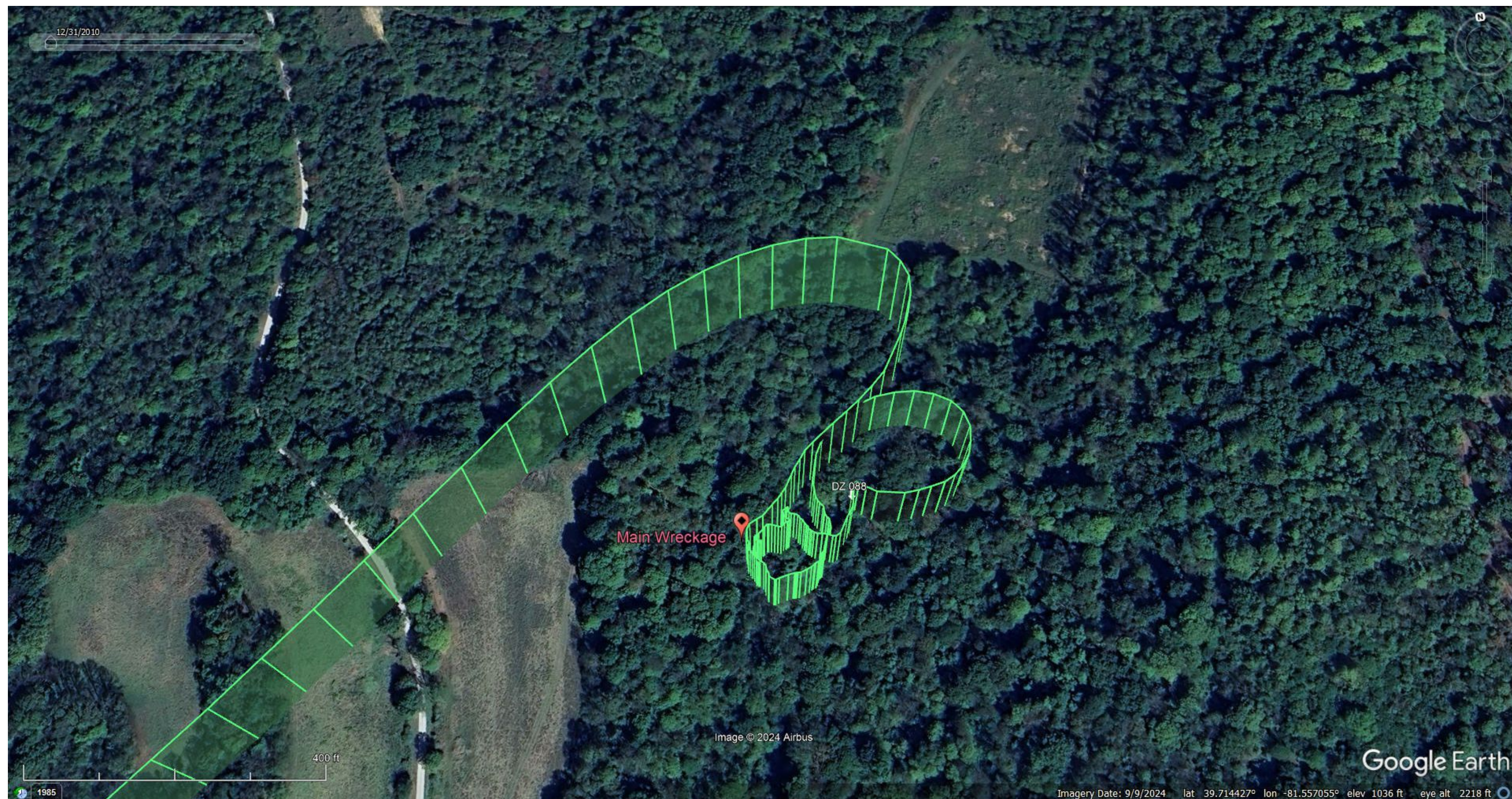
Figure A4.11: Flight path reconstruction (green lines) of N482TJ making clockwise approach to drop zone 088 during the accident flight, maneuvering, and experiencing an uncontrolled vertical descent and terrain impact. Due north is toward the top of the page.
