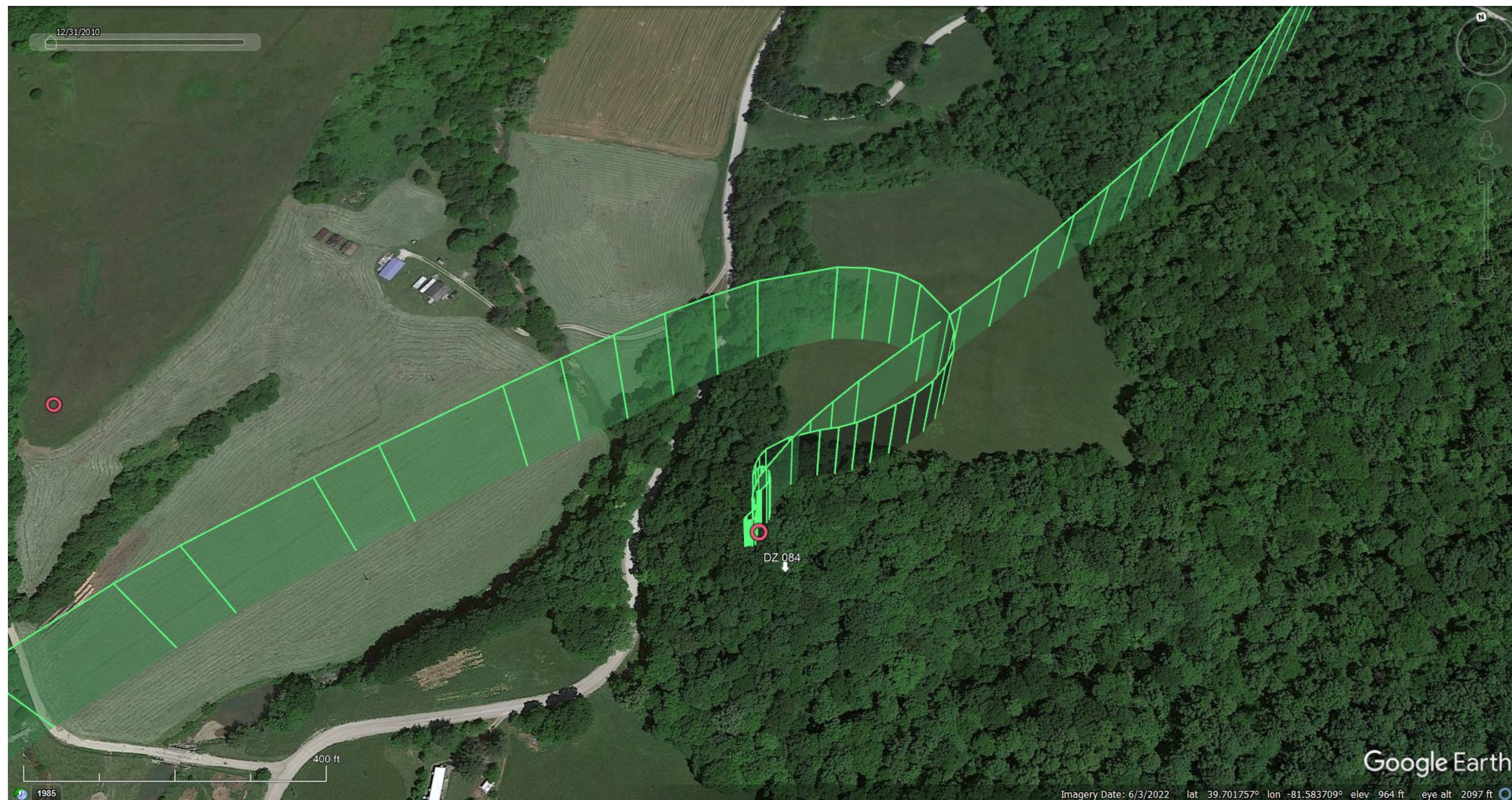
Figure A4.6: Flight path reconstruction (green lines) of N482TJ making clockwise approach to (and departure from) drop zone 084 during the pre-accident flight. Due north is toward the top of the page.
