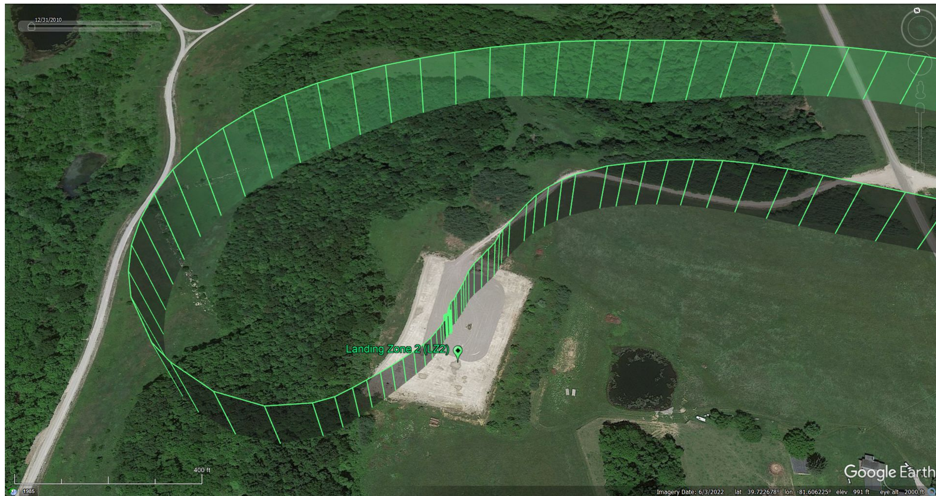
Figure A4.9: Flight path reconstruction (green lines) of N482TJ making clockwise approach to (and departure from) drop zone LZ2. Due north is toward the top of the page.
