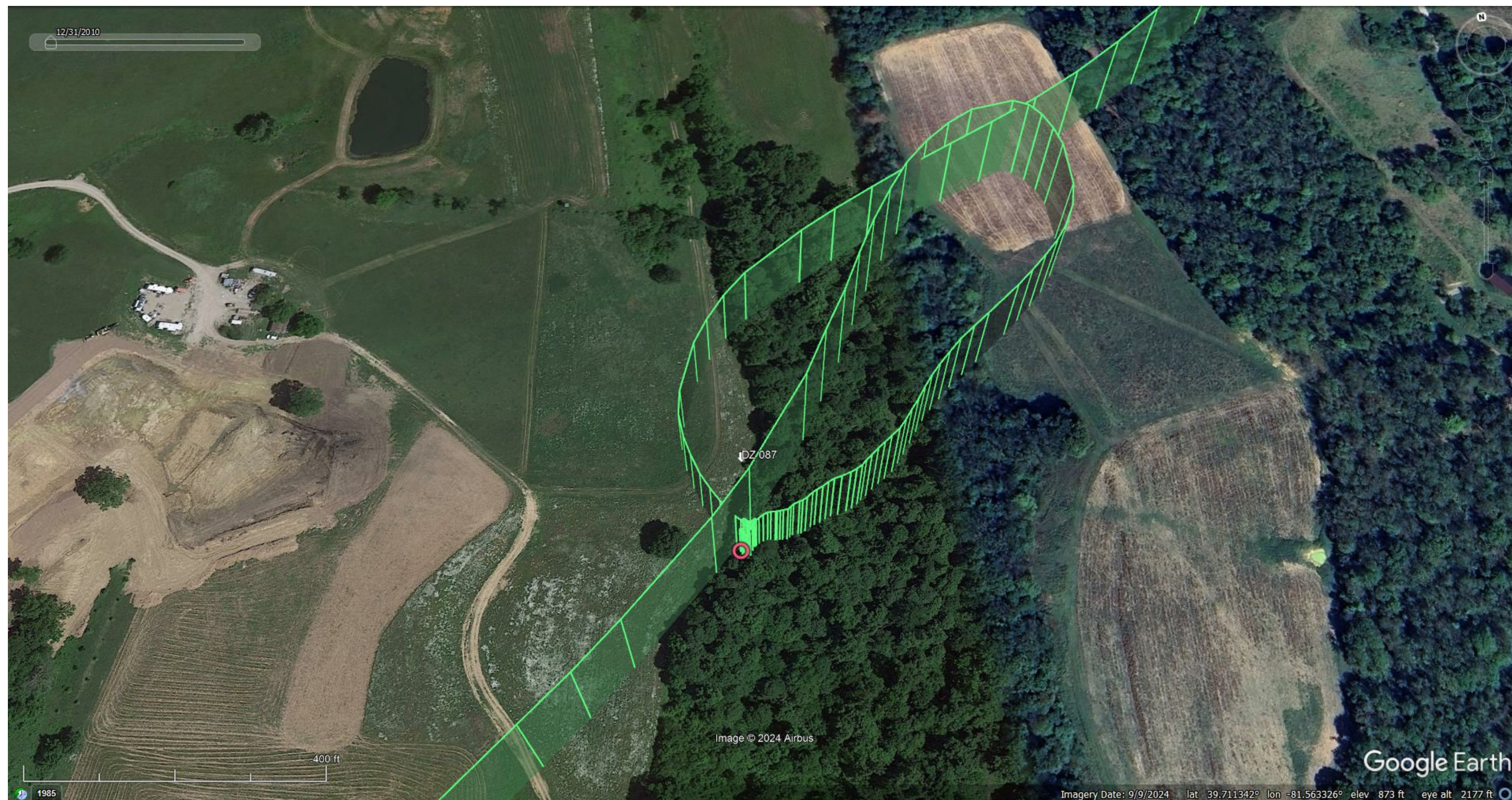
Figure A4.10: Flight path reconstruction (green lines) of N482TJ making clockwise approach to (and departure from) drop zone 087 during the accident flight. Due north is toward the top of the page.
