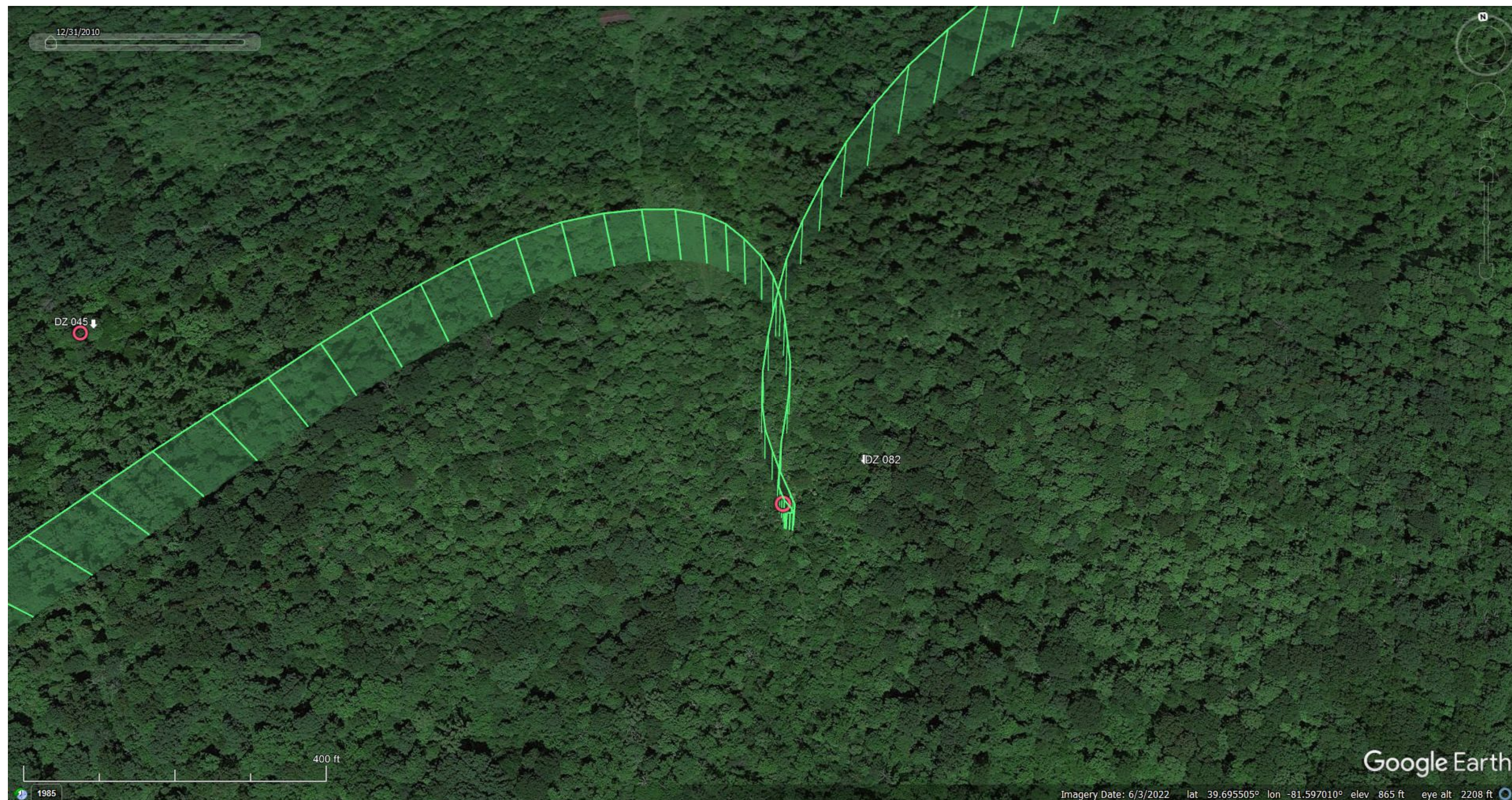
Figure A4.4: Flight path reconstruction (green lines) of N482TJ making clockwise approach to (and departure from) drop zone 082 during the pre-accident flight. Due north is toward the top of the page.
