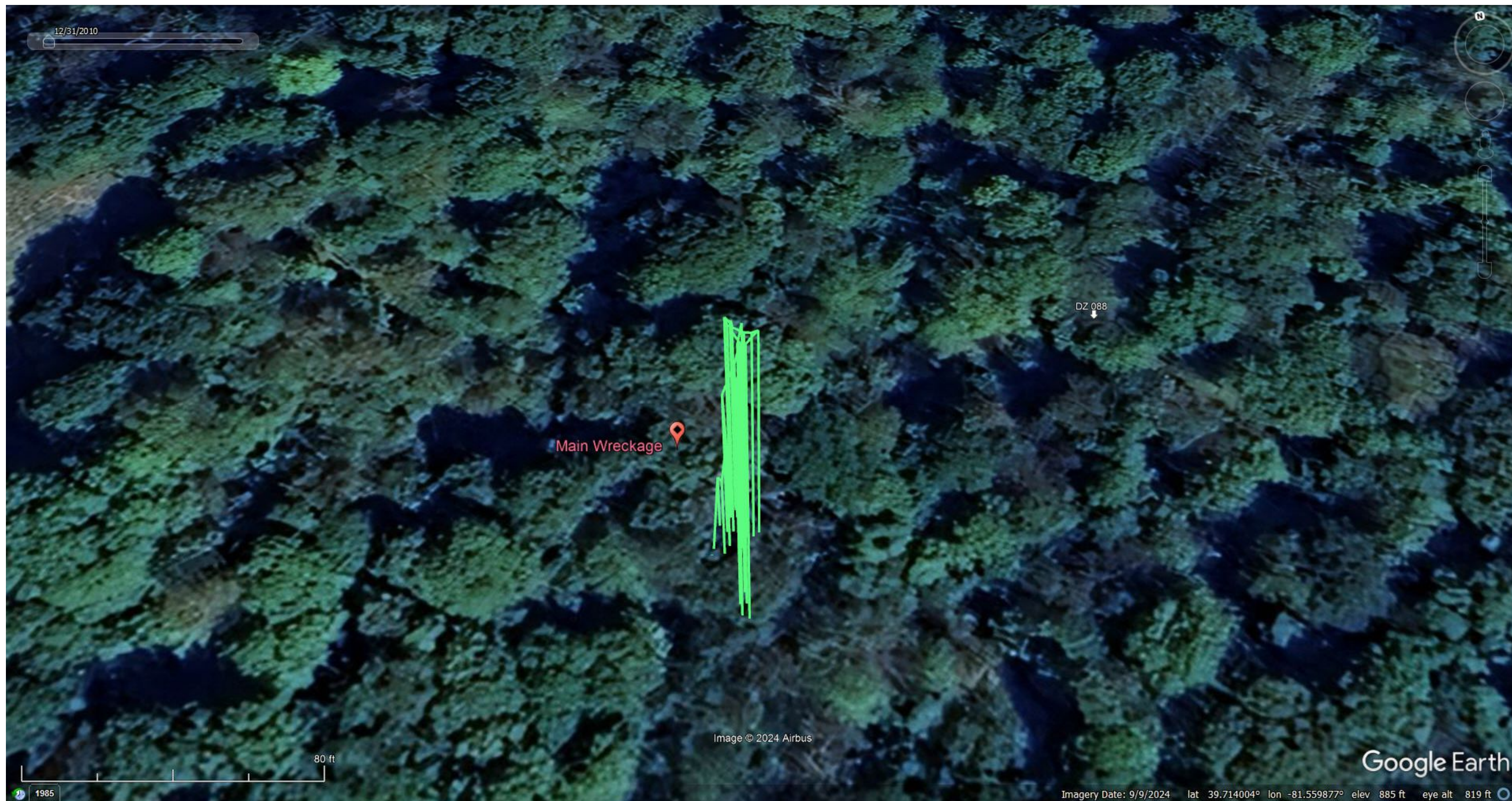
Figure A4.14: Flight path reconstruction (green lines) of N482TJ maneuvering near drop zone 088 during the accident flight about 40 seconds prior to experiencing an uncontrolled vertical descent and terrain impact. Due north is toward the top of the page.
