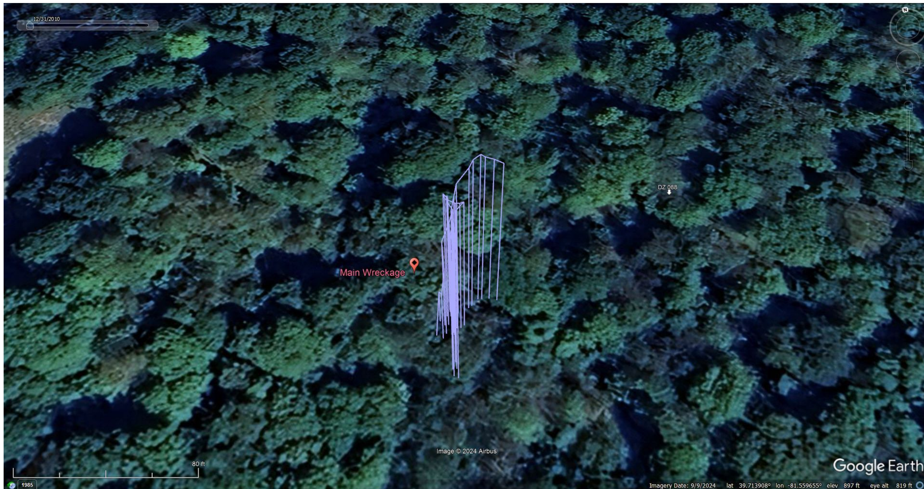
Figure A4.13: Flight path reconstruction (blue lines) of N482TJ maneuvering near drop zone 088 during the accident flight about 50 seconds prior to experiencing an uncontrolled vertical descent and terrain impact. Due north is toward the top of the page.
