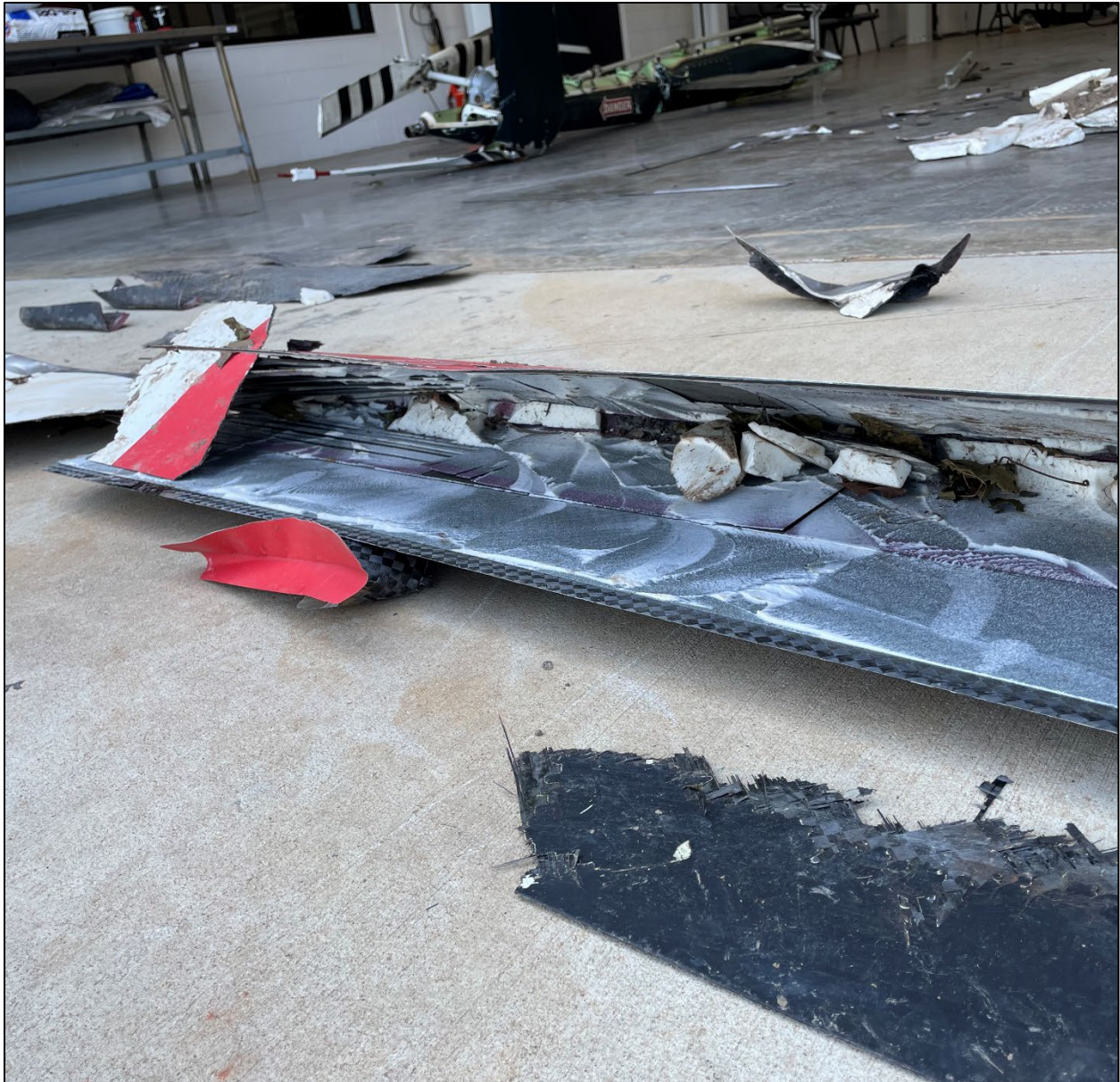
Figure 21: View of the main rotor blade recovered fragments.
