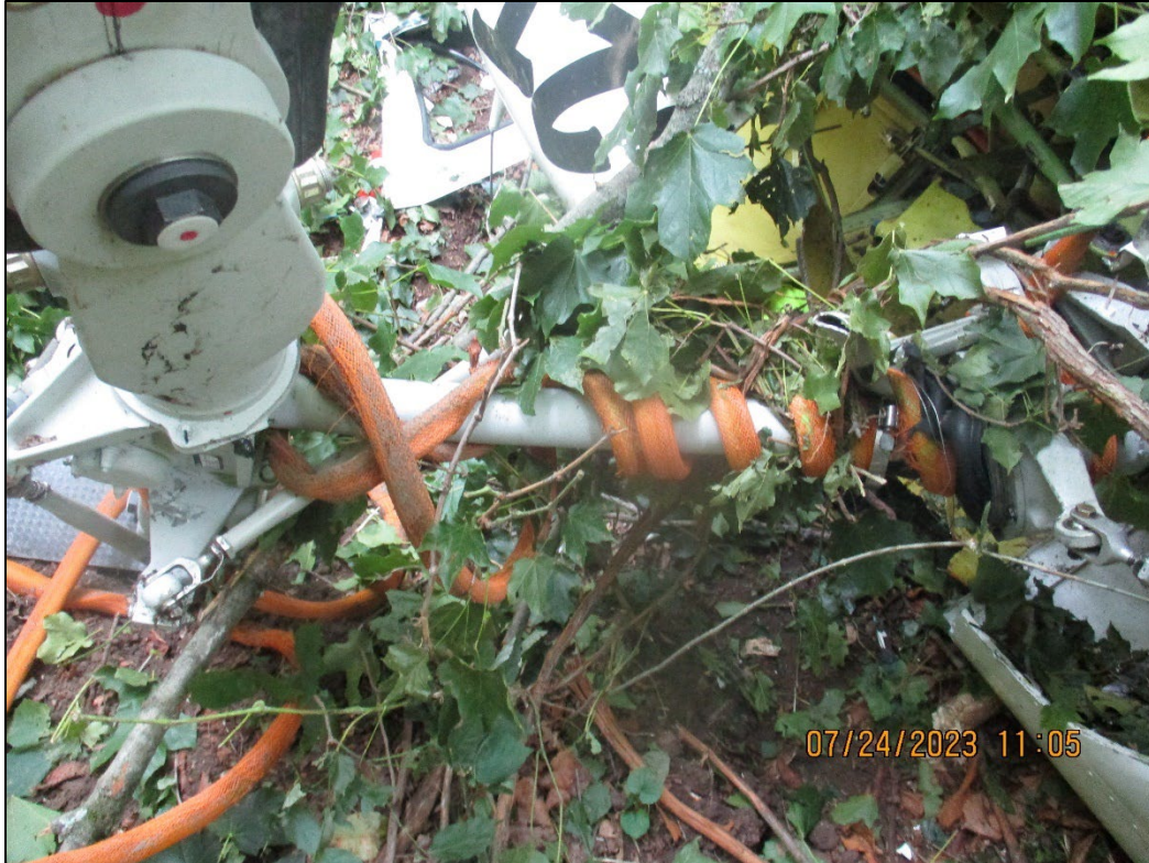
Figure 9: Additional view of the long line wrapped around the main rotor drive shaft.
