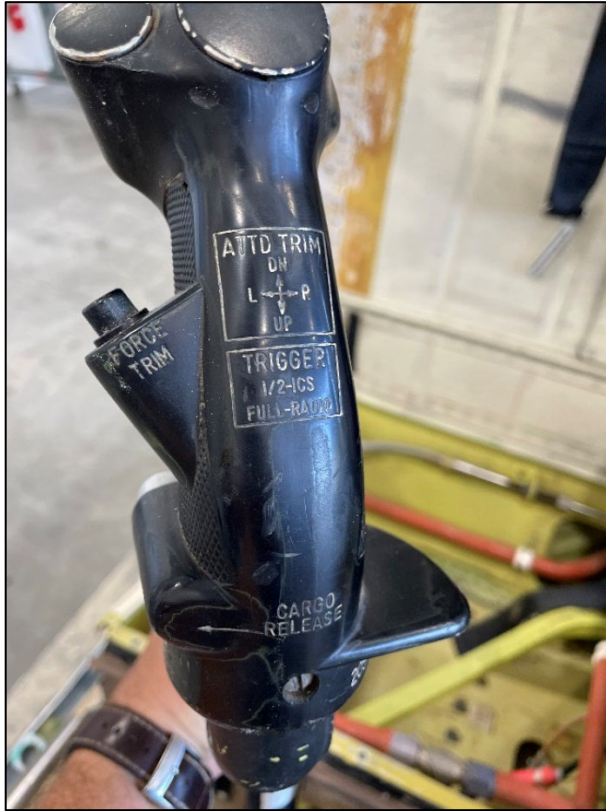
Figure 26: View of the control stick cyclic denoting the "Cargo Release." Right Side: Red handle, emergency cargo release (found closed - not released).
