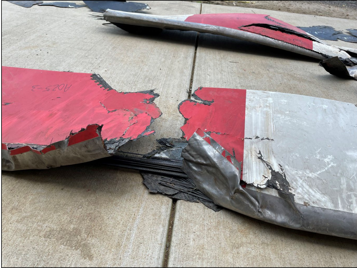
Figure 23: View of leading edge damage to A025 main rotor blade.
