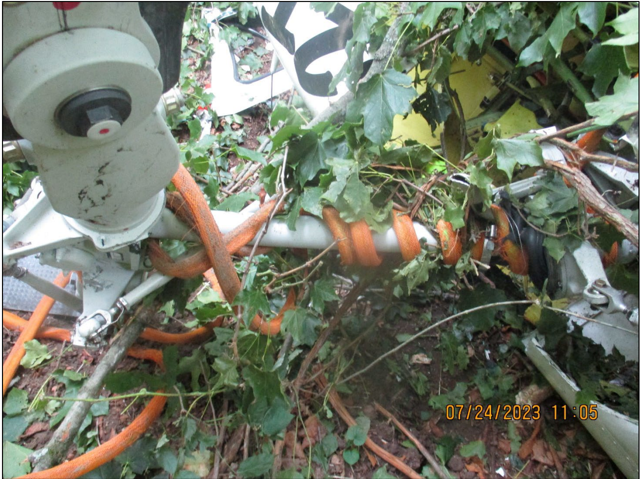
Figure 6: View of the helicopter and accident site area. Note the long line found wrapped around the main rotor drive shaft.
