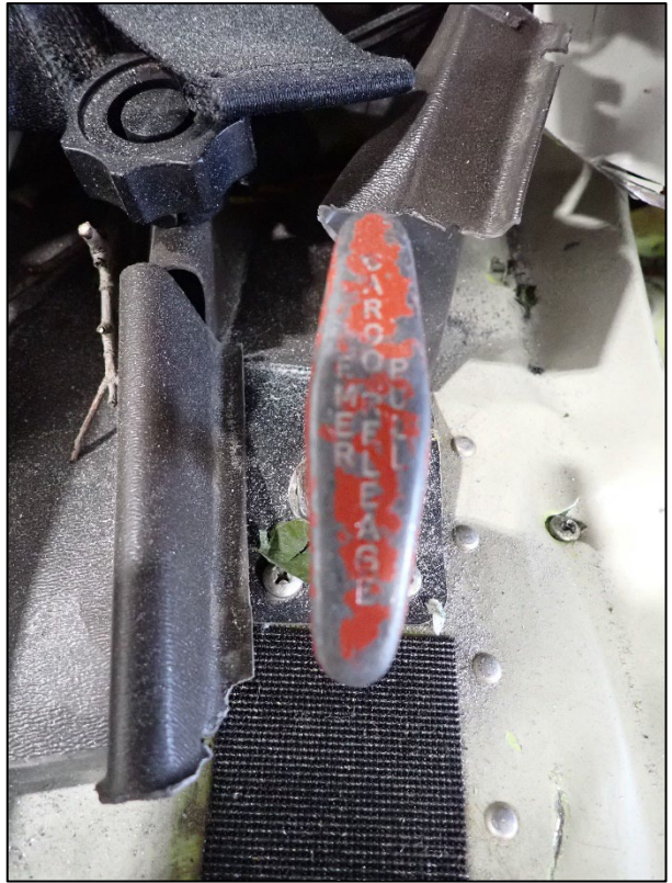
Figure 26: View of the control stick cyclic denoting the "Cargo Release." Right Side: Red handle, emergency cargo release (found closed - not released).
