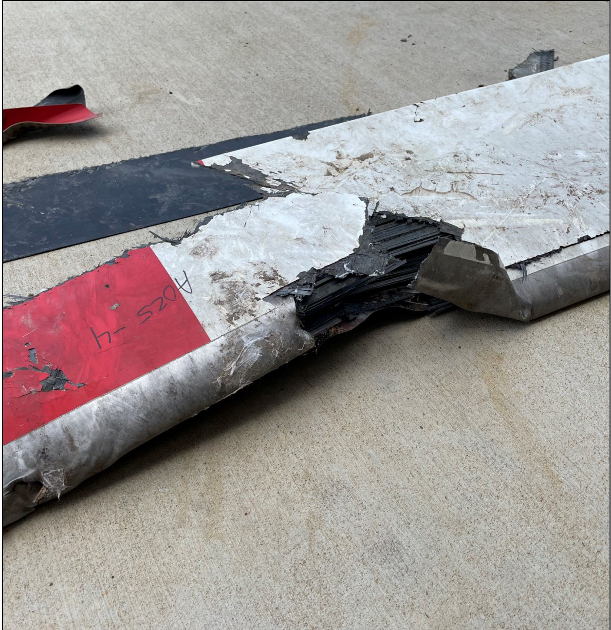
Figure 22: View of leading edge damage to A025 main rotor blade.
