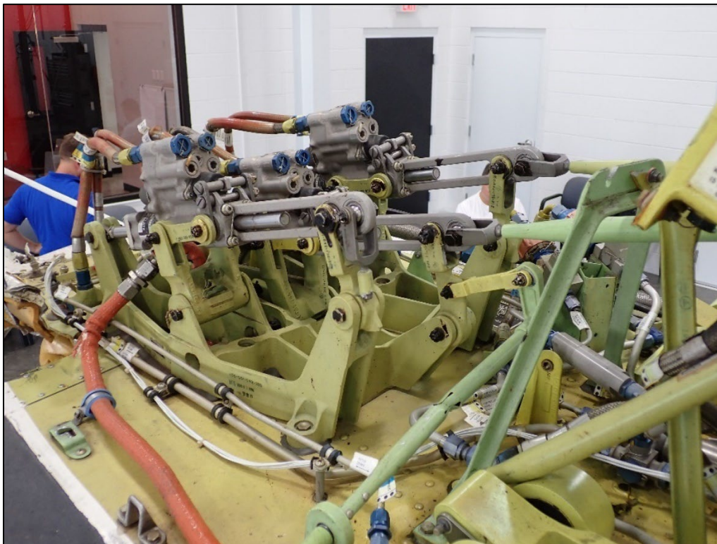
Figure 17: View of the servo actuators.
