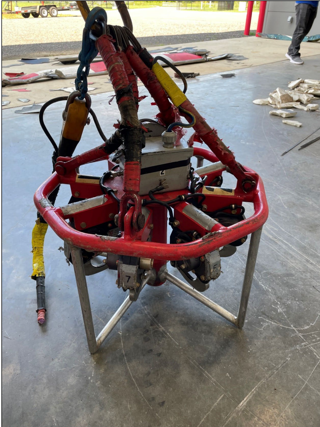
Figure 28: External load carrier with 8 separate release hooks.
