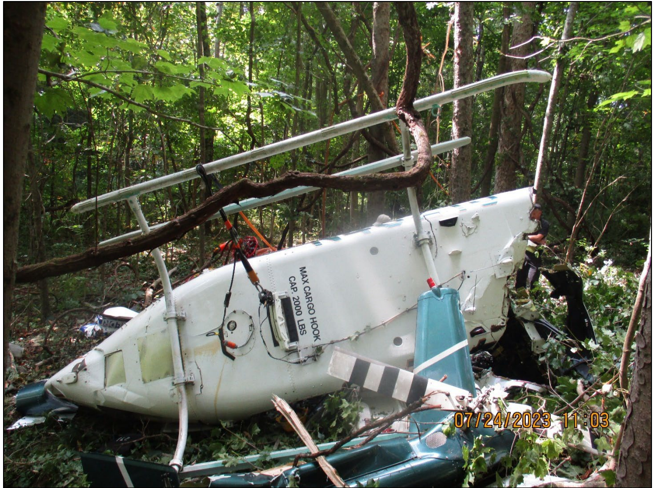
Figure 8: View of the helicopter and accident site area. Note the cargo hook remained closed/secured.
