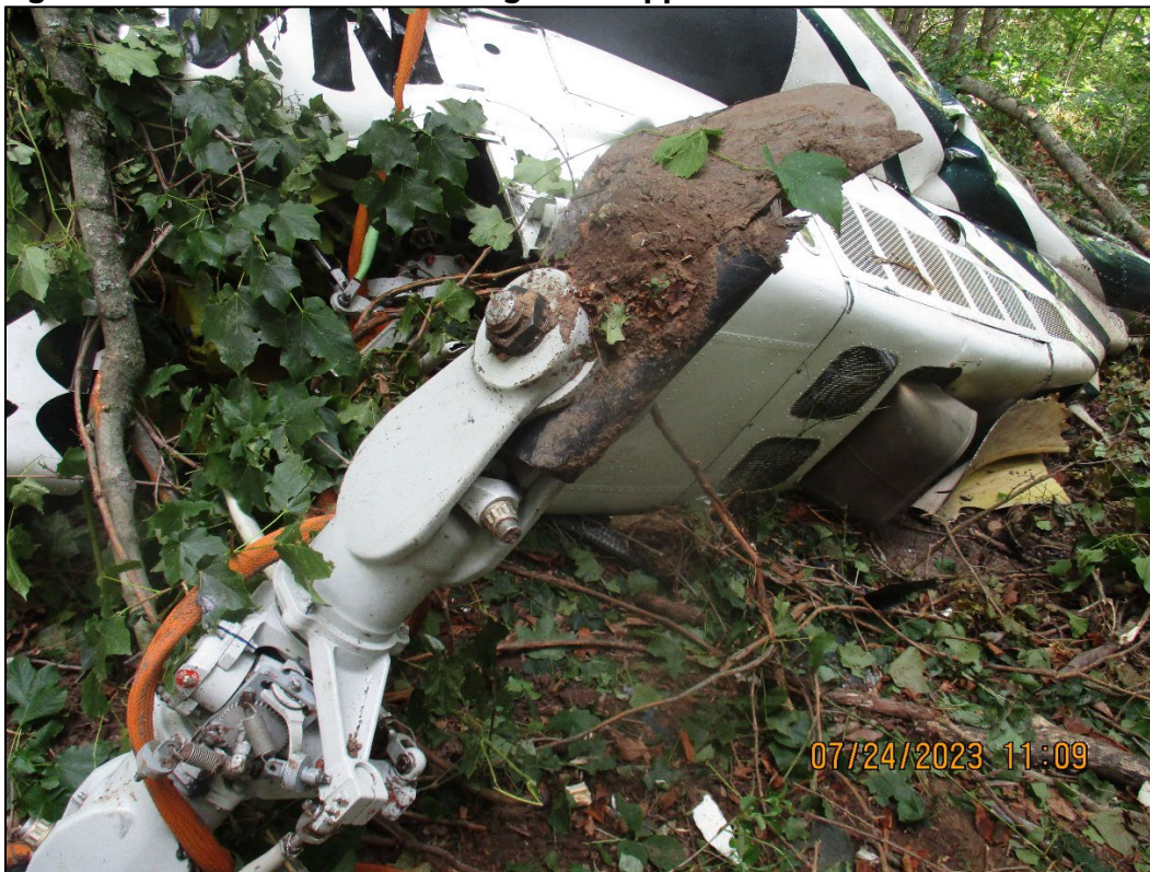
Figure 10: View of a main rotor blade with impact related dirt and debris affixed to its fracture area.
