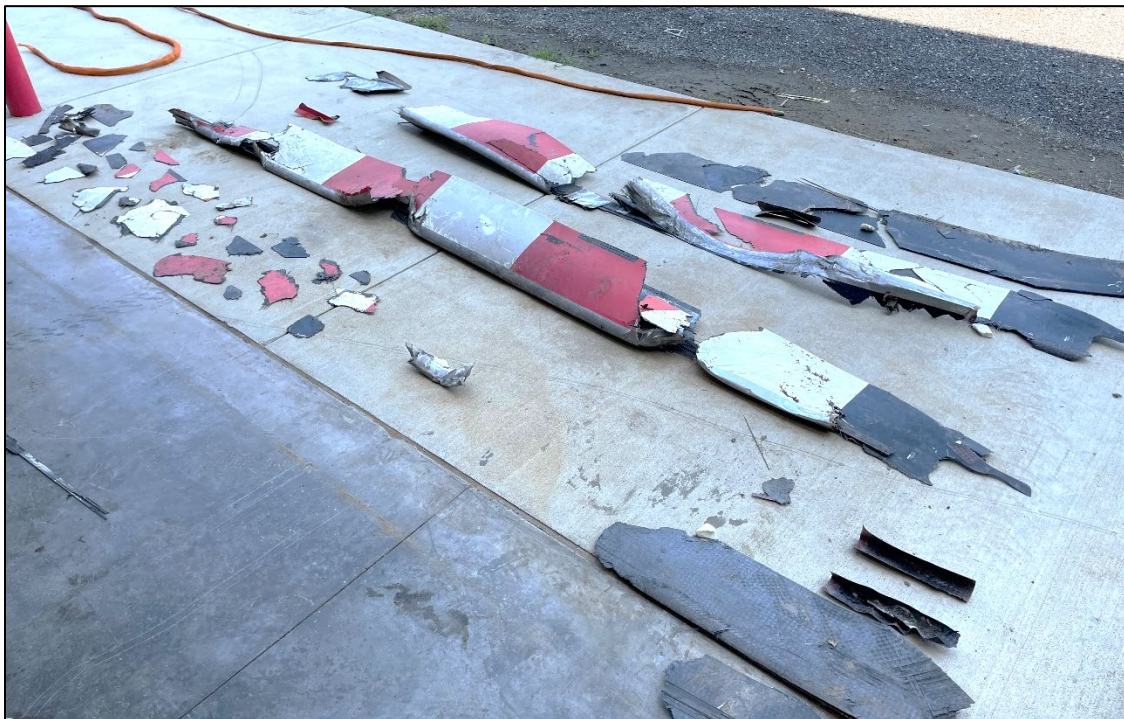
Figure 20: View of the main rotor blade recovered fragments.
