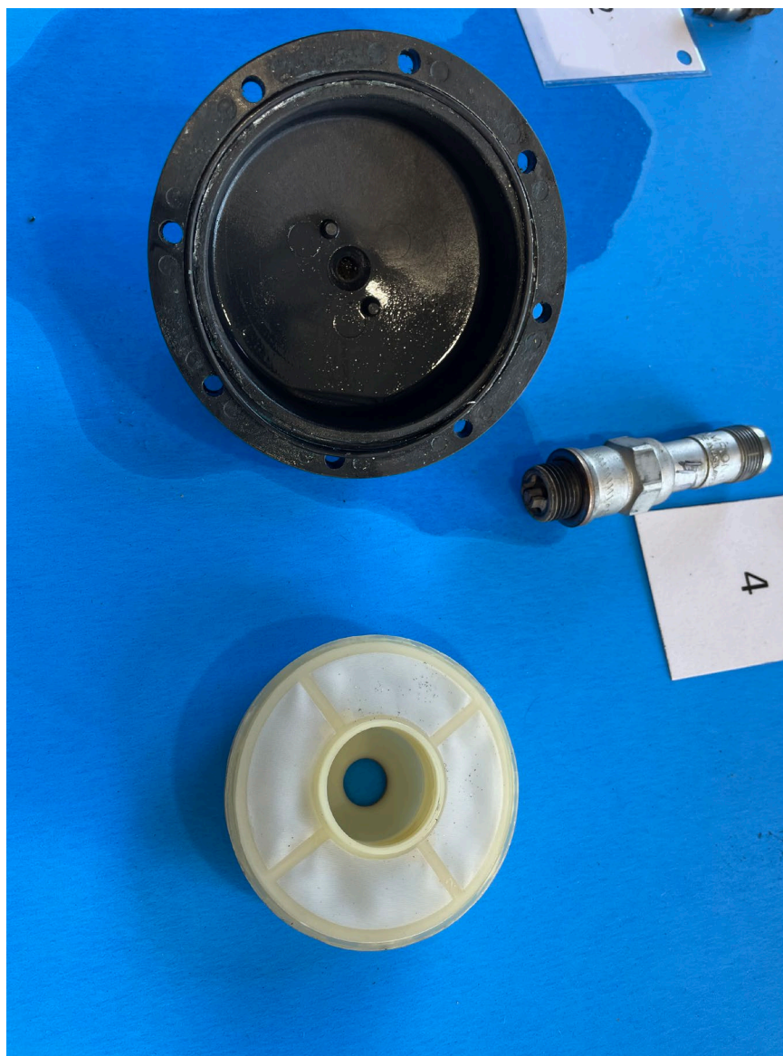
Photograph 7 - Fuel Strainer (NTSB Photo)
