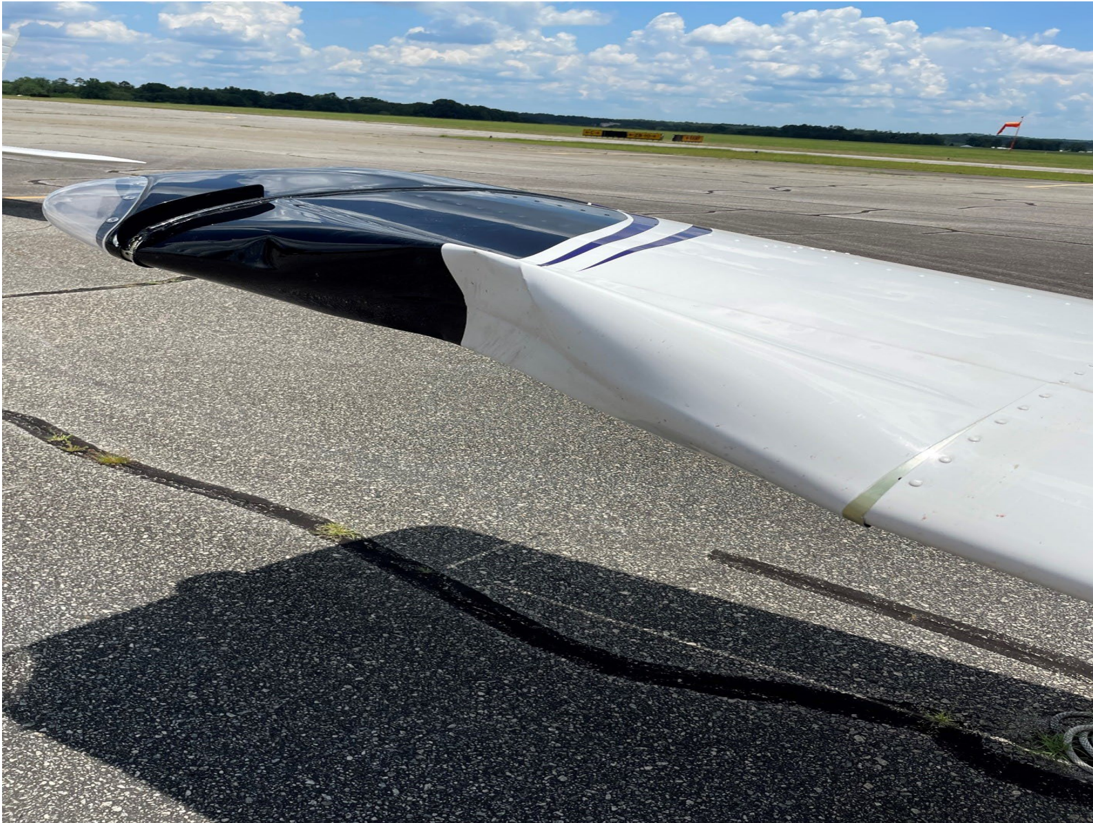
Photo 2: View of the damage to the right wing. (Photo Courtesy of FAA)
