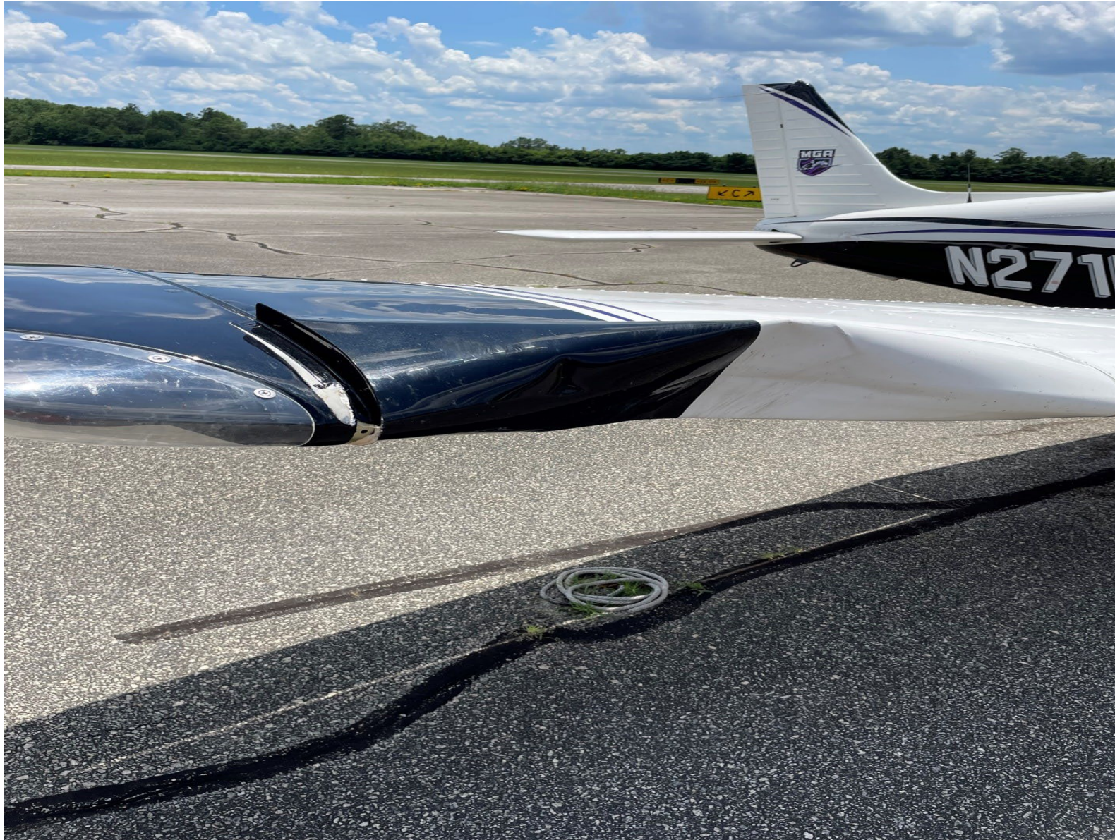
Photo 1: View of the damage to the right wing. (Photo Courtesy of FAA)
