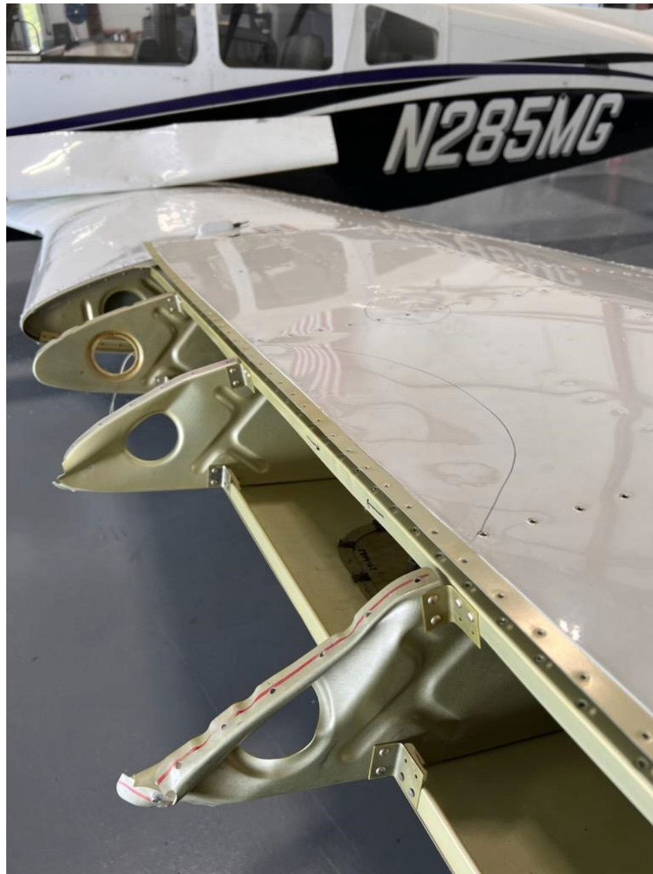
Photo 2 – View of Damaged Wing Ribs (MGSU)
