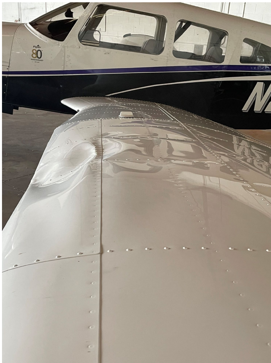
Photo 1 – View of Leading Edge and Wing Skin Damage (MGSU)
