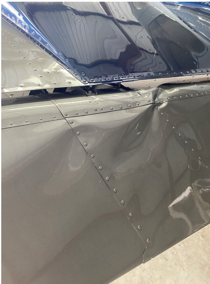
Photograph 2 - Flap and wing buckling (Courtesy of FAA)
