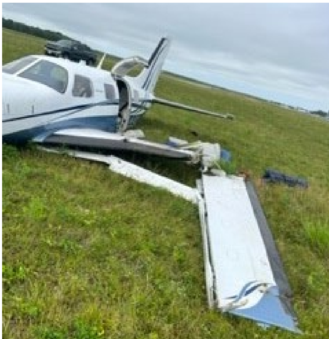
Photograph 4 - View of fractured left wing (Courtesy of MVY Airport Manager)
