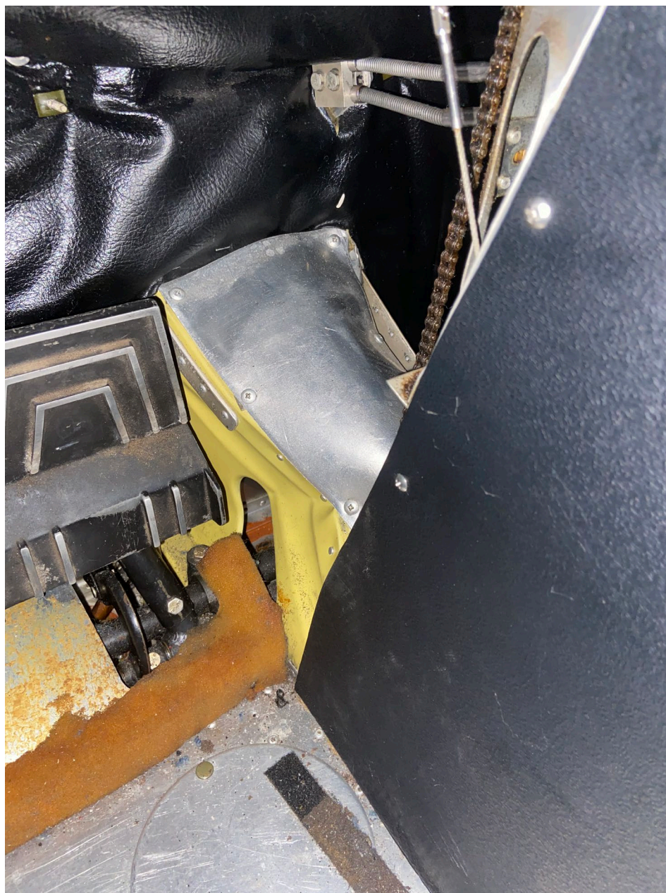
Photo 1 – FAA Digital Photograph. View of the Cockpit Showing the Structural Damage near the Pilot's Right Rudder Pedal
