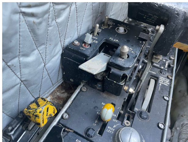
Flaps and Flap Switch discovered in the UP position
