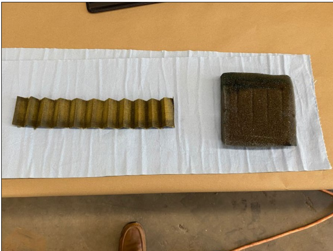
Photo 6: View of the engine filters (Photo Courtesy of FAA)
