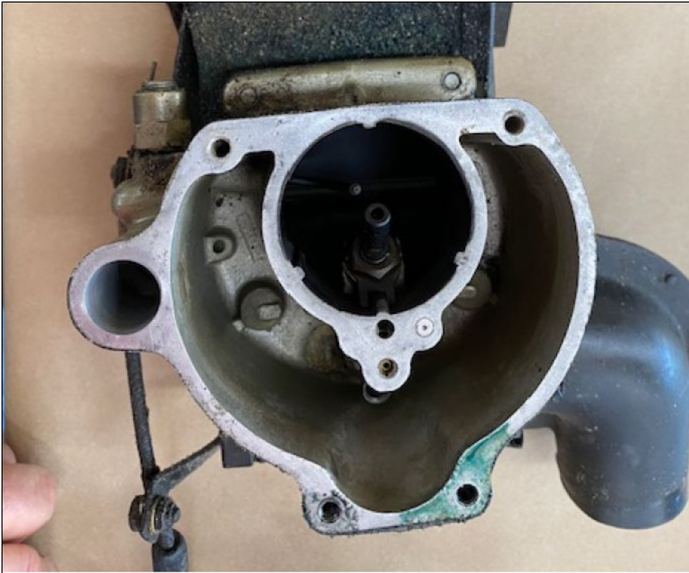
Photo 7: View of the partially disassembled carburetor (Photo Courtesy of FAA)
