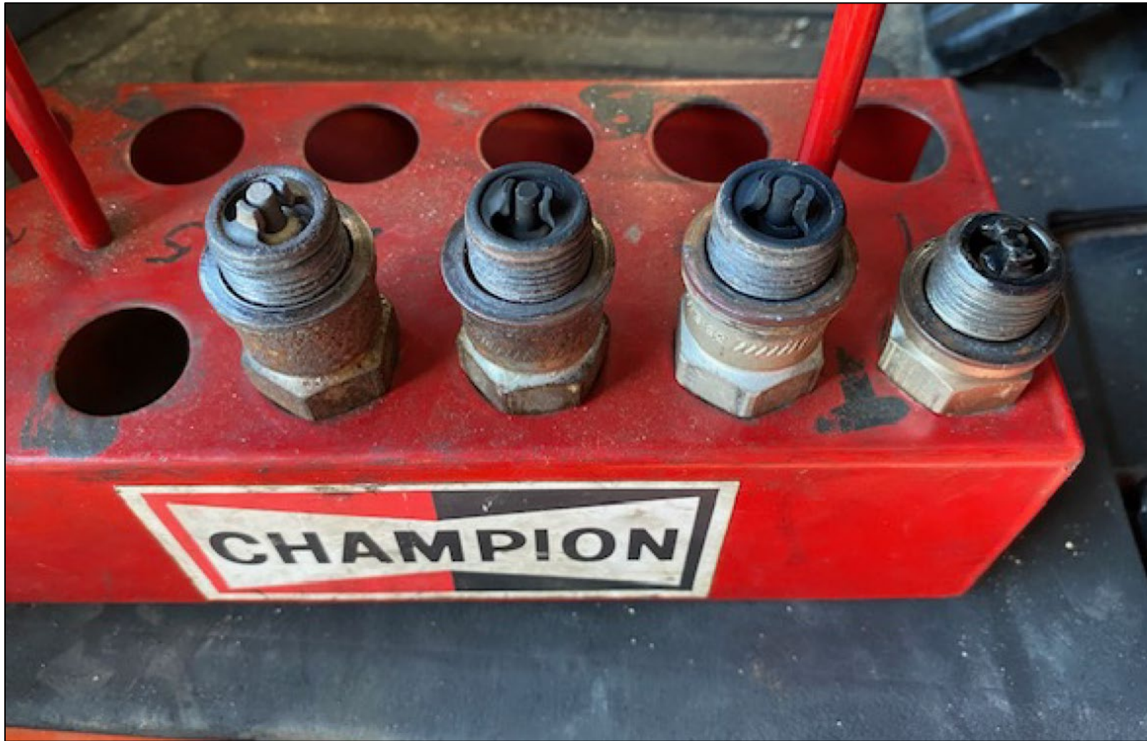
Photo 5: View of the top spark plugs (Photo Courtesy of FAA)
