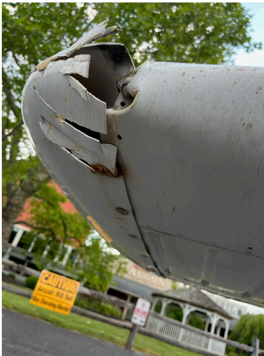
Photograph 1 - Right-Side Tip of Stabilator - Courtesy of FAA
