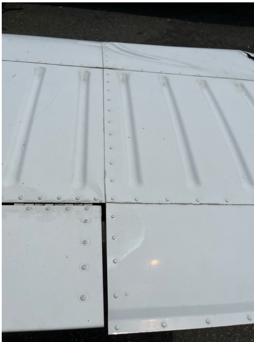
Photograph 4 - Top of Outboard Portion of Right-Side of Stabilator - Courtesy of FAA
