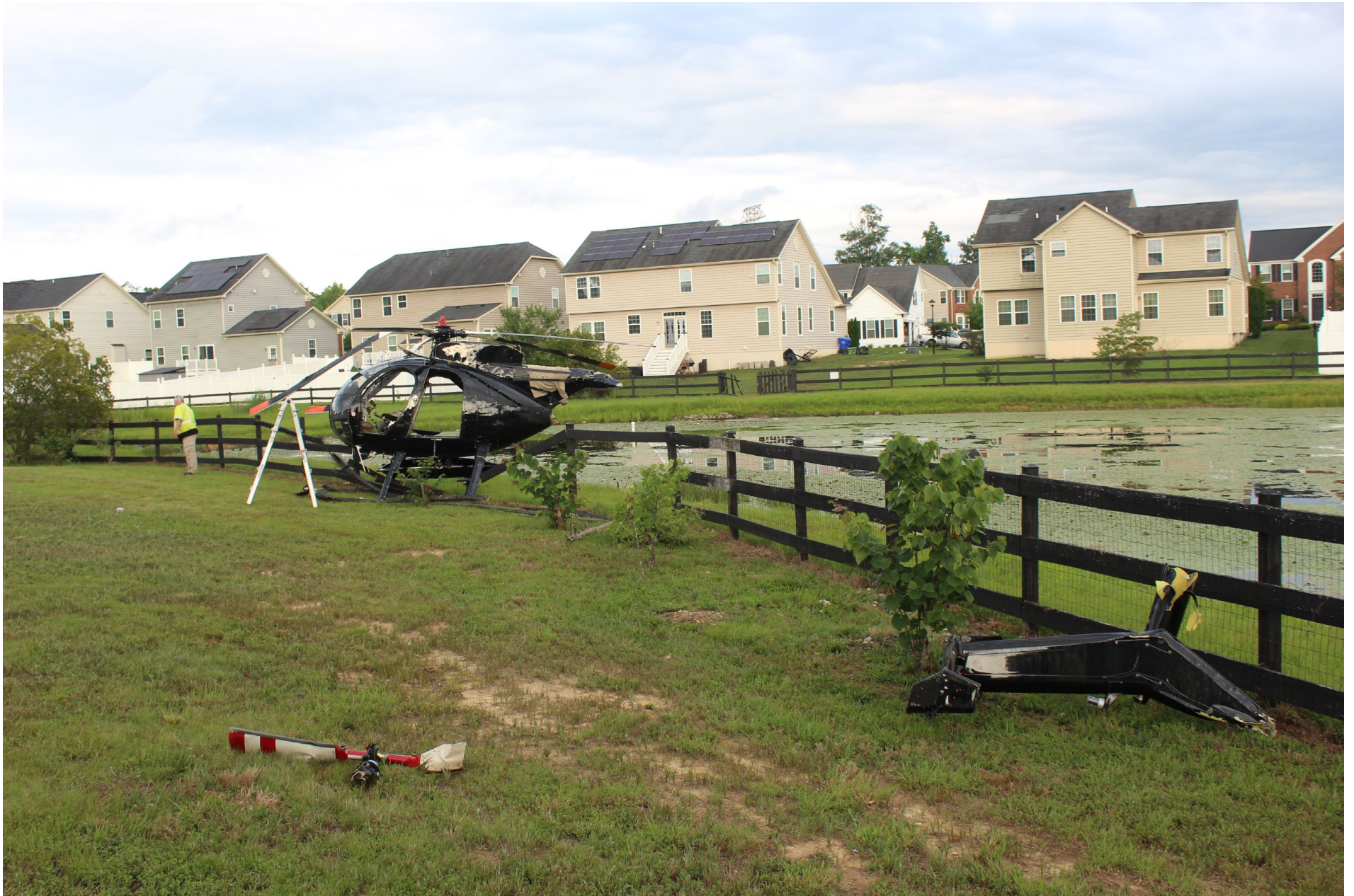
Photo 2 - View of Main Wreckage with Separated Tail and Tailrotor Gearbox and Tailrotor Assembly in Foreground. (AAR)
