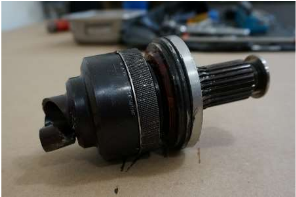
Figure 2. The accident overrunning clutch subassembly.
