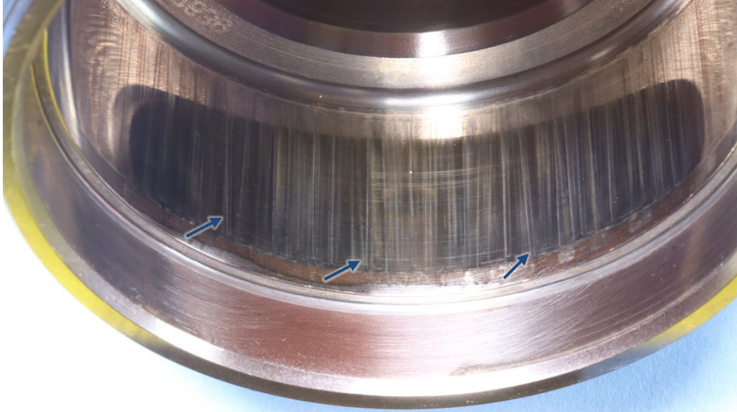
Figure 9. Sprag element contact marks on the clutch outer race. Unlabeled arrows point to several off-axis sprag element contact marks.
