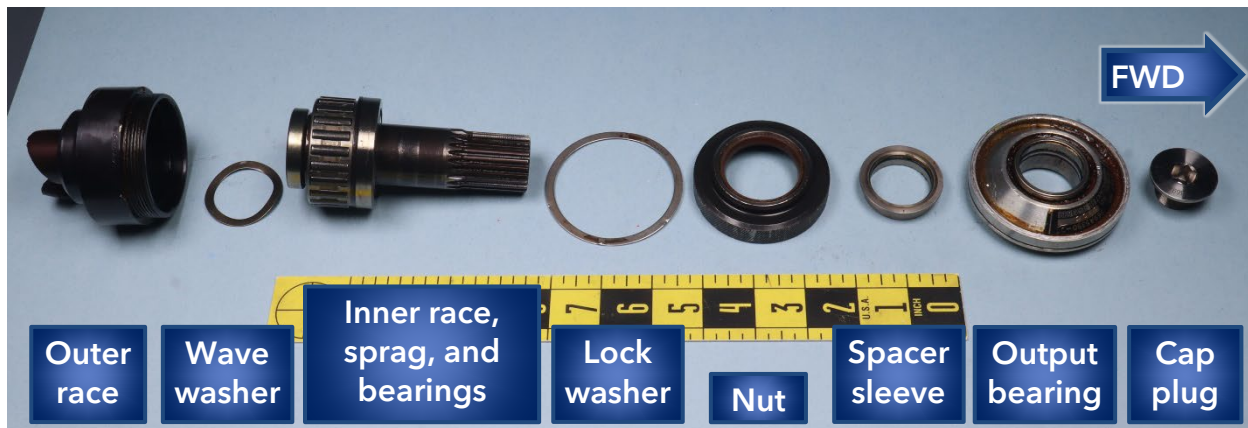
Figure 7. Disassembled pieces of the overrunning clutch subassembly.
