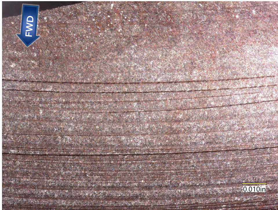
Figure 5. Intact fillet radius between the input shaft and adjacent shoulder on the clutch outer race forward of the spiral portion of the fracture.
