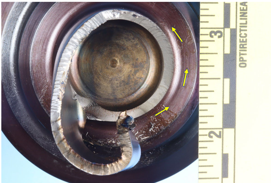
Figure 2. Visible portion of the forward side of the fracture surface in the clutch outer race. Unlabeled arrows next to the fracture surface indicate the direction of fatigue propagation on the spiral portion of the fracture.
