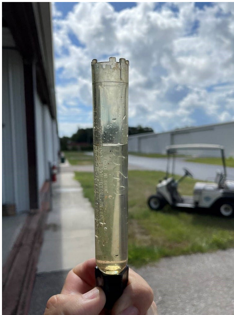
Photo 2 – Water Drained from Right Wing Fuel Tank (FAA)
