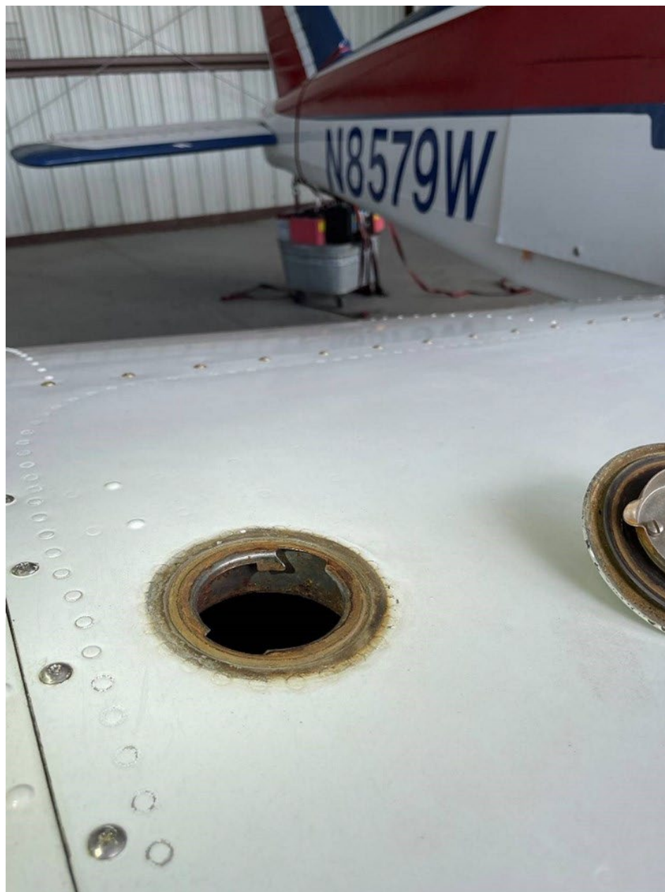
Photo 3 – Right Wing Fuel Tank with Corrosion (FAA)
