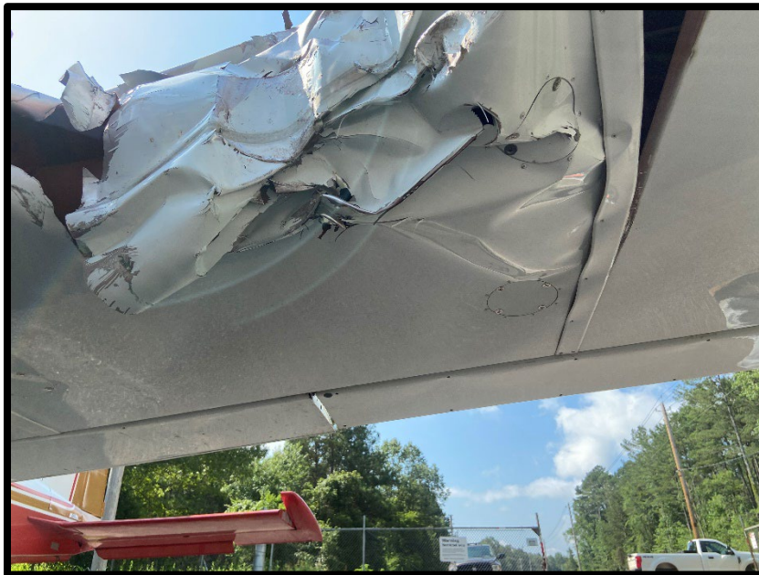
Figure 1: FAA Photograph. View Showing the span of Damage to the Left Wing Leading Edge.
