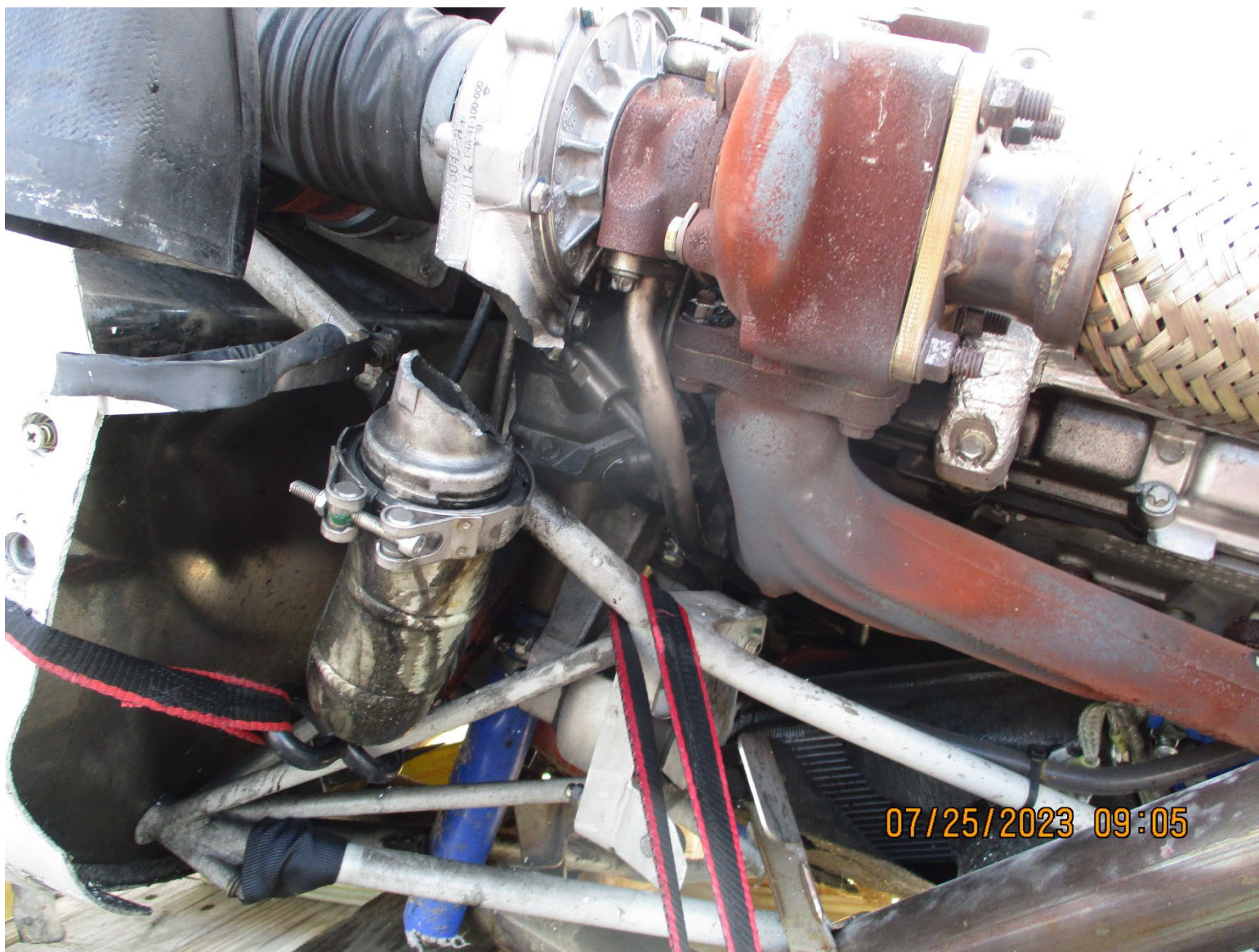
Photograph 3 - Turbo charger fractured.
