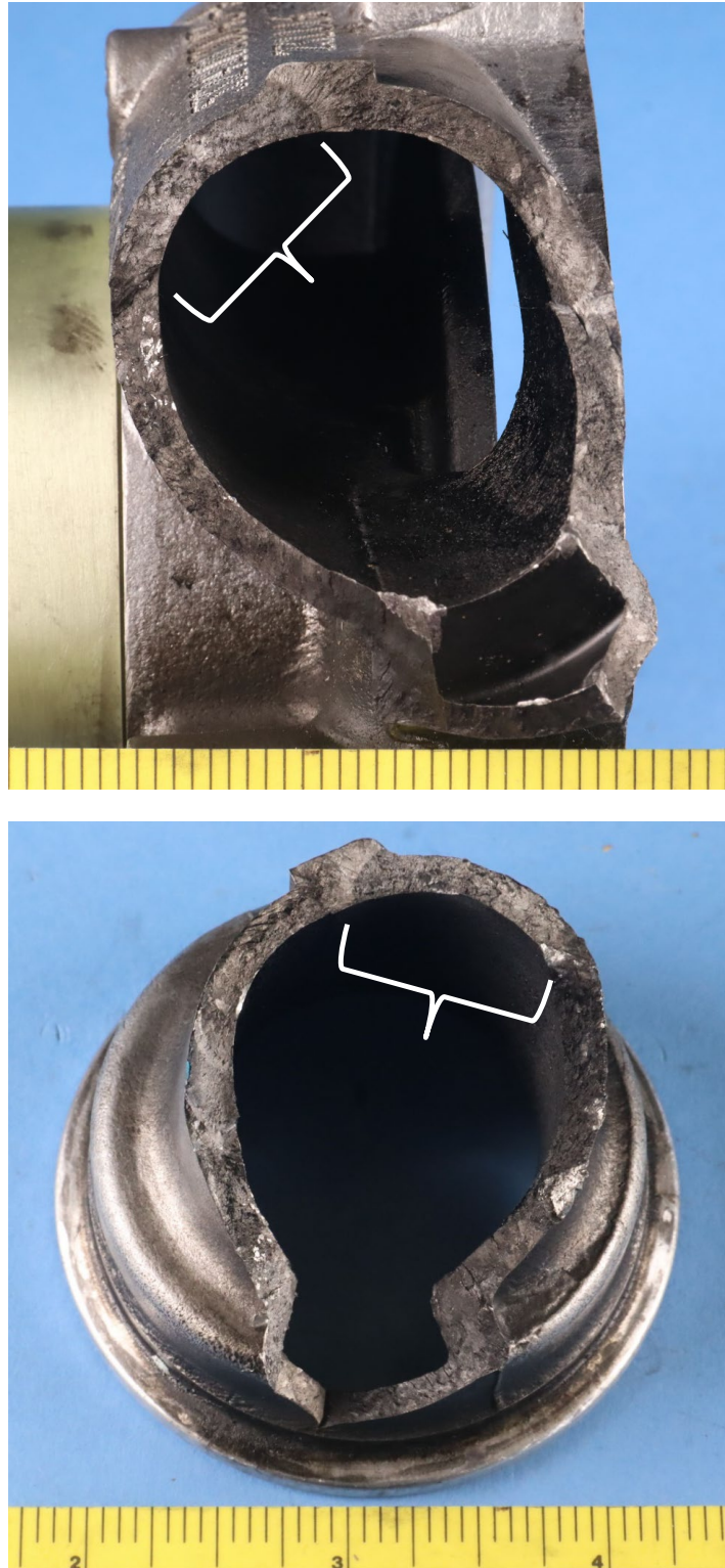
Figure 2. Close-up photos of the mating housing fracture surfaces with the straight portions indicated by white brackets.
