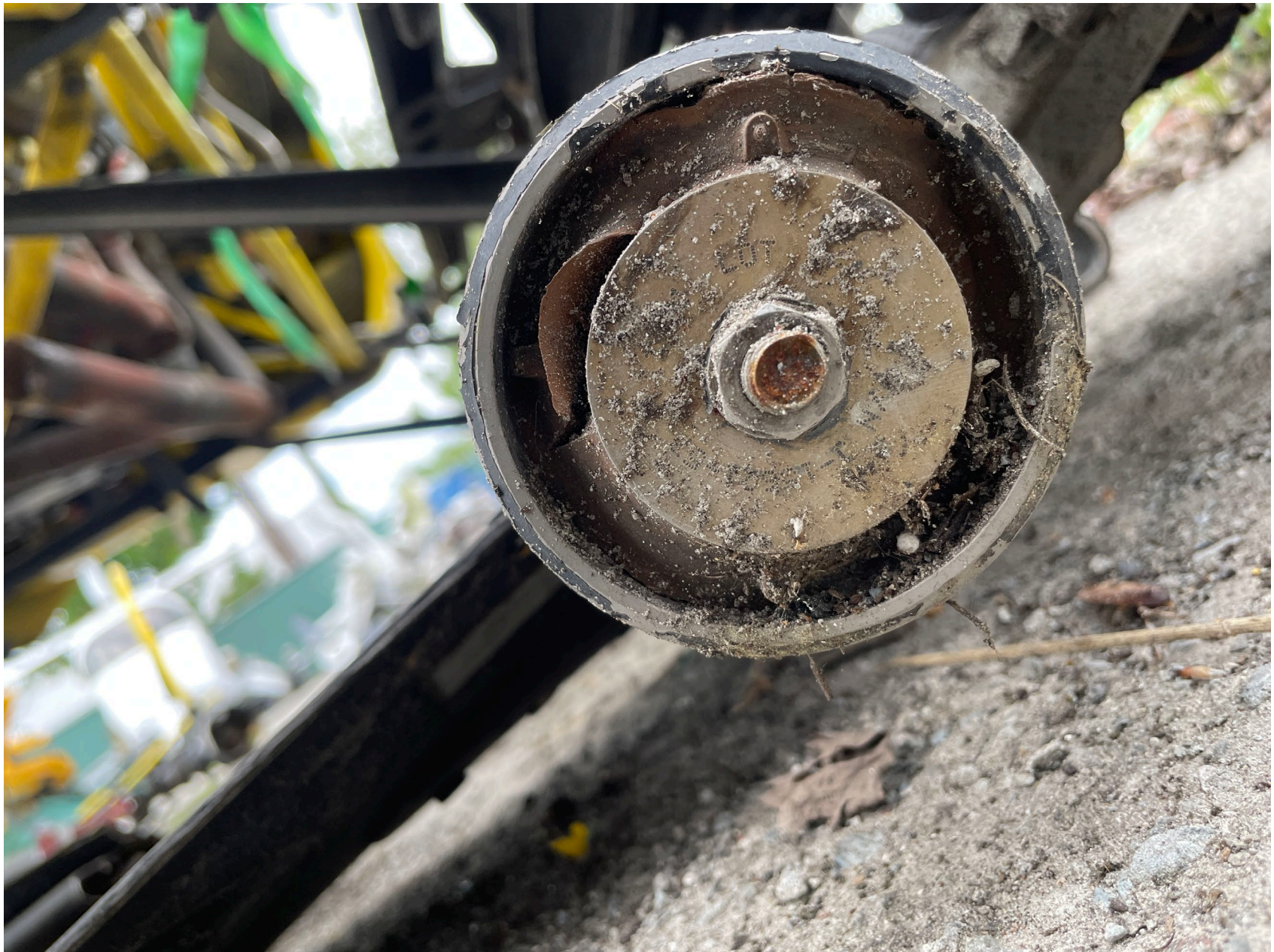
Photo 3 – View of Yellow M/R Blade Elastomeric Damper (FAA)
