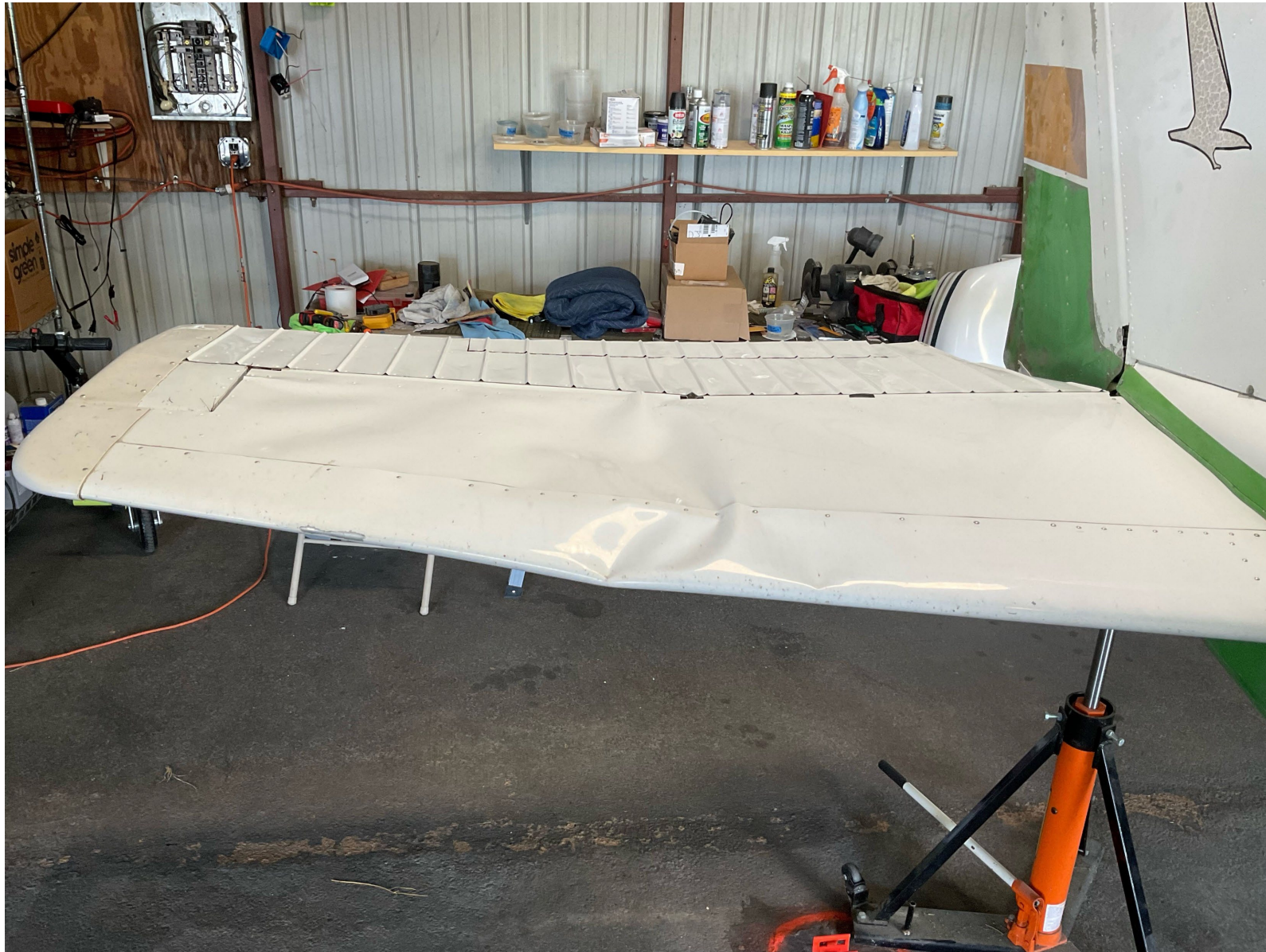
Photo 2: View of substantial damage to the right horizontal stabilizer (Photo Courtesy of FAA)
