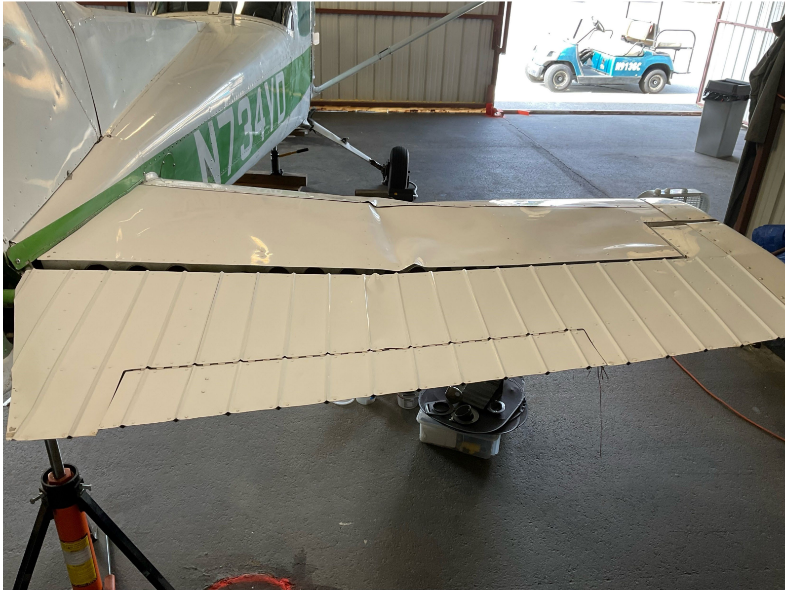
Photo 3: View of substantial damage to the right horizontal stabilizer (Photo Courtesy of FAA)
