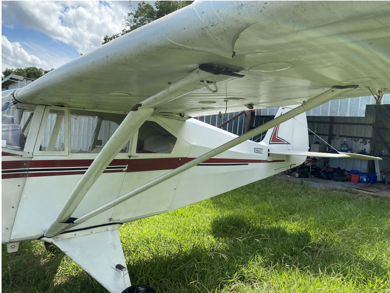
Photograph 1 - Damaged left wing strut. (Courtesy of FAA)
