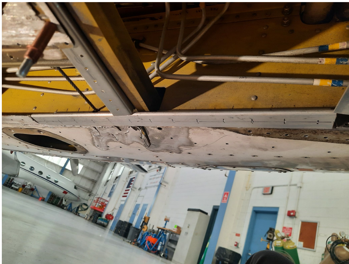
Figure 13 keelson web lower intercostals being repaired
