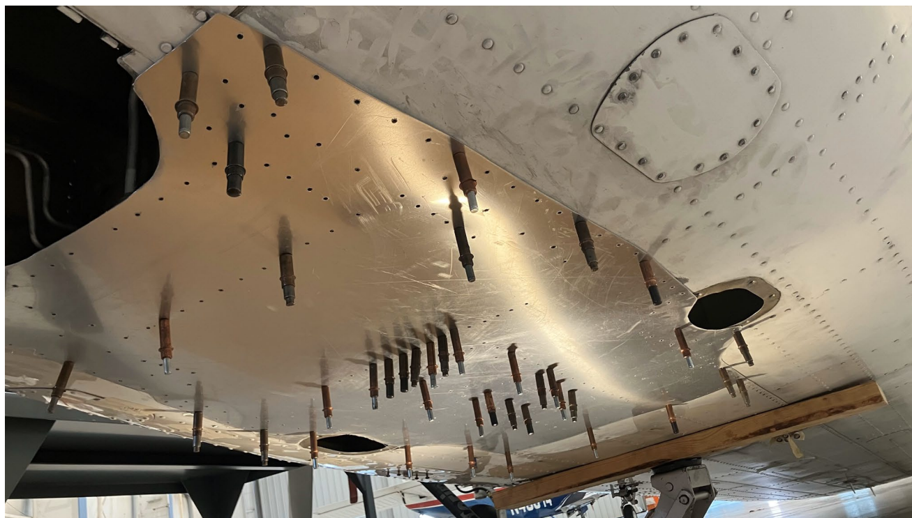
Figure 18 Skin doubler attach holes being located and picked up.
