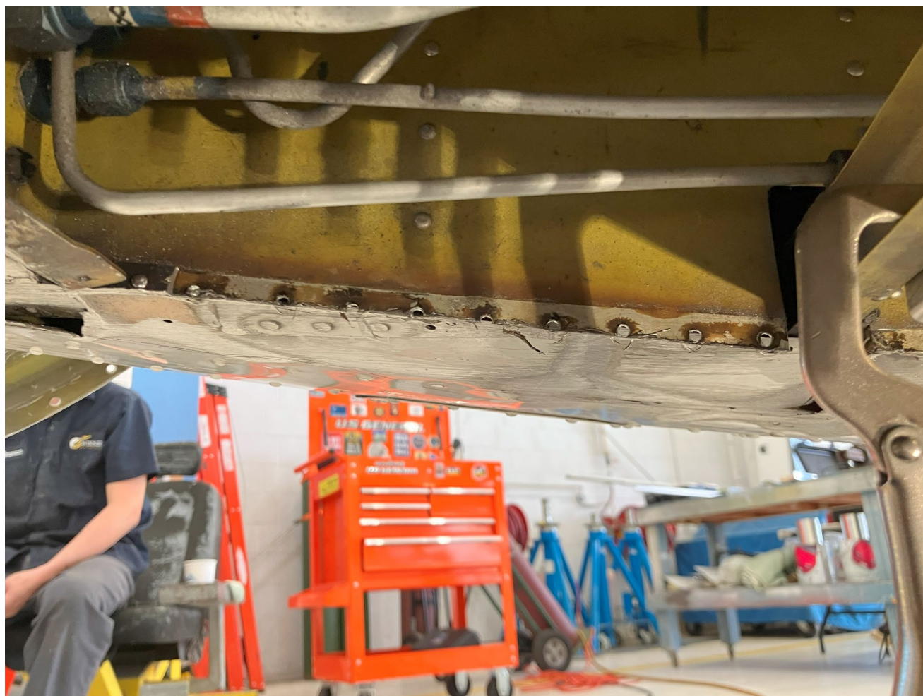
Figure 4 Chafed skin been trimmed out LH Side just fwd of FS23.5
