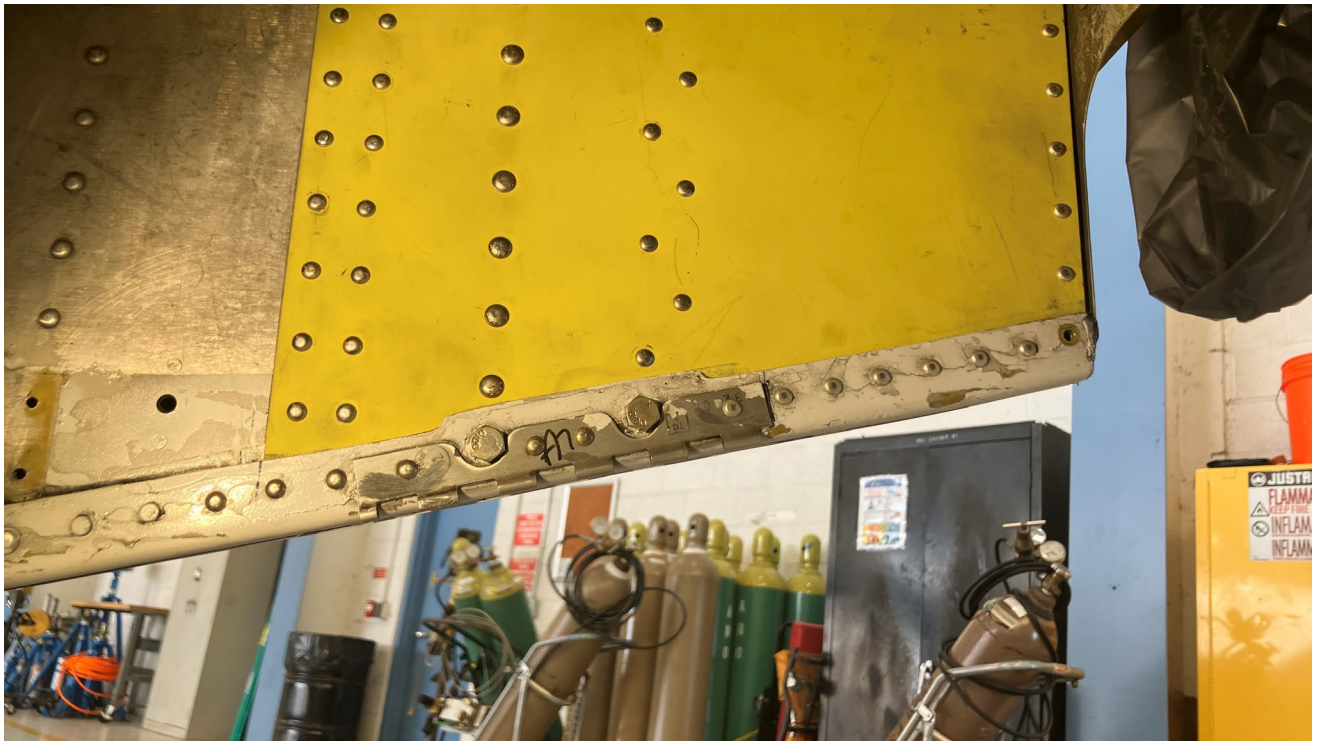
Figure 10 LH CK 159-2 being installed to keelson
