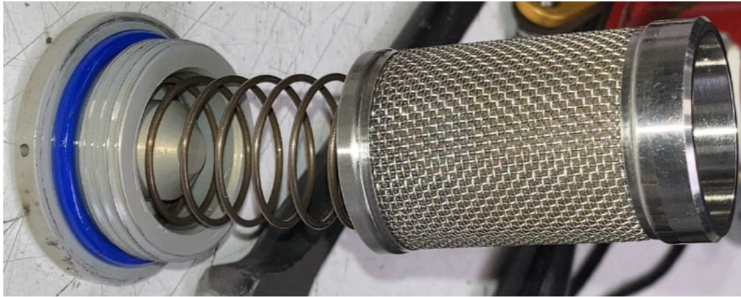
Photo No. 19, Fuel Pump Screen Filter
