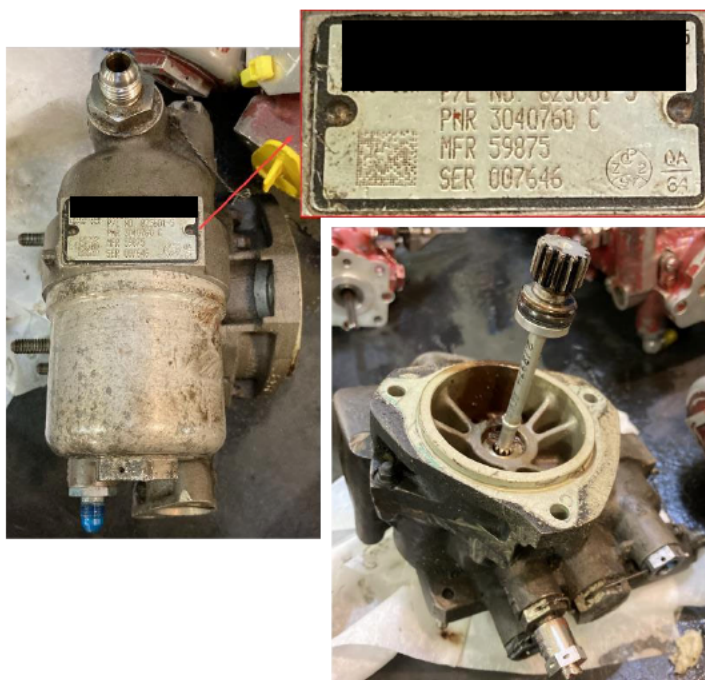
Photo No. 27, Fuel Pump Data Plate and Drive Shaft
