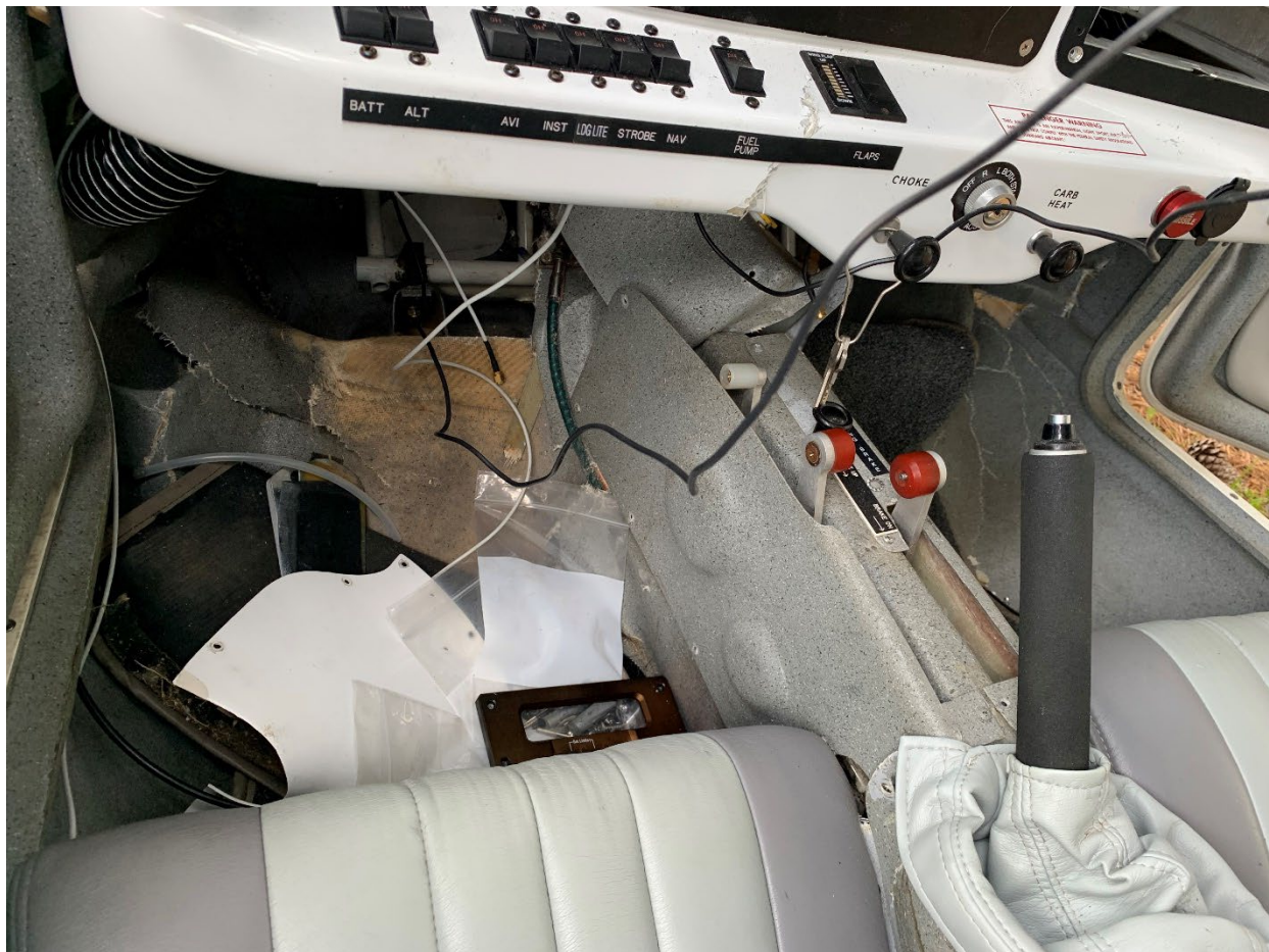
Photo6: View of the cockpit, note deformation of cockpit floor.
