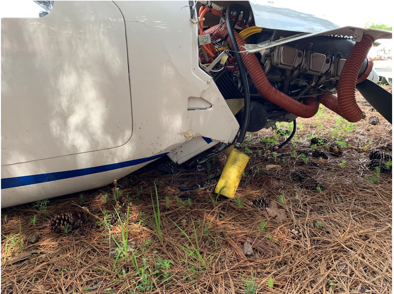
Photo 2: View of the forward fuselage crushed up and aft.
