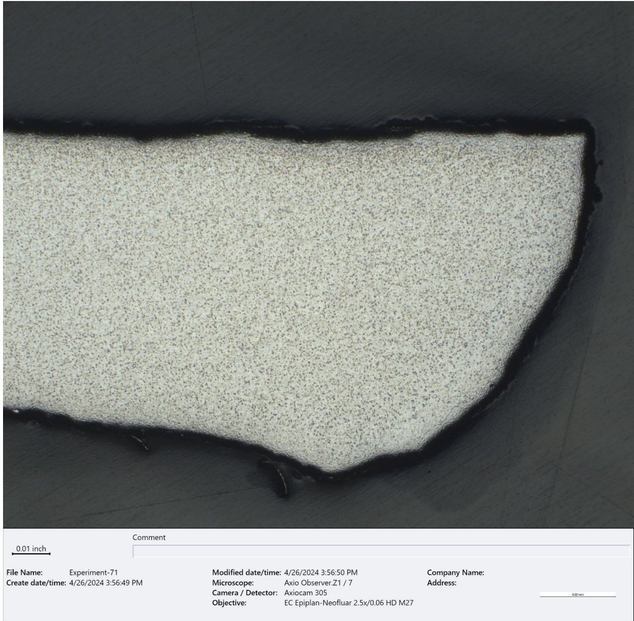
Figure 25. BF optical micrograph of the opposite side of the valve, in cross-section (~25X, etched Fry's Reagent).
