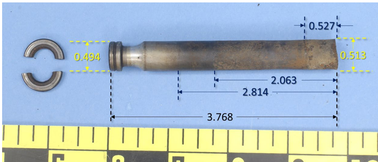
Figure 7. Closer view of the exhaust valve stem remnant and keepers.
