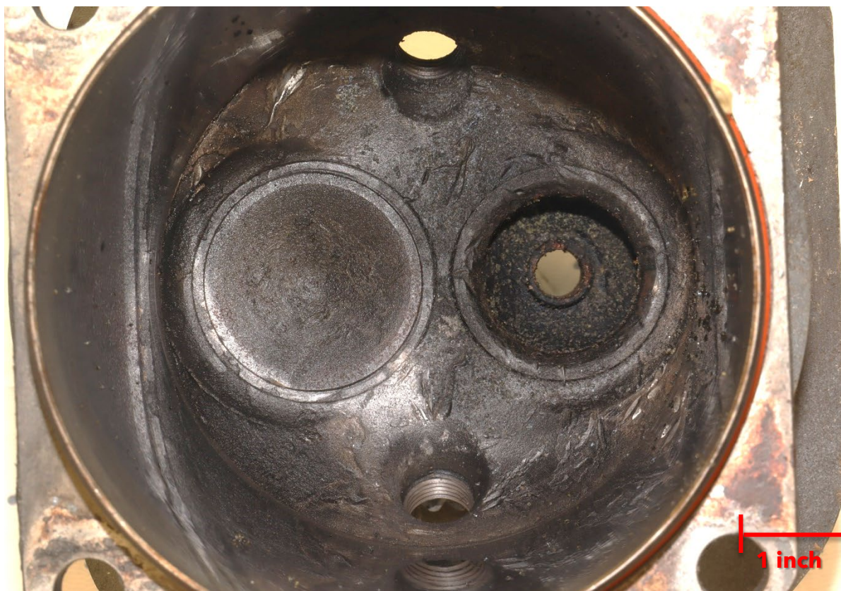
Figure 4. Closer view of the interior of the cylinder, showing impact damage to the cylinder and valve seat surfaces.
