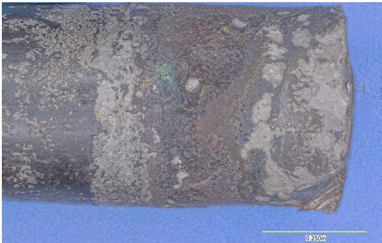
Figure 12. Side view of the valve near the fracture, after cleaning, rotated 90° from Figure 11.
