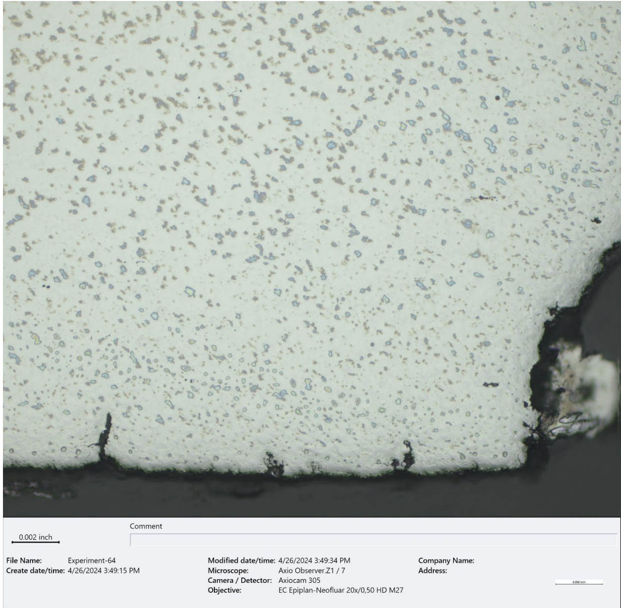
Figure 26. BF optical micrograph of a closer view of the exterior surface of the valve area in Figure 25, showing three surface cracks (~100X, etched Fry's Reagent)..
