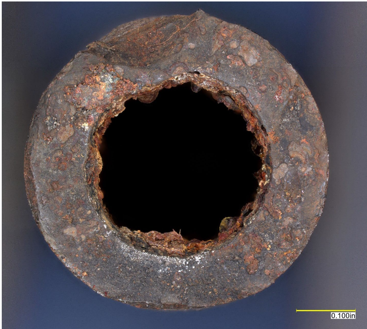
Figure 9. The exhaust valve stem fracture surface, as received.
