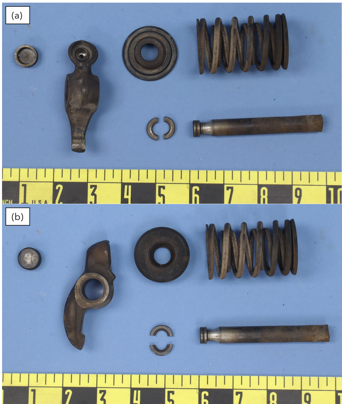
Figure 6. The disassembled rocker arm, retainer, keepers, springs, cap, and exhaust valve stem, from different sides.
