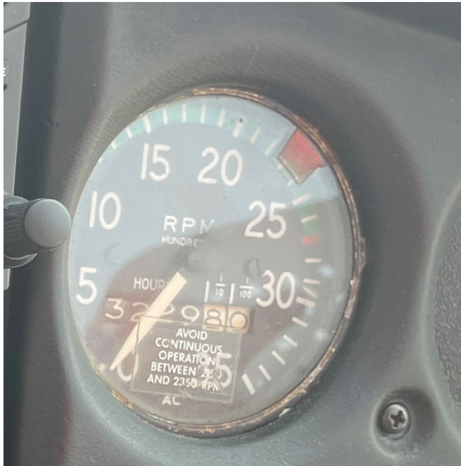
Figure 5: View of the Engine Tachometer Post Accident. Photograph Provided by the Insurance Adjuster.
