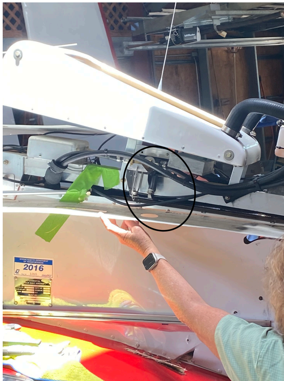
Photo 6 – View of Approximate Alignment of Witness Hole Access to Gascolator Bowl Mount (FAA)
