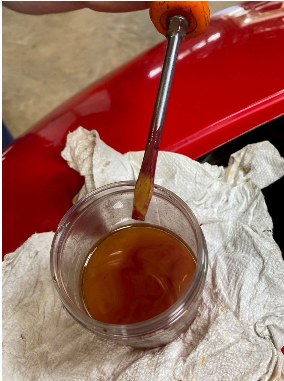
Photo 4 – View of Water Detection (Paste) Test of Gascolator Bowl Contents (FAA)
