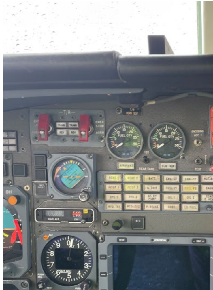
Photograph 10 - T/R Emergency Stow Switches as Found Prior to Aircraft Recovery
