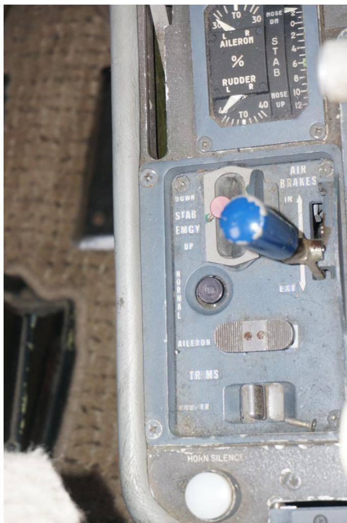
Photograph 12 - Air Brakes (Spoilers)
