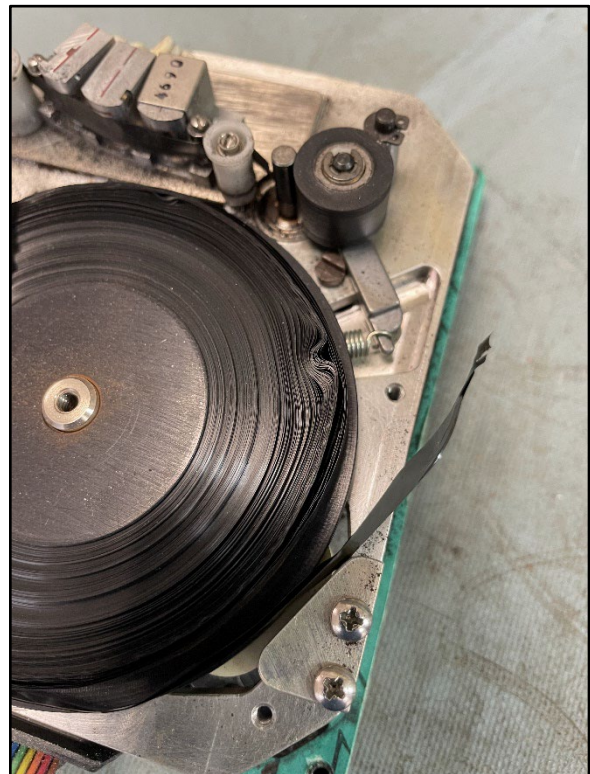
Figure 3. Magnetic tape with cover removed (left) and magnetic tape damage (right).
