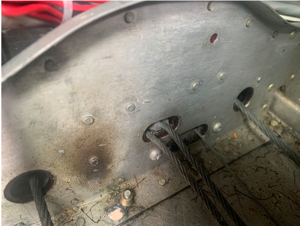
Photograph 3 - View of the bridle cable block against F.S. 179 (Courtesy of NTSB)
