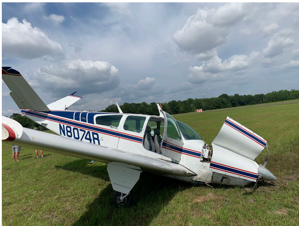
Photograph 1 - Blue and white accident airplane showing fuselage damage (Courtesy of FAA)
