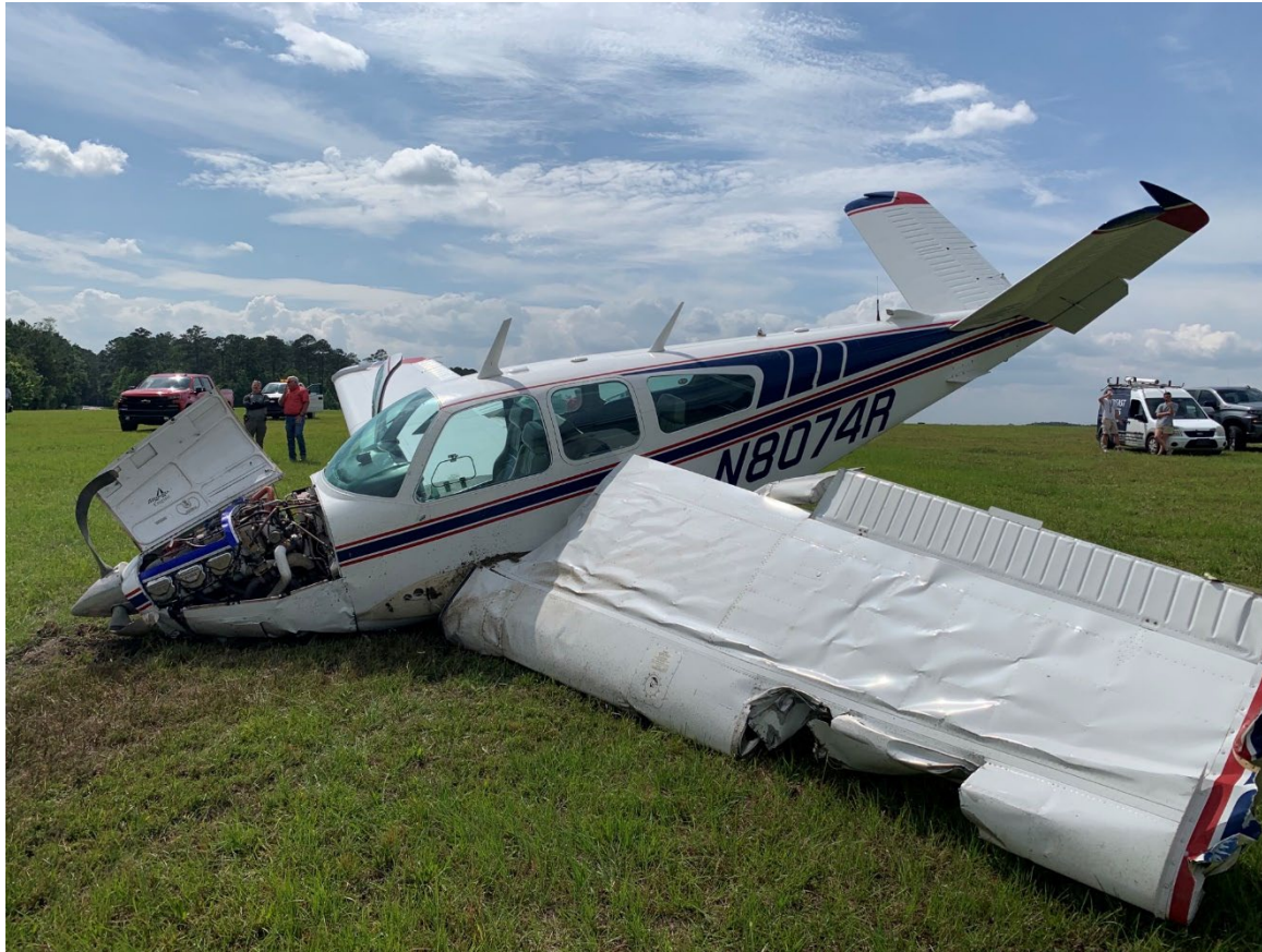
Photograph 2 - Left side of blue and white accident airplane showing left wing damage (Courtesy of FAA)
