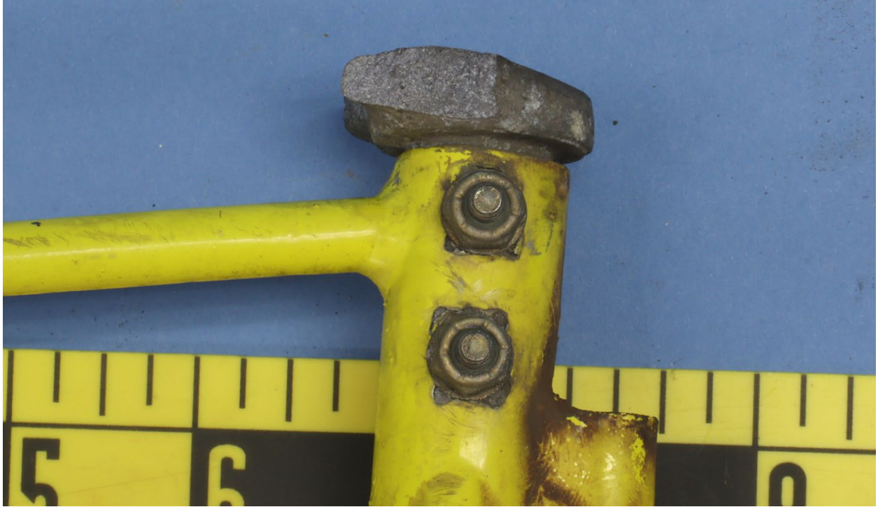
Figure 14. View of one of the fracture surfaces of the link casting.
