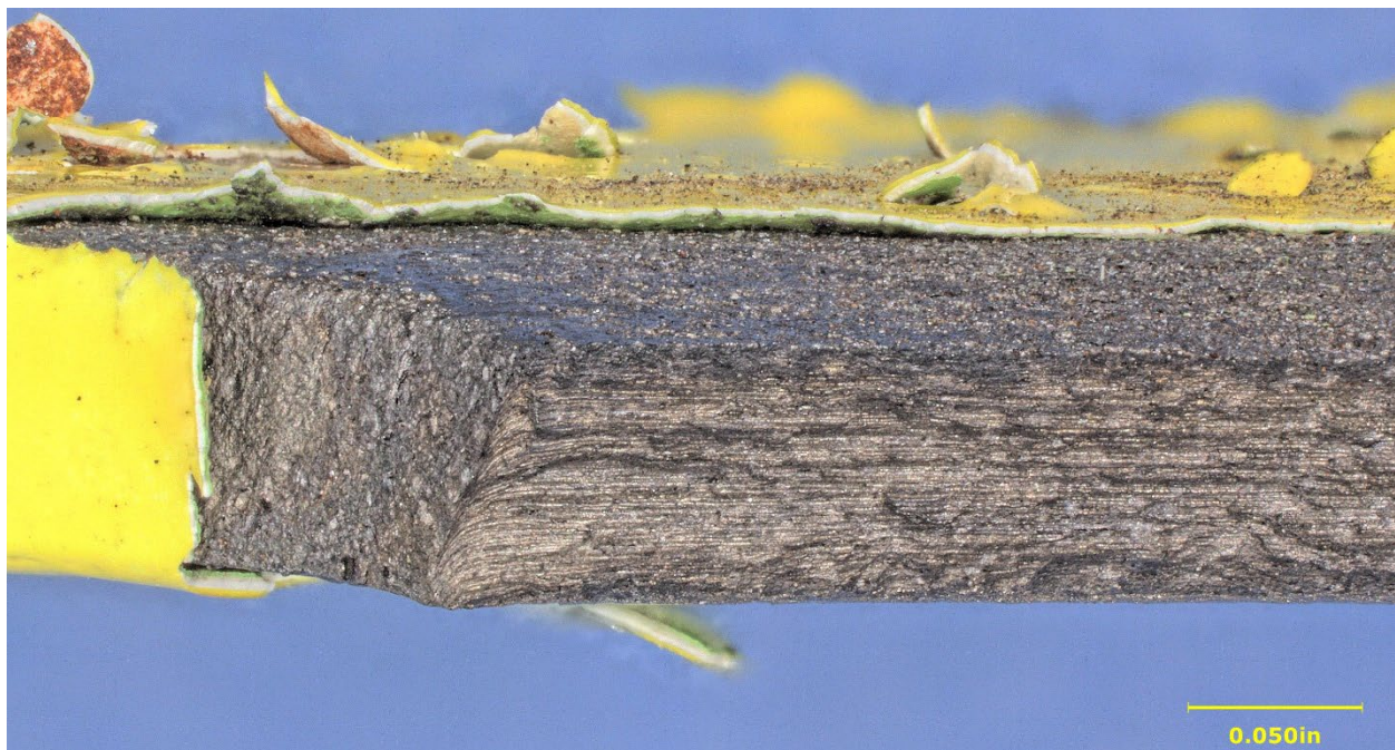
Figure 10. Fracture surface edge with the bore of the horn section in Figure 6.
