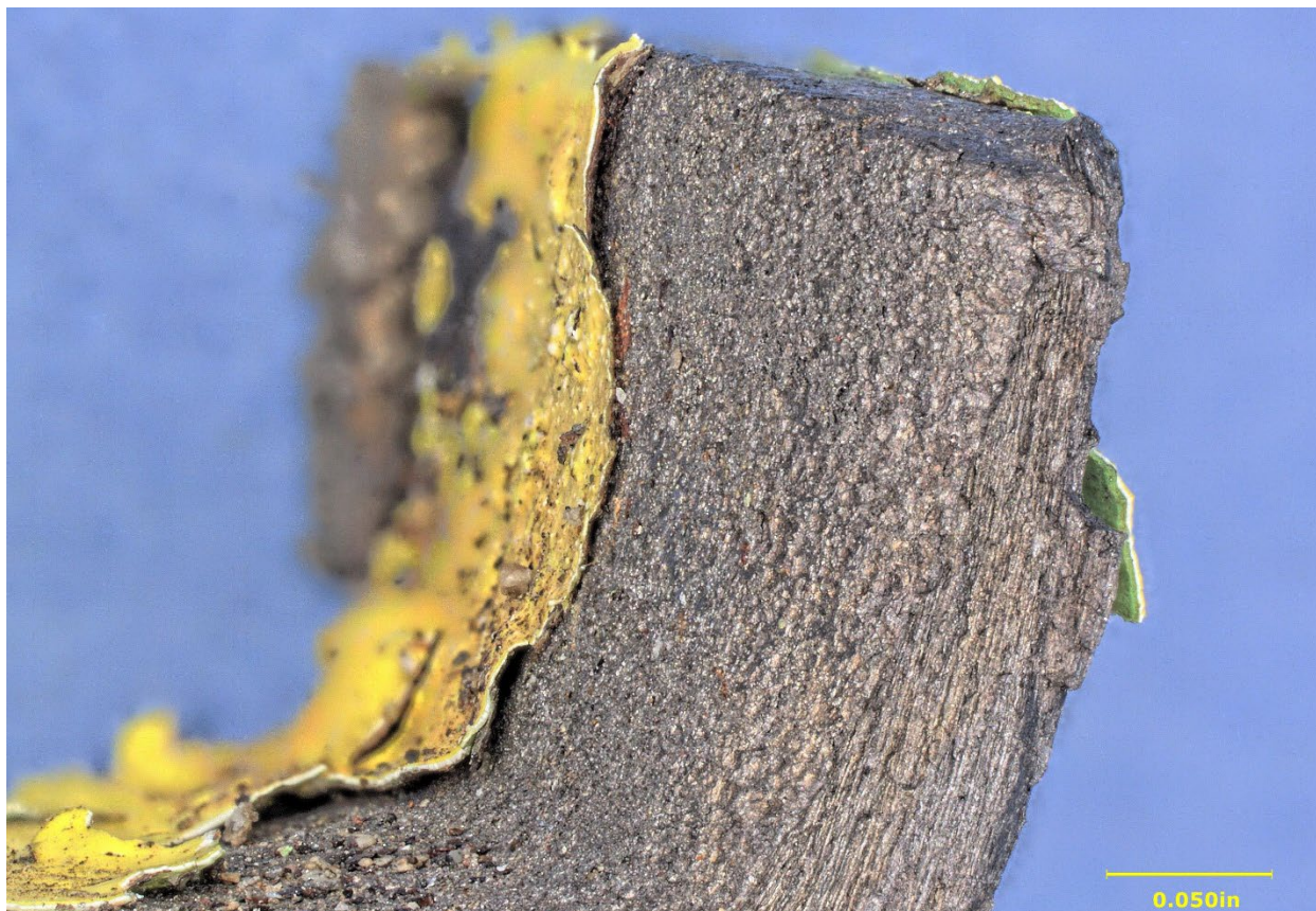
Figure 13. Opposite edge of the right fractured segment in Figure 6, showing thinning.
