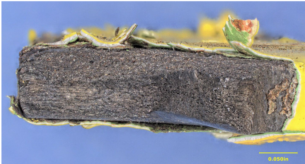
Figure 7. Closer view of the fractured segment of the horn to the left in Figure 6.
