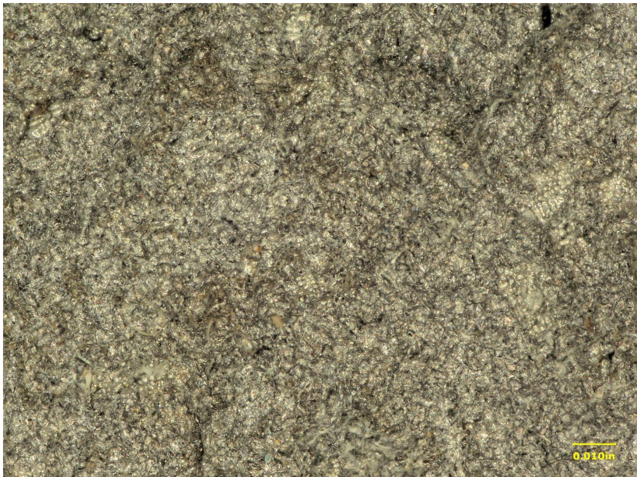
Figure 17. Typical area of the fracture surface in Figure 16.
