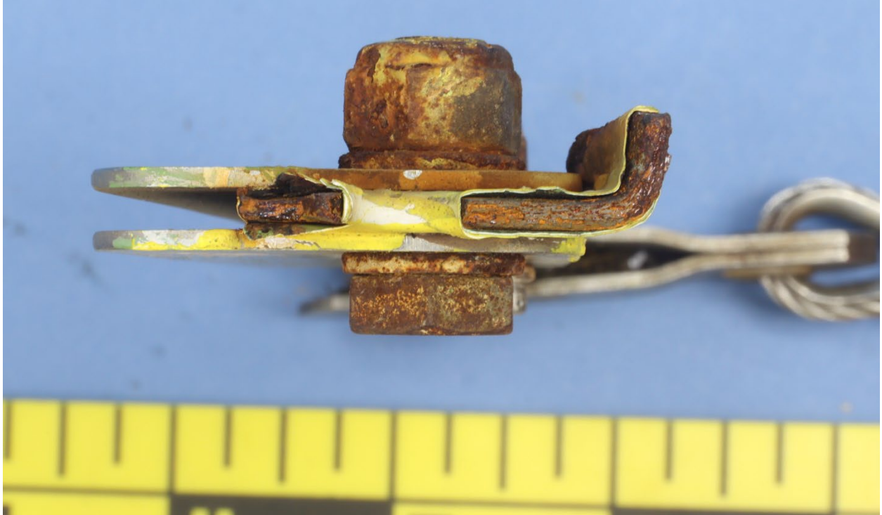
Figure 3. View of the outboard horn fracture still attached to the respective extension.
