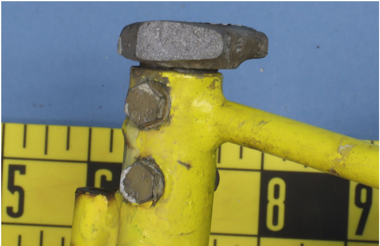
Figure 15. The opposite fracture surface from that shown in Figure 14.
