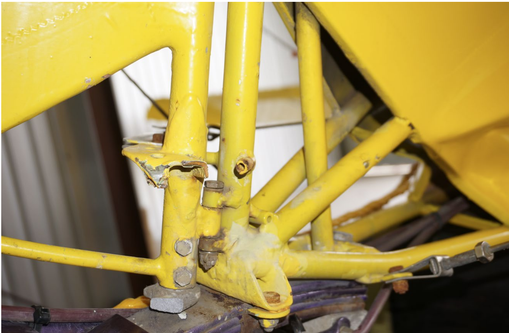
Photograph 8 - Close Up of Right Side of Lower Rudder Showing Fractured Rudder Horn
