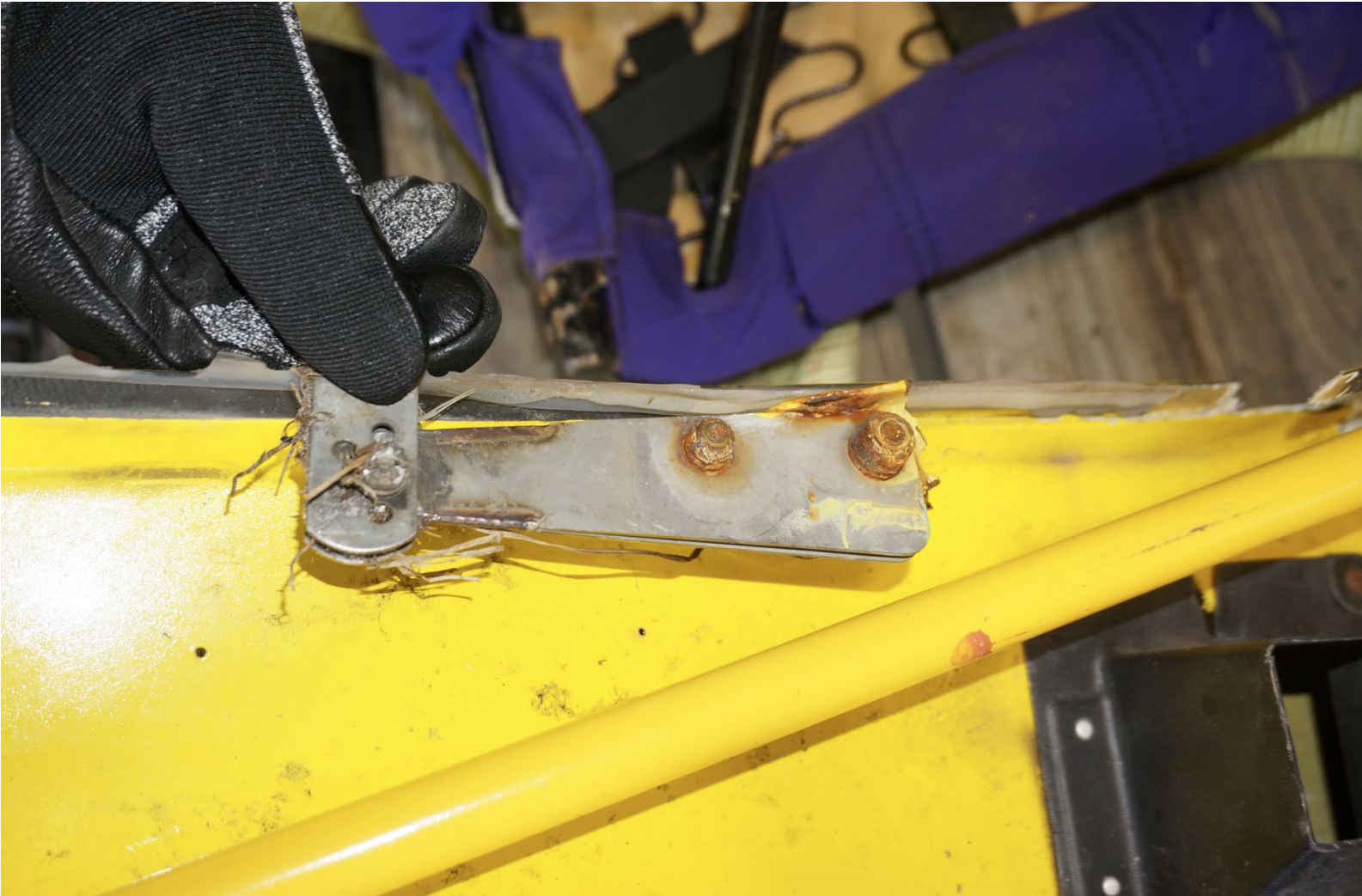
Photograph 12 - Bottom View of Broken Right Rudder Horn and Extension
