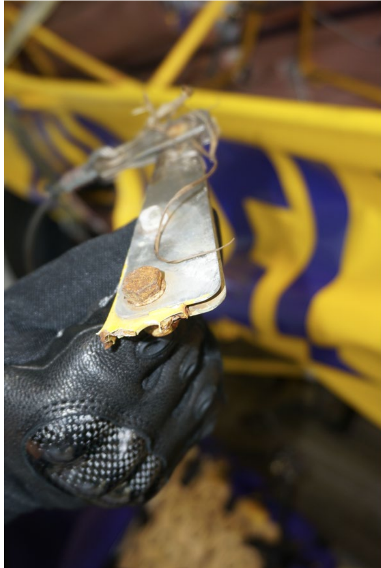
Photograph 9 - Broken Right Rudder Horn and Extension
