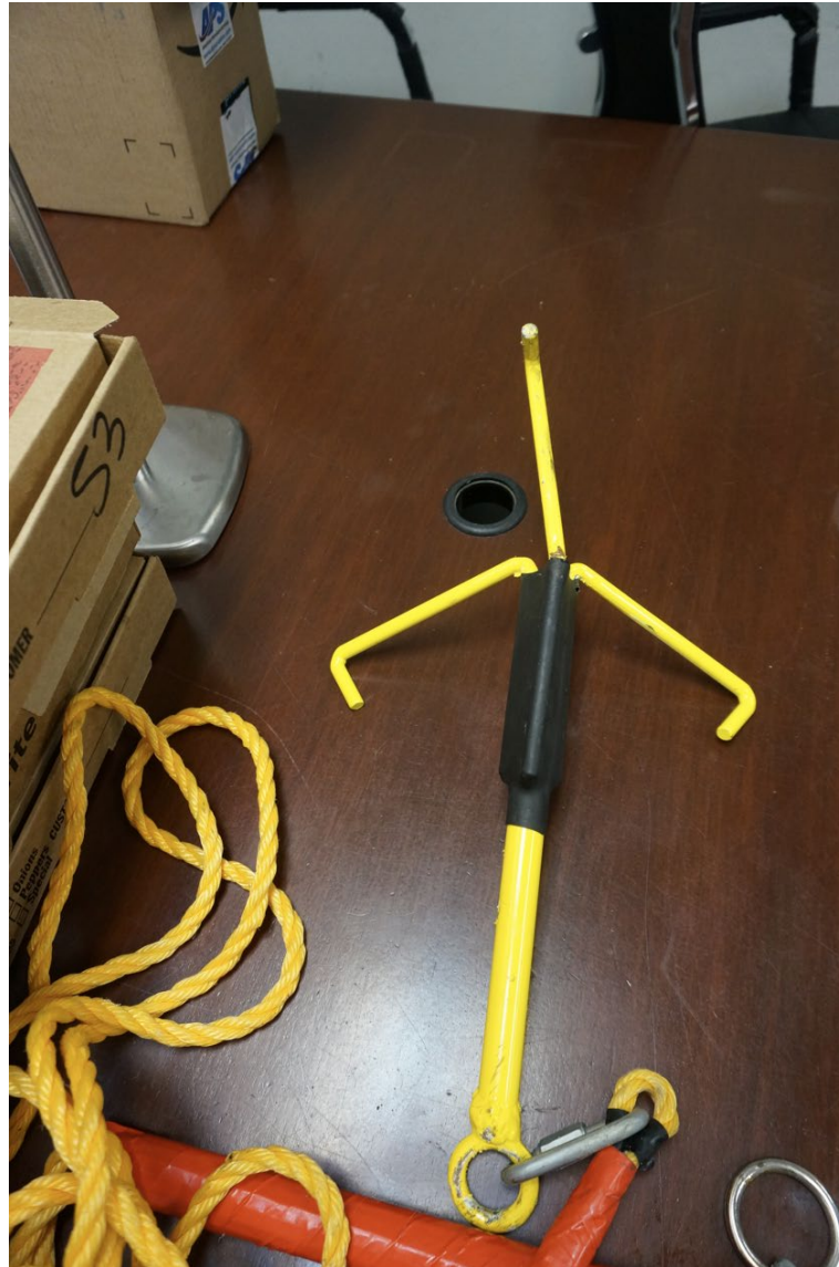
Photograph 13 - Tow Hook Displaying Bent Prong
