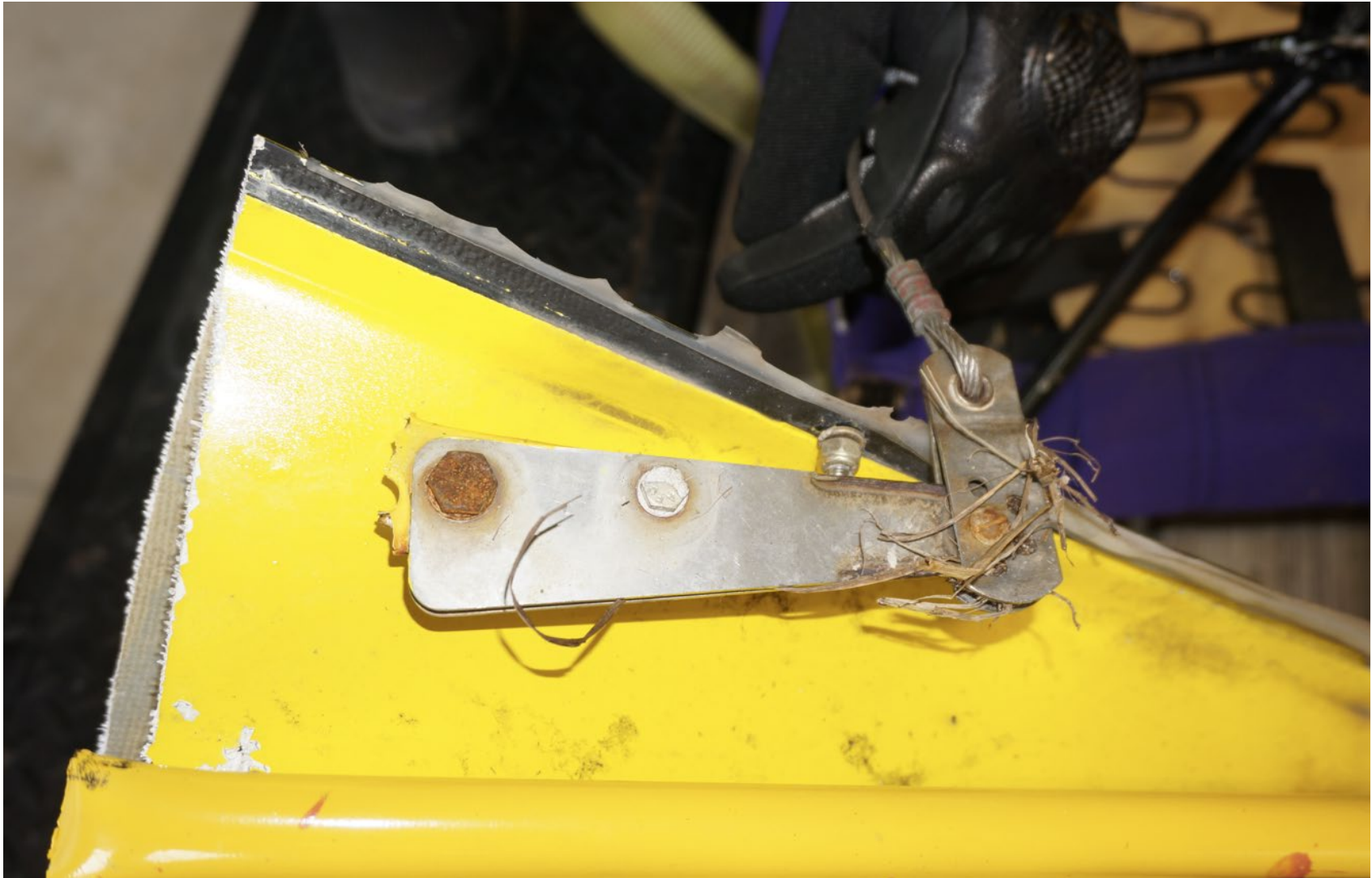
Photograph 10 - Top View of Broken Right Rudder Horn and Extension
