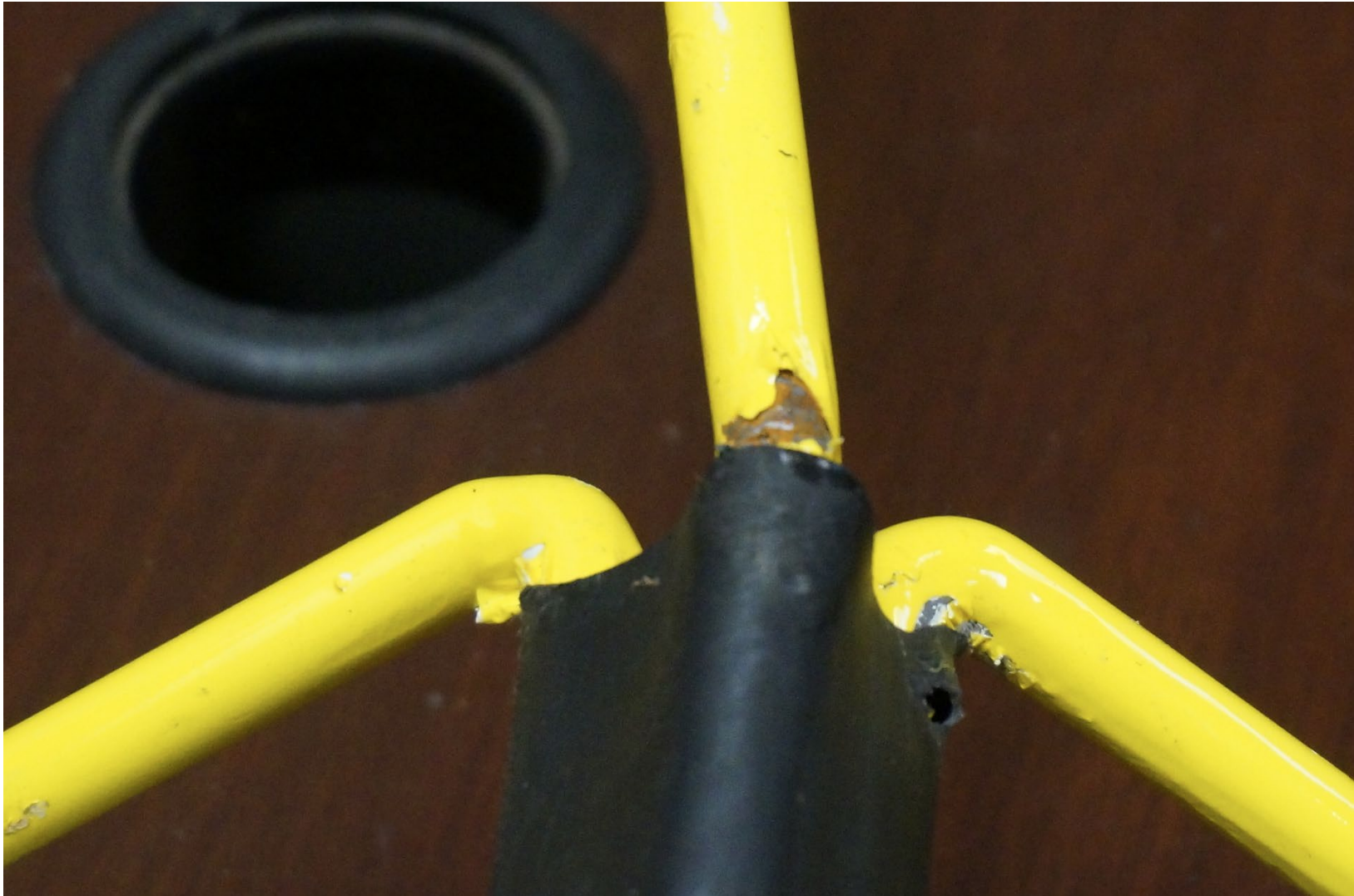
Photograph 15 - Close Up of Bend in Prong
