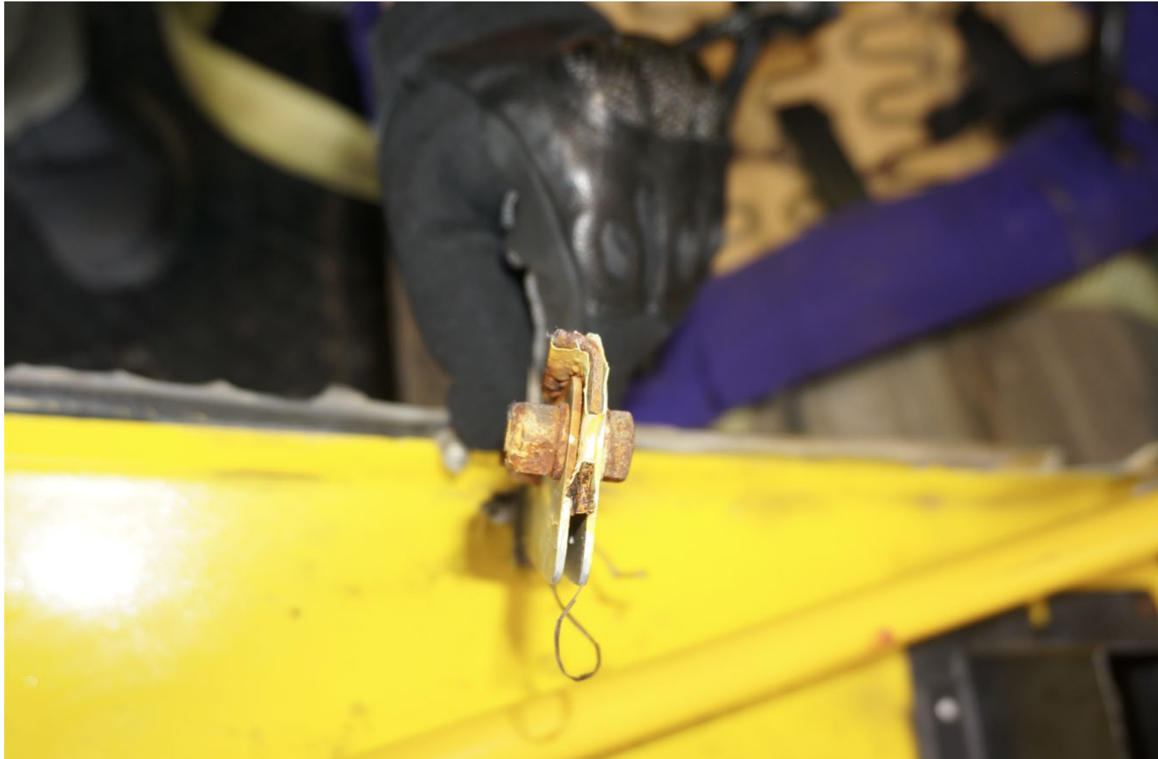
Photograph 11 - Fracture Face on Right Rudder Horn and Extension
