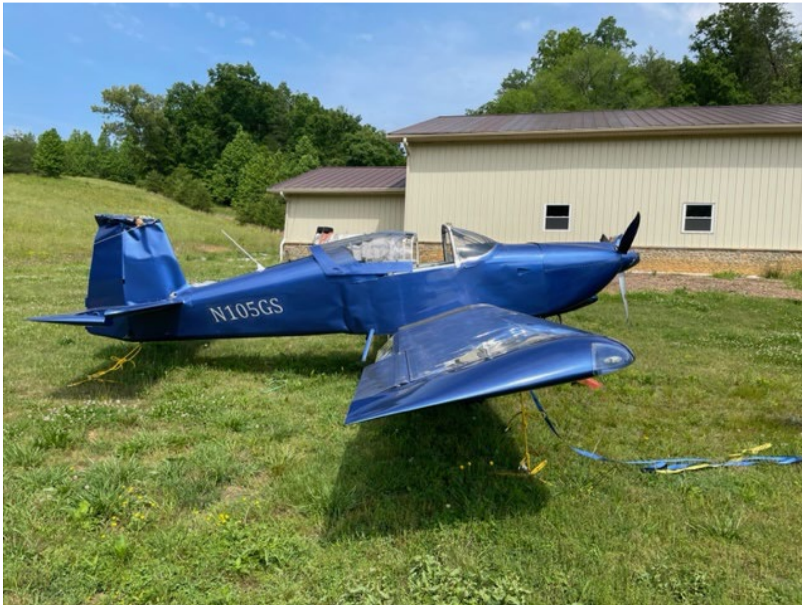
Photo 1: View of the airplane fuselage, vertical stabilizer and rudder damage (Photo Courtesy of FAA)
