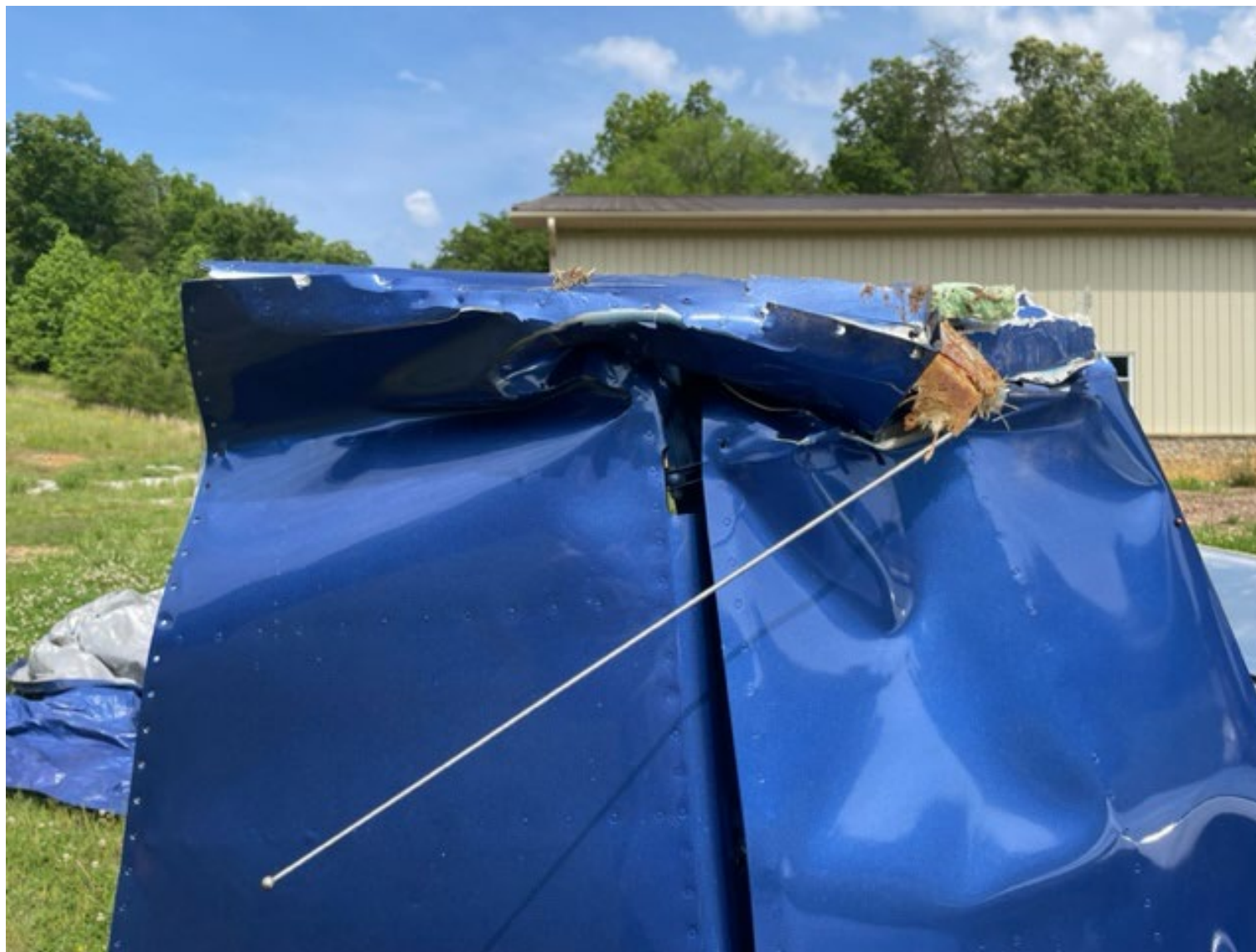
Photo 2: View of the damage to the vertical stabilizer and rudder (Photo Courtesy of FAA)
