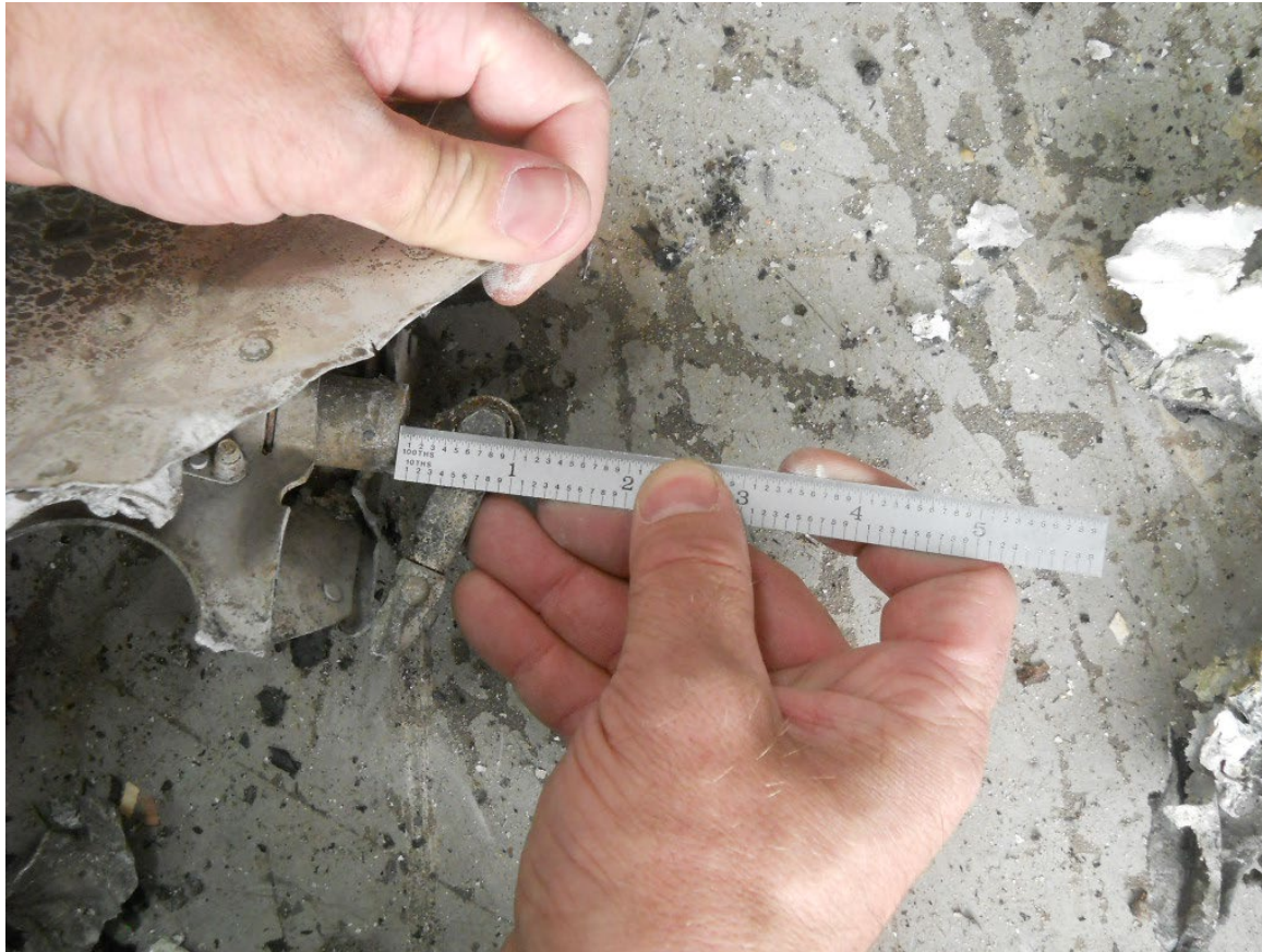
Photograph 4 - Elevator Trim Actuator Measurement
