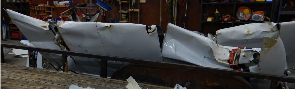
Photo 4 - View of underside of left wing showing leading edge impact damage before examination.
