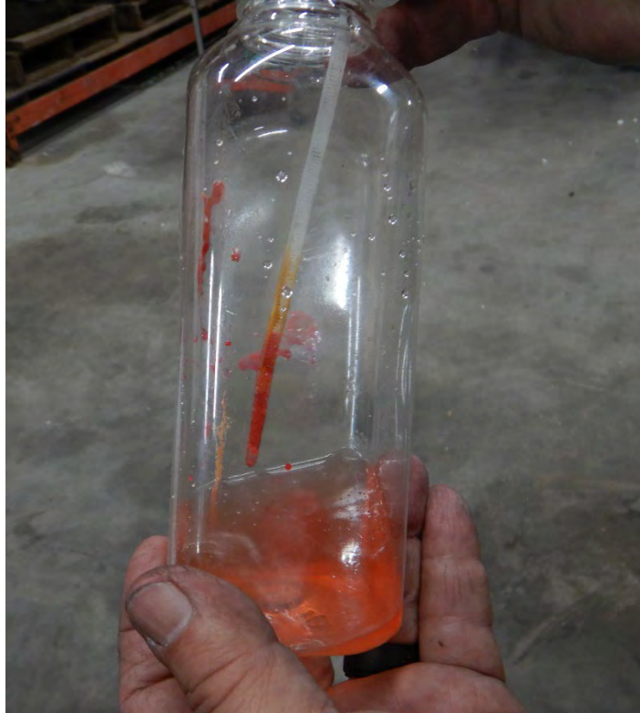
Photo 10 - Liquid drained from left wing fuel sump testing positive for water.
