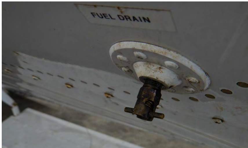
Photo 11 - Close-up view of right wing fuel sump in closed position.
