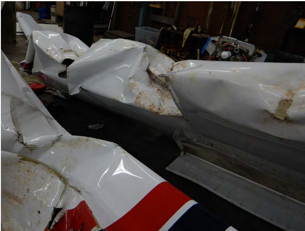
Photo 5 - View of right wing leading edge with impact damage prior to examination.
