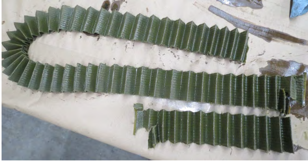
Photo 21 - Oil filter element after removal with no metallic debris.
