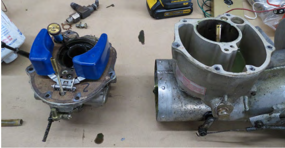
Photo 17 - Disassembled carburetor and floats (note no hydraulic deformation).
