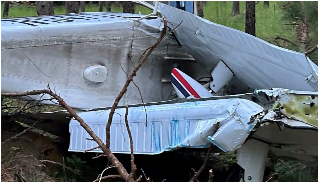
Photo 2 - Enlarged close-up view of fuel staining on left flap. (Photo courtesy of owner)
