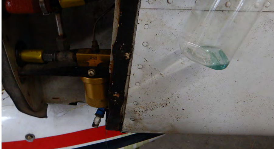
Photo 12 - View of fuel strainer bowl and sump drain with drained fluid.
