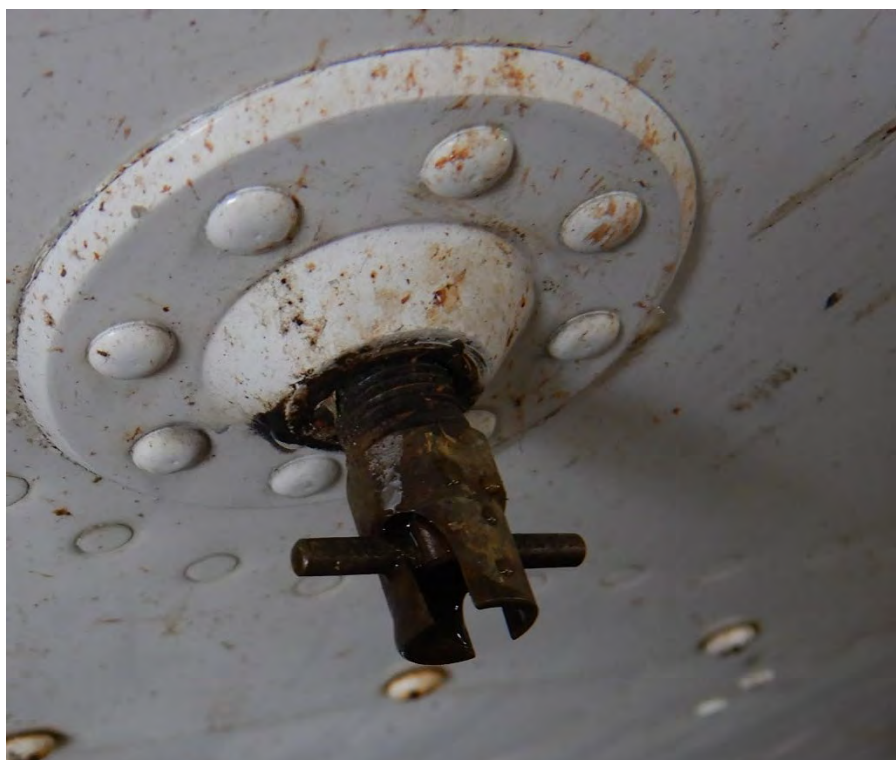
Photo 9 - Close-up view of left wing fuel sump in open and locked position.
