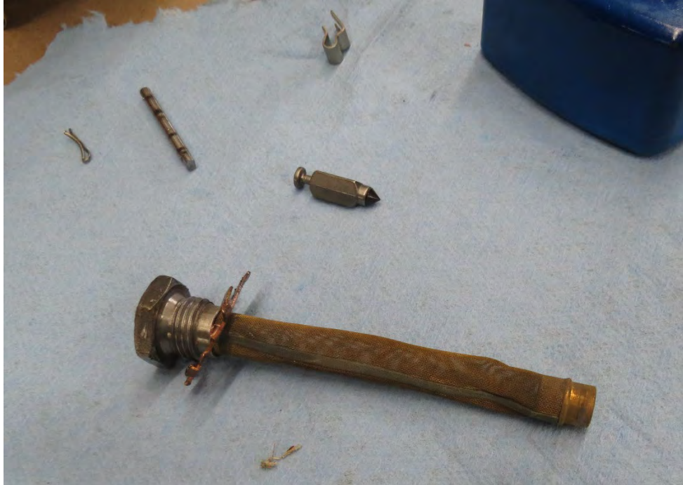
Photo 19 - Disassembled carburetor parts including fuel inlet screen (free from debris).
