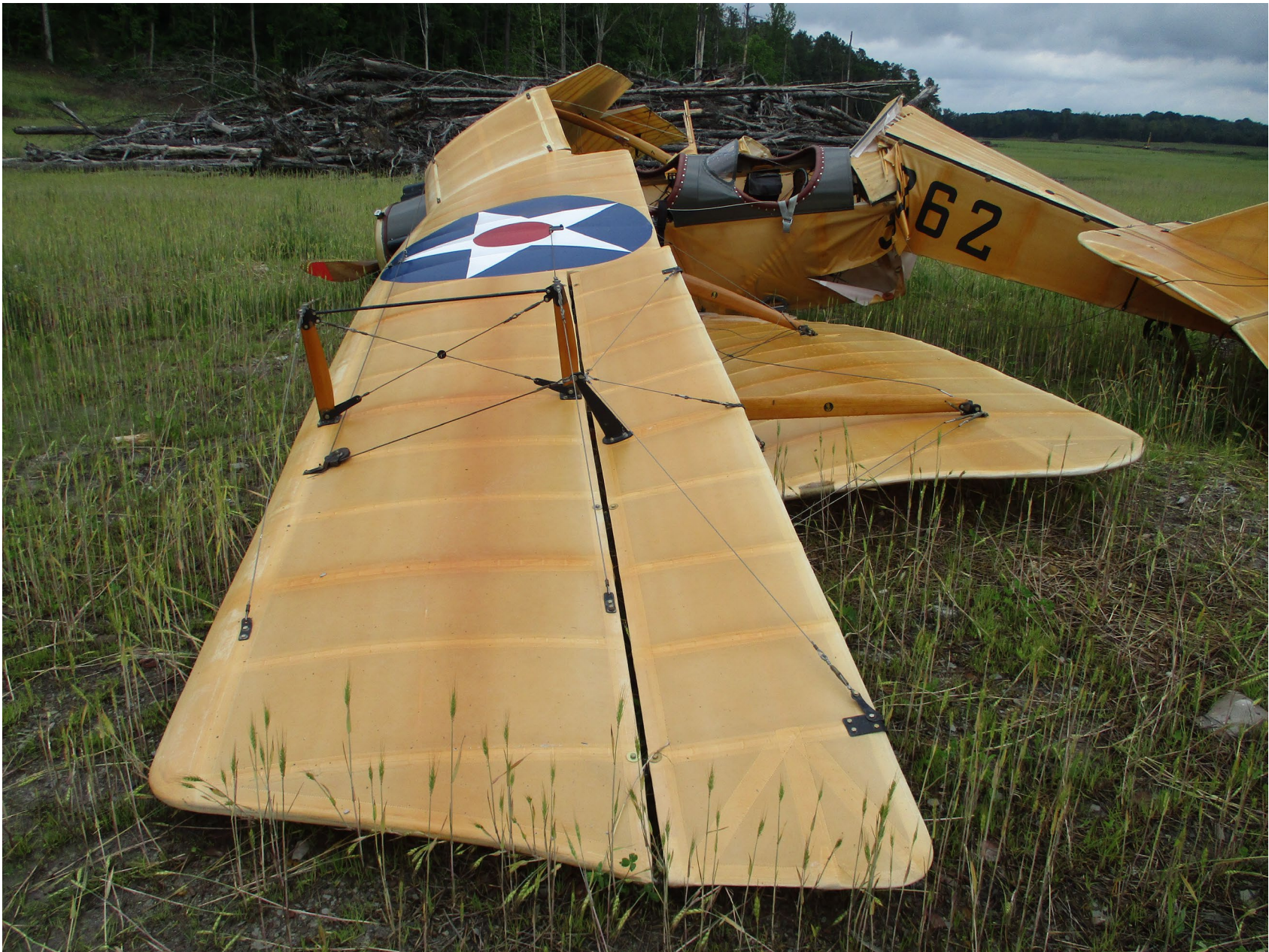
Photo 1 – FAA Digital Photograph. Left Side View of the Airplane at the Accident Site. Note the displaced Aft Empennage, and Upper and Lower Left Wings.
